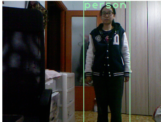
Figure 5.10: YOLO3: full body detection with a confidence value of 98%
