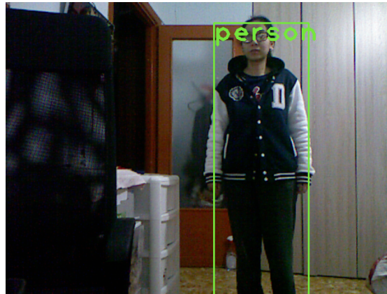
Figure 5.12: YOLO3-tiny: full body detection with a confidence value of 67%
