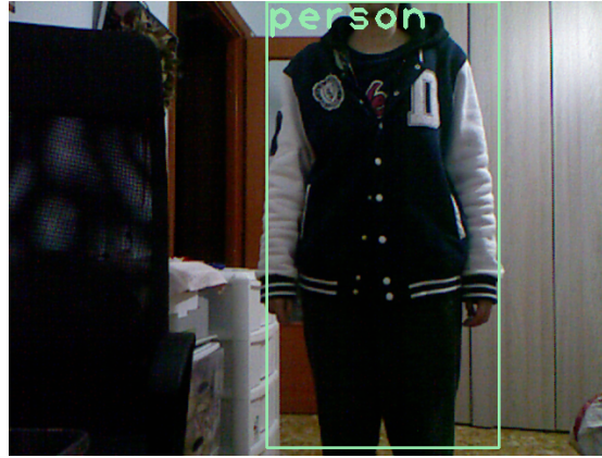
Figure 5.11: YOLO3: partial body detection with a confidence value of 96%
