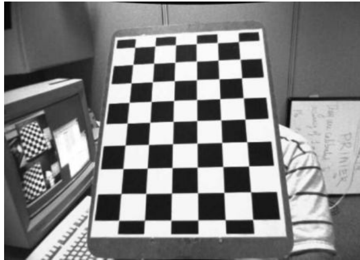
Figure 5.14: Checkerboard for camera calibration [43]
