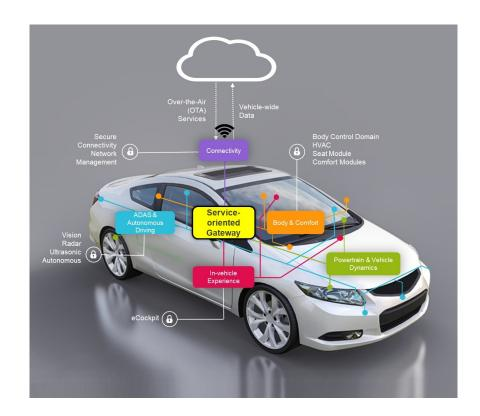
Figure 3.2: Vehicle domains and connectivity
