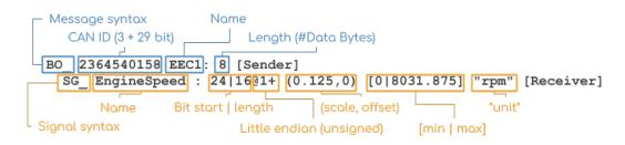
**Figure 4.7:** CAN DBC file with the explanation of the fields, from Csselectronics[14]
