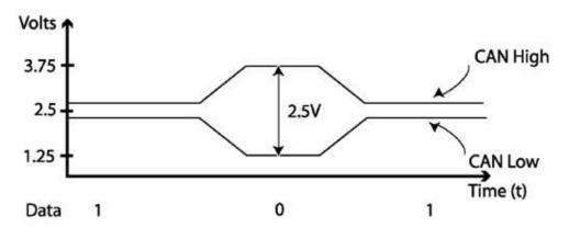
Figure 4.5: CAN voltage
