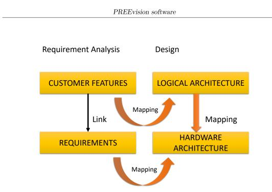
Figure 3.5: Relationship between customer features, requirements, logical architecture and hardware architecture mapping
