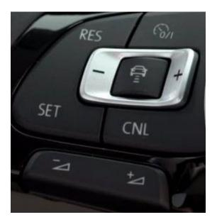
Figure 5.2: ACC controller in steering wheel
