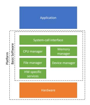
Figure 2.3: ECU division into standard components
