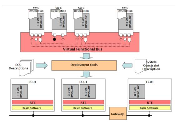
Figure 2.4: AUTOSAR components and their communication
