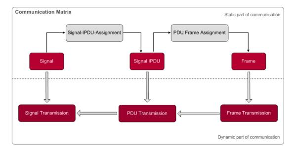
Figure 3.6: Signal, PDU and Frame relationship
