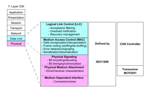
Figure 4.1: CAN and the OSI model
