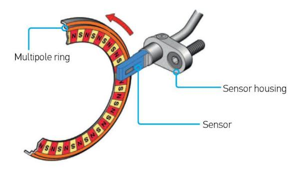
Figure 5.16: RPM sensor, from [15]
