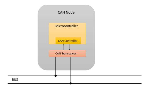
Figure 4.2: Can node components
