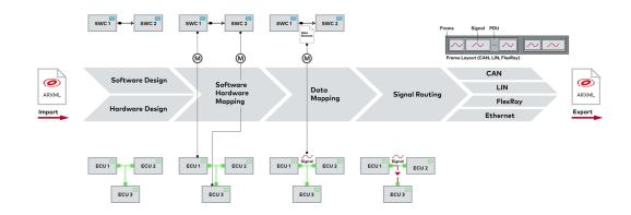
Figure 3.7: AUTOSAR system and software design process in PREEvision
