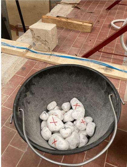
Figure 2.19: Debris Flow rocks used for the tests
