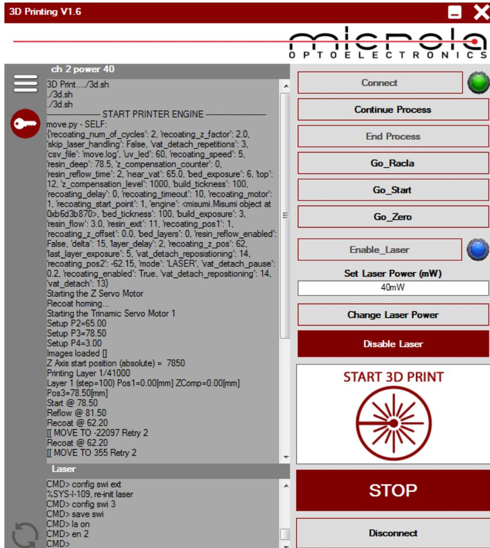
Figure 10 The software control panel of Microla printer.
