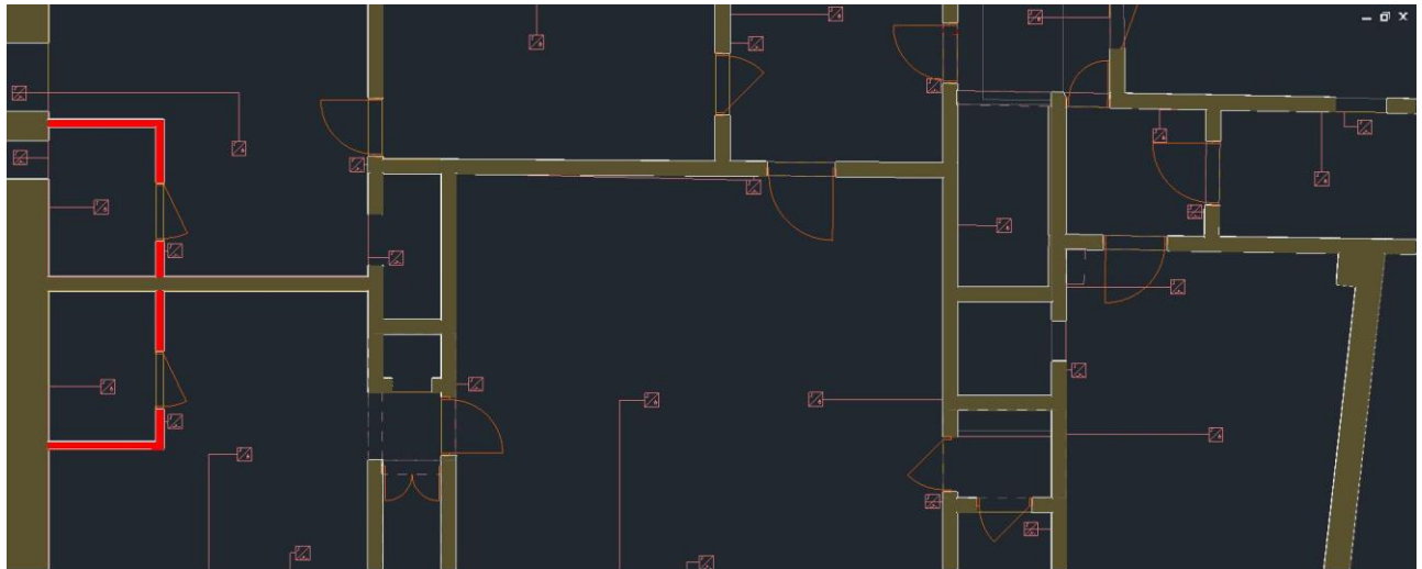
Figure 46 Binary entrances for smoke detectors, opening in the west area first floor
