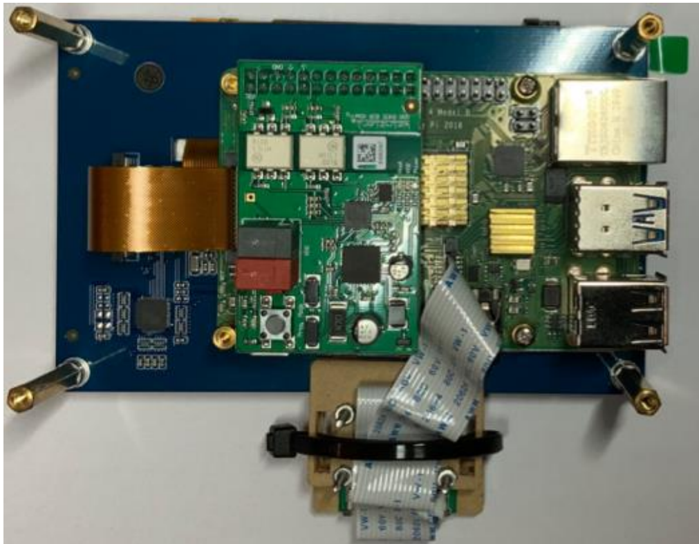
Figure 7 Device complete with a display, an 8Mp video camera and communication interface with the bus.
