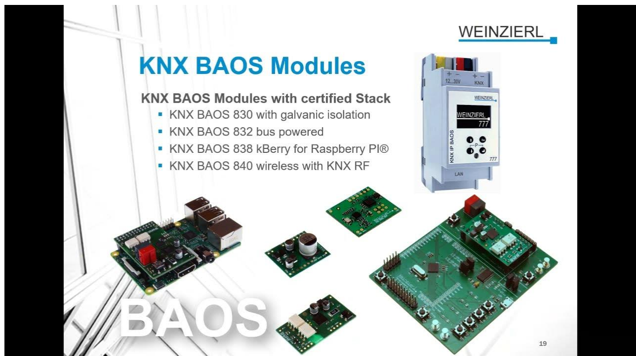
Figure 8 Weinzierl BAOS devices compatible with different media and used by many companies to develop products that can be interfaced with the KNX system.
