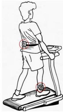
*Figure 1.18 Example of the experimental set-up of a subject walking on a treadmill walking machine equipped with accelerometers on the sacrum and the shank (Sabatini et al. 2015).*
