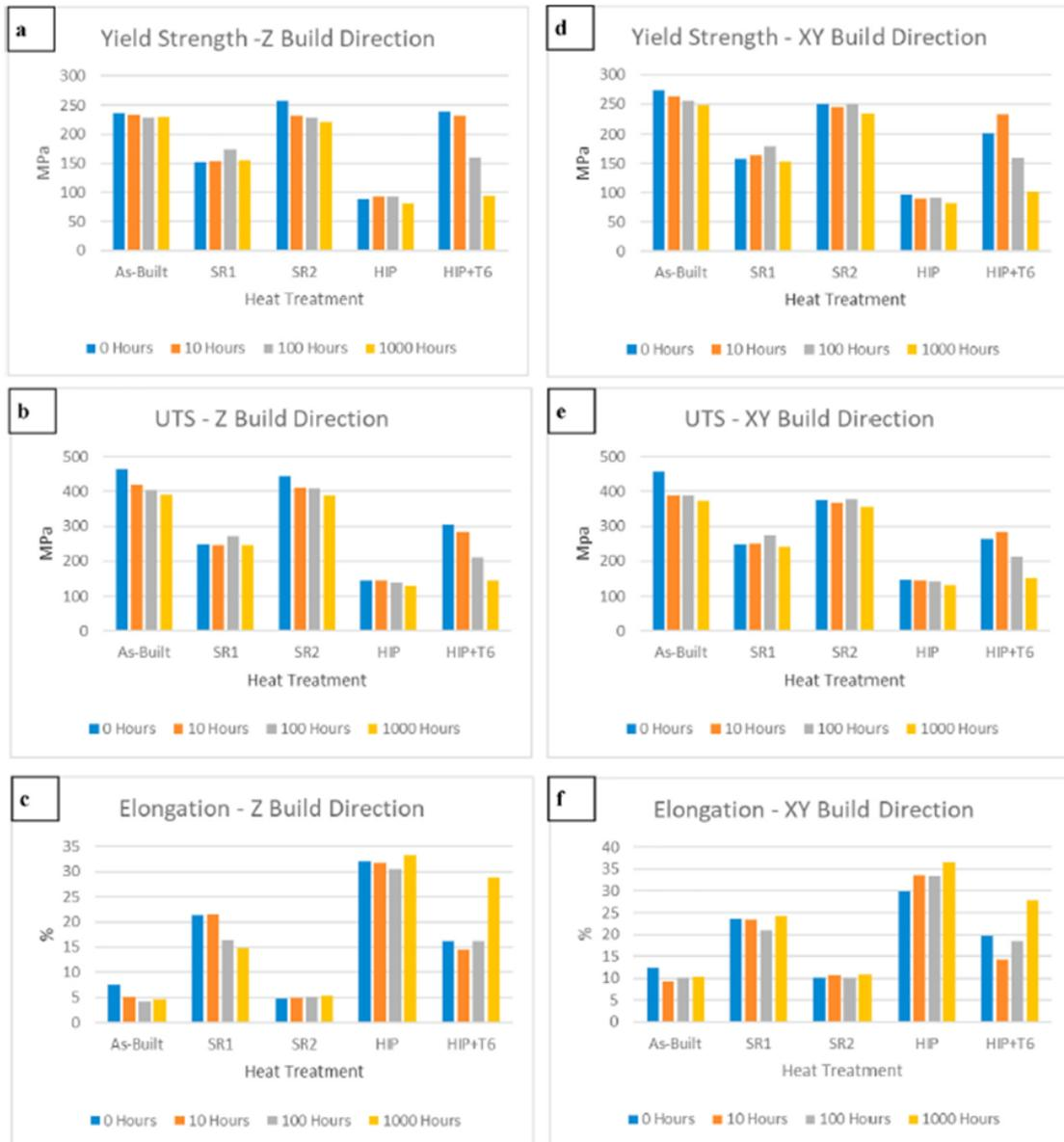
Figure 99: Effect of heat treatments (Table 10) on properties of AlSi10Mg SLMed samples for different aging times at 177 °C along Z and XY directions: (a) and (d) YS; (b) and (e) UTS; (c) and (f) elongation (from [137]).
