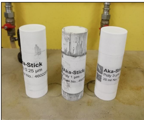
Fig.4.7 Diamond pastes (different size)
