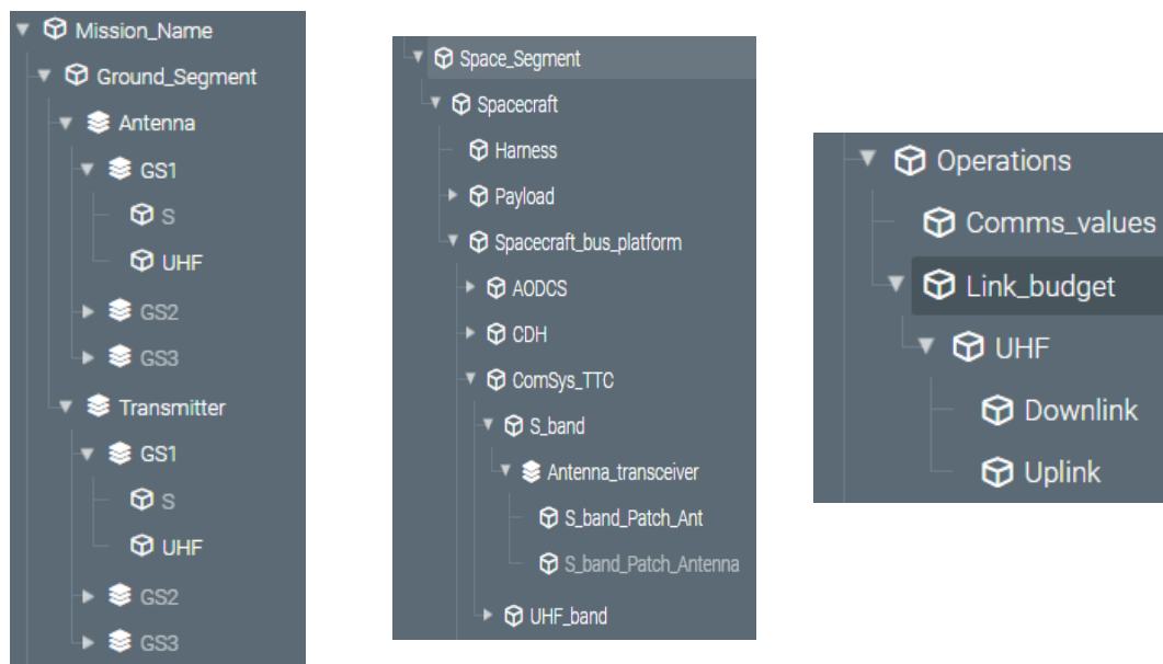
Figure 60: Example of Valispace architecture for the ground segment (left), space segment (centre), operations (right)
