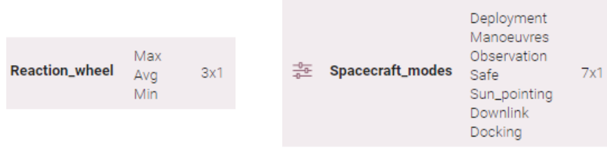
Figure 48: Mode example for components (left) and mission phases (right)
