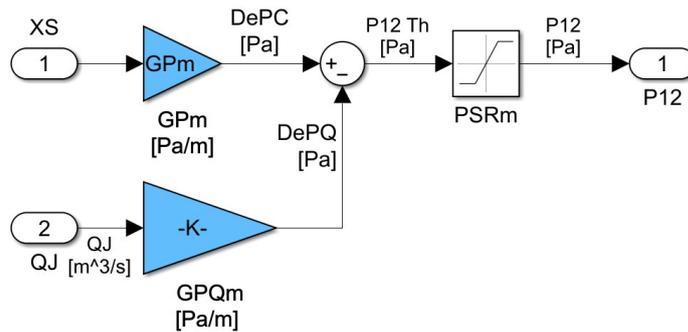
Figure 3.18: Model of the first stage of the valve in the simplified model
