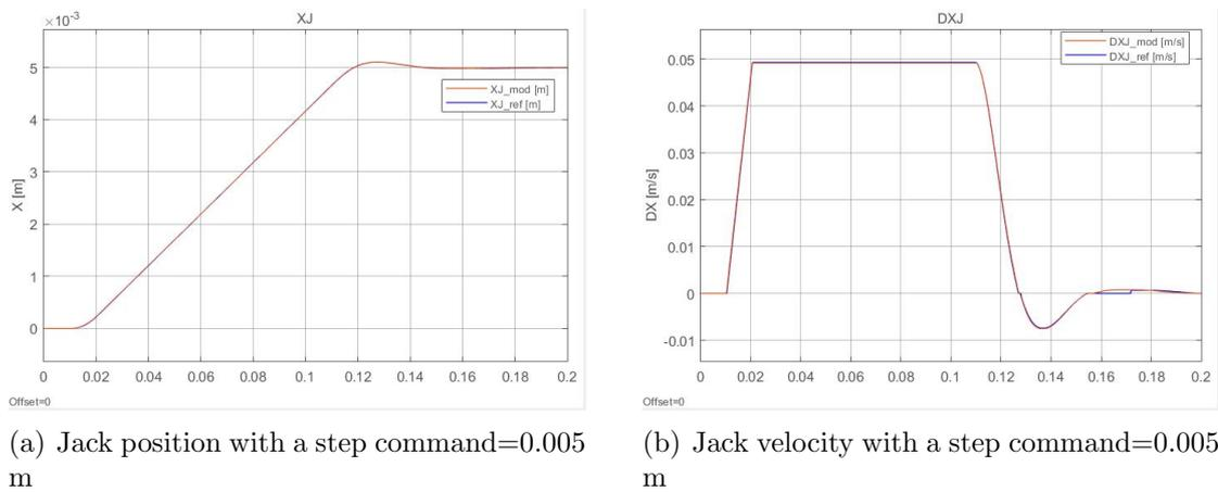
Figure 5.29: Position and velocity of the jack with no pipes implemented
