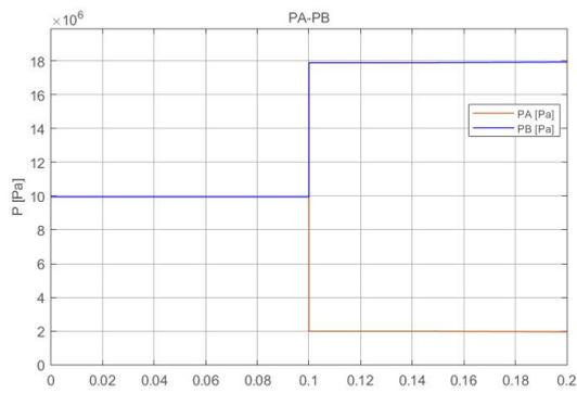
(a) Pressure in the chambers of the cylinder with a ramp command=0.5 m/s
