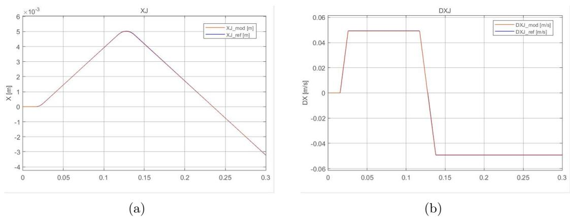
Figure 6.15: Position and Velocity of the jack with simultaneous commands
