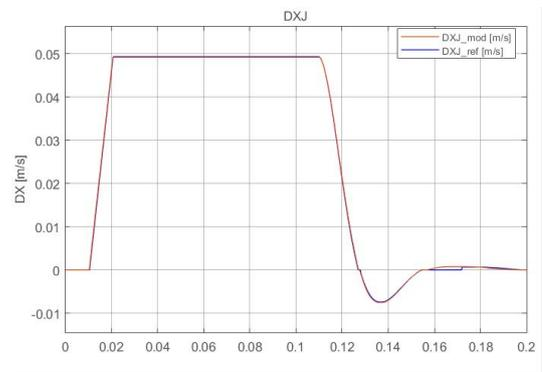
(b) Jack velocity with a step command= $0.005$  m
