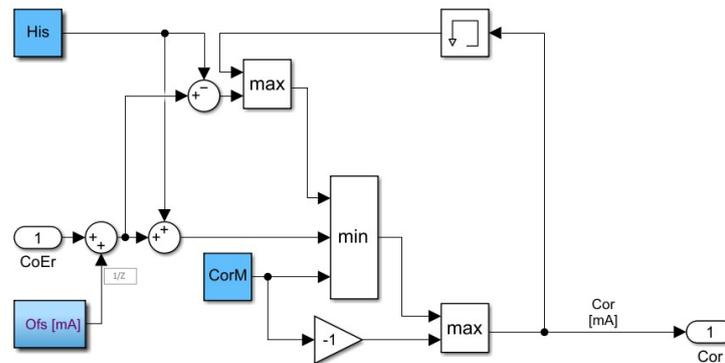
Figure 3.6: Torque motor Hysteresis block
