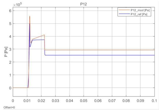
(d) [Pressure Difference in the actuator with a ramp command=0.1 m/s
