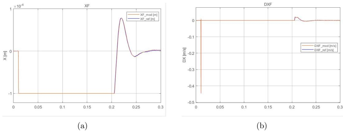
Figure 6.2: Position and Velocity of the flapper with a step command
