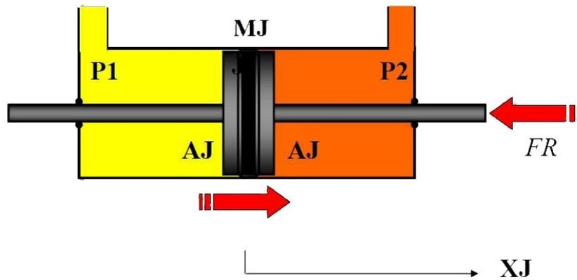
Figure 4.6: Scheme of a double-acting cylinder
