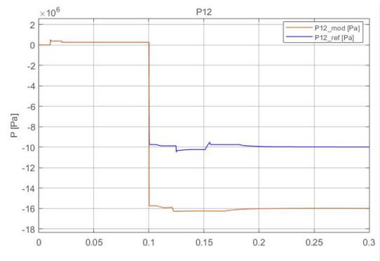
(b) Pressure Difference in the actuator with a step command=0.005 m
