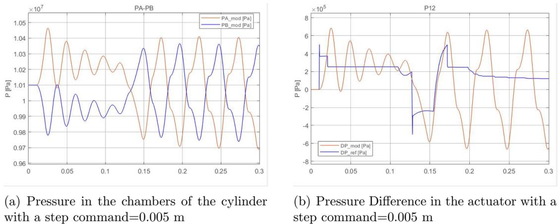
Figure 5.18: Pressure and difference pressure in the chambers of the actuator with a step commands and with the **Double-acting Cylinder - Translational friction** combination
