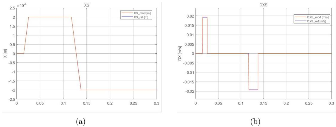
Figure 6.13: Position and Velocity of the spool with simultaneous commands
