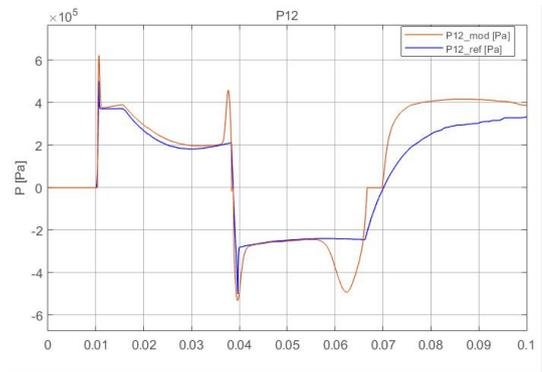
(f) [Pressure Difference in the actuator with a step command=0.0005m
