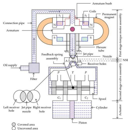
Figure 2.2: Scheme of Jet Pipe Valve
