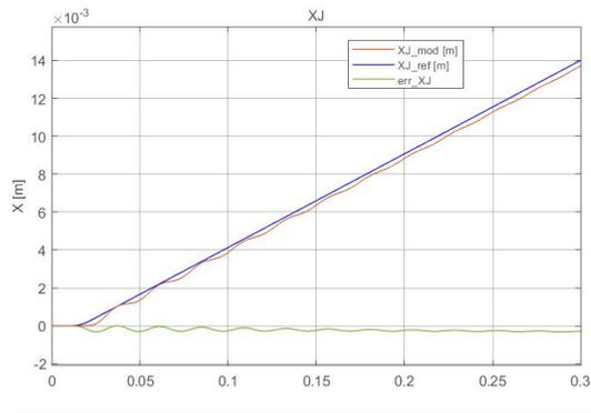
(a) Jack position with a ramp command=0.5 m/s
