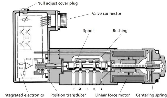
Figure 2.1: Scheme of Direct Drive Valve
