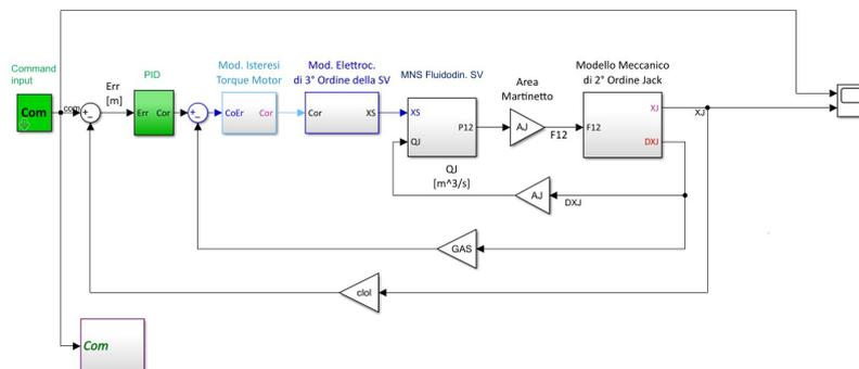
Figure 3.2: Light up of Command Subsystem in the Simulink model
