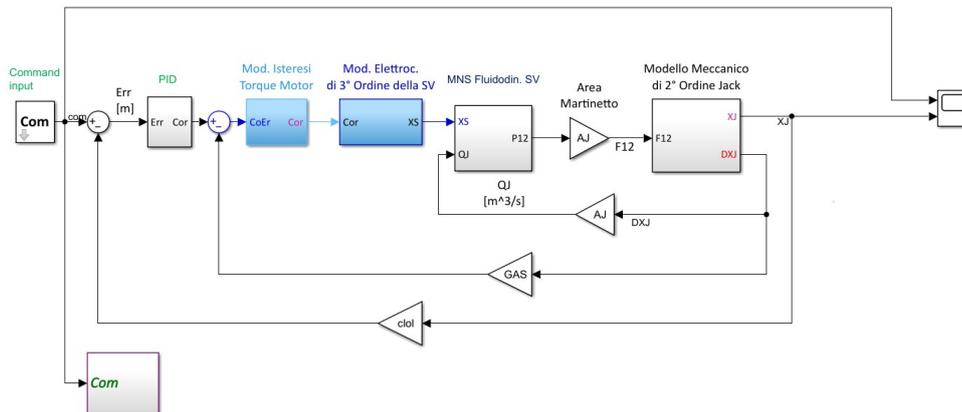
Figure 3.5: Light up of the First Stage in the Simulink model
