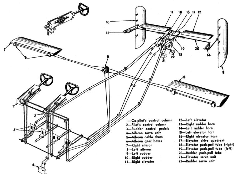
Figure 1.2: A scheme of mechanical control system
