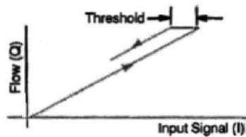
Figure 2.9: Effect of a threshold
