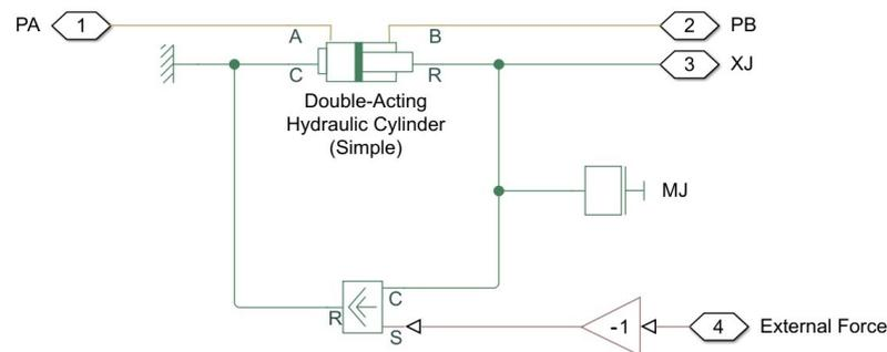
Figure 4.10: SimScape model of the actuator with the Double-Acting cylinder (simple) block
