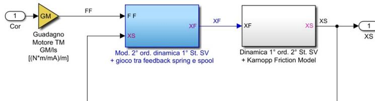
Figure 3.7: Electromechanical model blocks with light up of the first stage block
