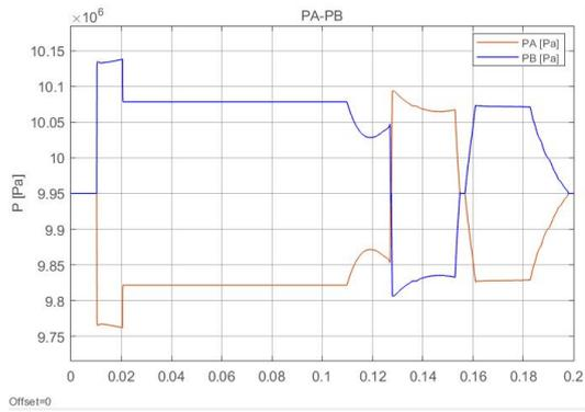
(a) Pressure in the chambers of the cylinder with a step command=0.005m
