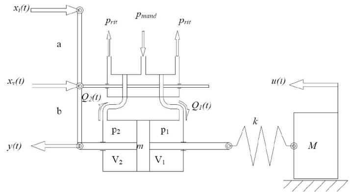
Figure 1.3: Scheme of an Hydromechanical actuator (HMA)
