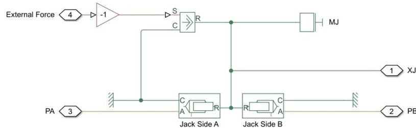
Figure 4.9: SimScape model of the actuator with two Translational Hydro-Mechanical converter
