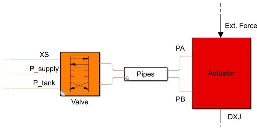
Figure 4.16: Connection between Valve and Actuator with the Pipe block
