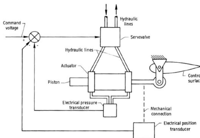
Figure 1.5: A scheme of an Electrohydraulic actuator
