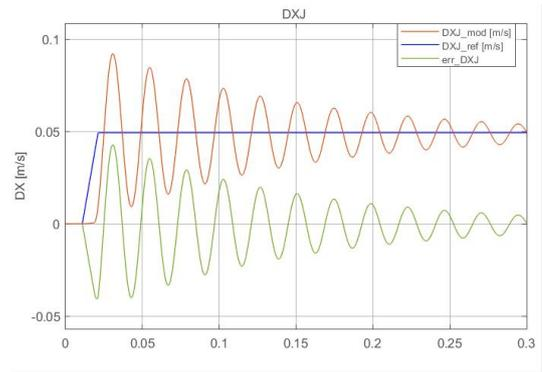
(b) Jack velocity with a ramp command=0.5 m/s
