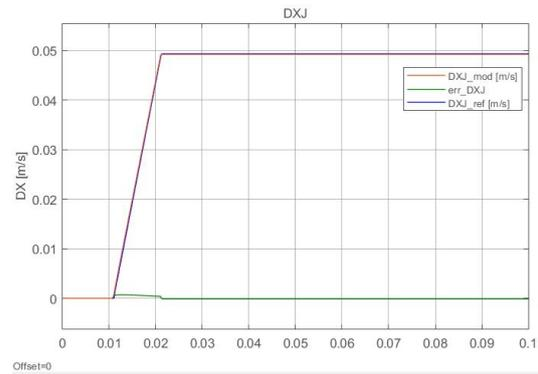
(b) Jack velocity with a ramp command=0.5 m/s
