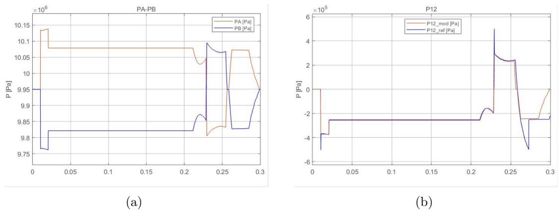
Figure 6.4: Pressures and Difference pressure with a step command
