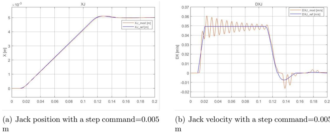
Figure 5.27: Position and velocity of the jack with the compressibility ON
