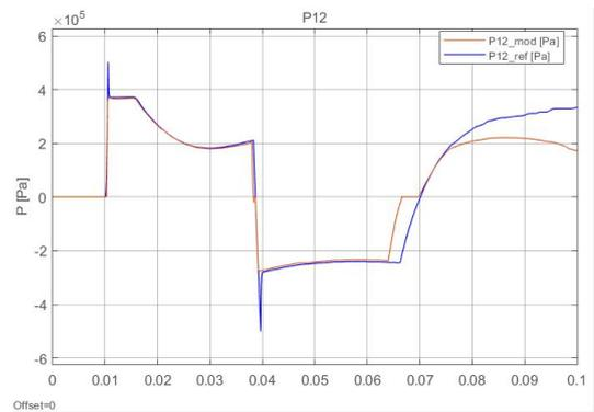
(f) [Pressure Difference in the actuator with a step command=0.0005m
