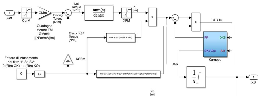
Figure 3.17: Model of the first stage of the valve in the simplified model
