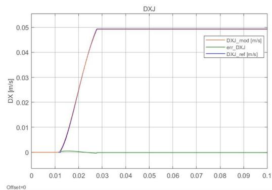
(f) Jack velocity with a ramp command=0.05 m/s
