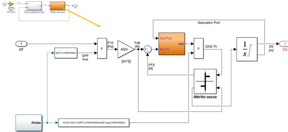
Figure 3.9: Model of the second stage of the servovalve
