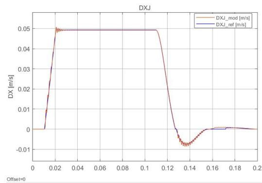
(b) Jack velocity with a step command=0.005 m
