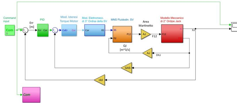
Figure 3.1: Reference Simulink model of electro-hydraulic servovalve
