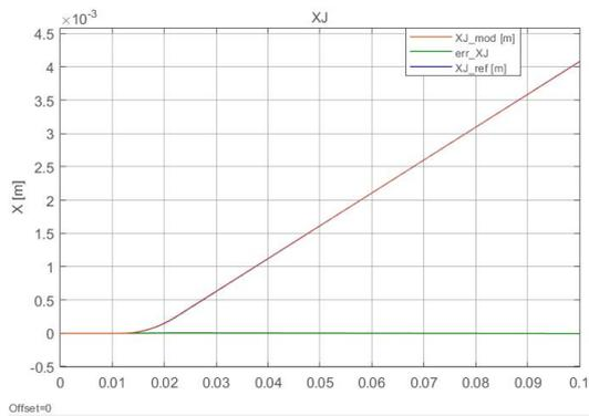
(c) Jack position with a ramp command=0.1 m/s
