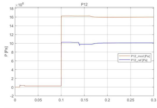
(b) Pressure Difference in the actuator with a step command=0.005 m
