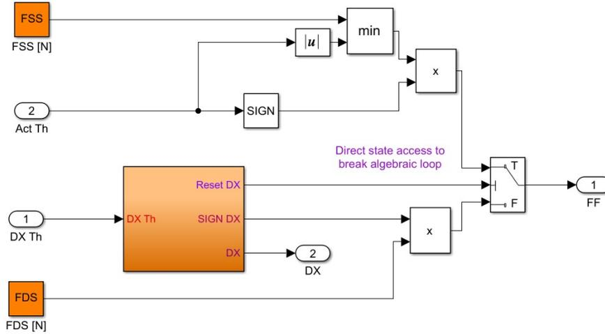
Figure 3.10: Borello's friction model
