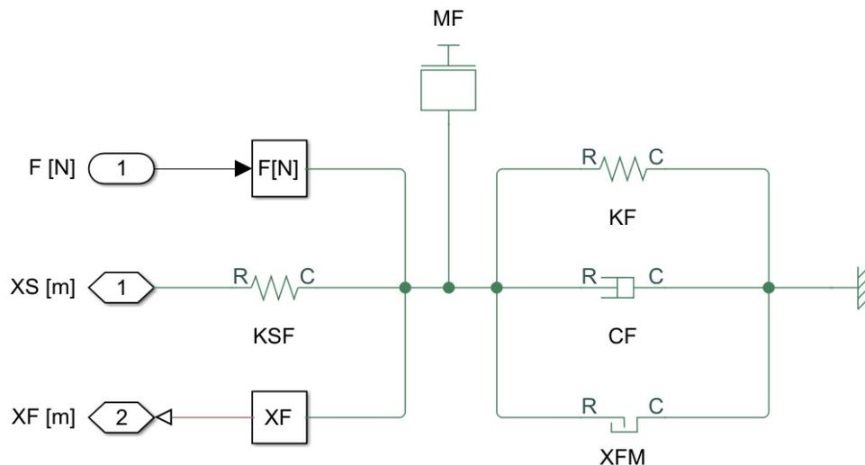
Figure 4.3: SimScape model of the flapper
