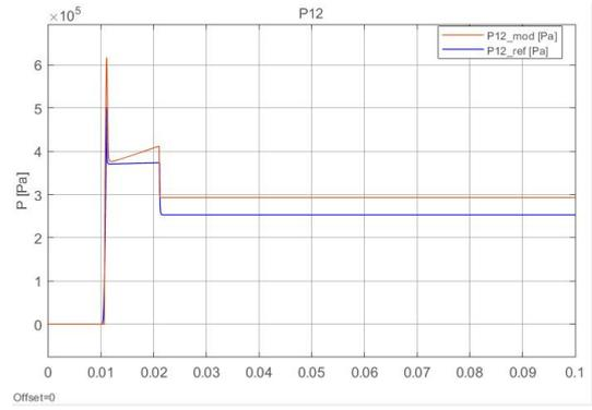
(b) Pressure Difference in the actuator with a ramp command=0.5 m/s
