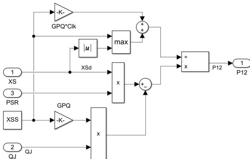
Figure 3.12: Fluid dynamic model in the second block
