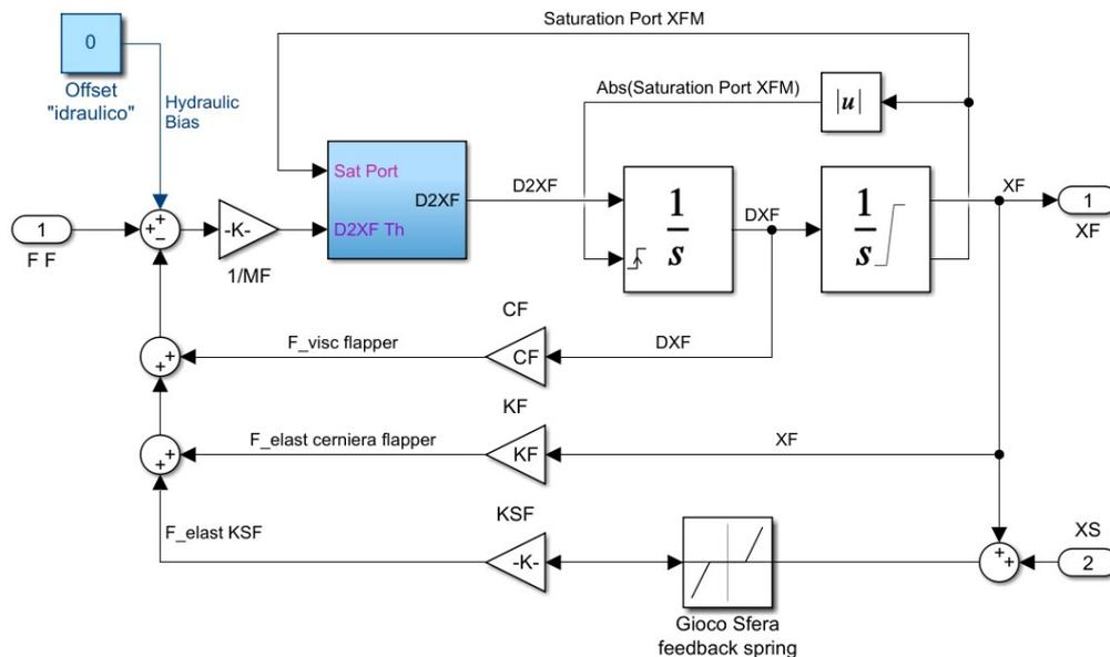
Figure 3.8: Model of flapper dynamics
