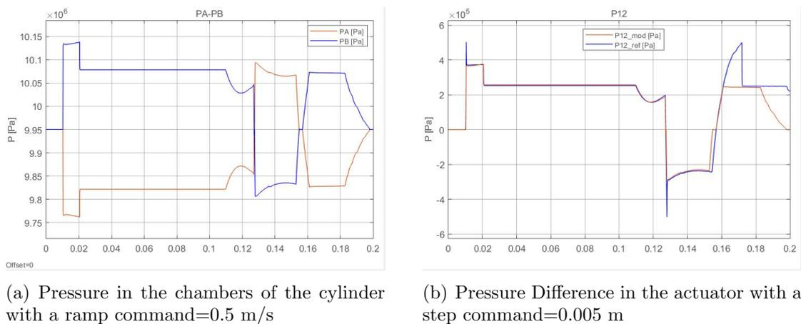
Figure 5.30: Pressure and difference pressure in the chambers of the actuator with no pipes implemented
