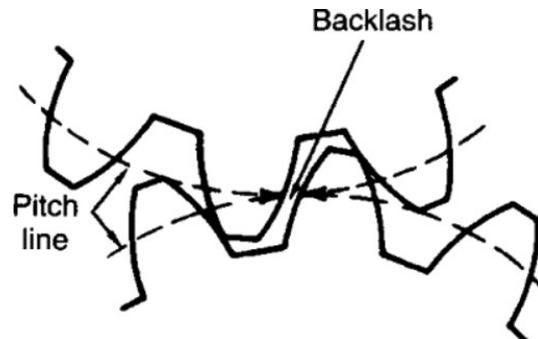
Figure 2.11: Backlash in a gear connection
