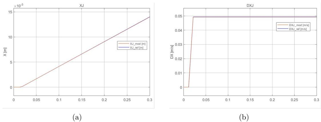
Figure 6.10: Position and Velocity of the jack with a ramp command
