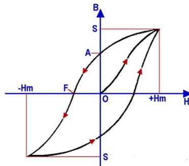
Figure 2.8: Typical magnetization curve
