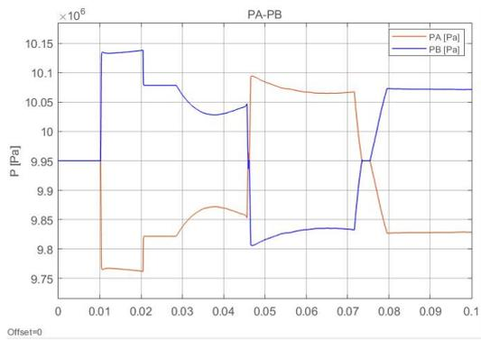
(c) Pressure in the chambers of the cylinder with a step command=0.001m
