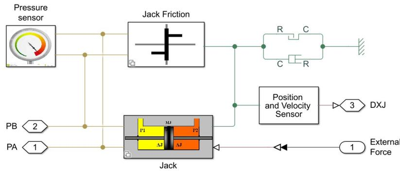
Figure 4.7: Overview of the SimScape model of the actuator
