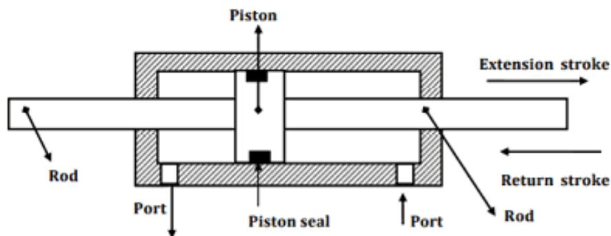
Figure 3.14: Double-acting cylinder with the piston-rod
