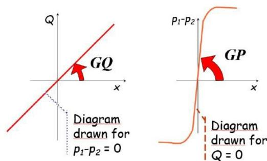
Figure 2.7: Gains of the servovalve
