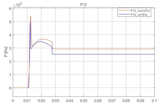
(f) [Pressure Difference in the actuator with a ramp command=0.05 m/s
