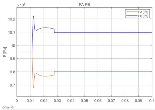
(e) Pressure in the chambers of the cylinder with a ramp command=0.05 m/s
