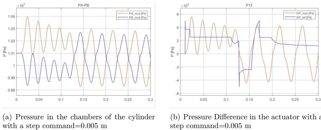
Figure 5.22: Pressure and difference pressure in the chambers of the actuator with a step commands and with the **Double-acting Cylinder - Cylinder friction** combination
