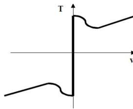
Figure 2.13: Striebeck's curve
