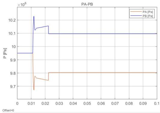
(c) Pressure in the chambers of the cylinder with a ramp command=0.1 m/s
