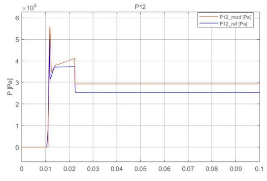
(d) [Pressure Difference in the actuator with a ramp command=0.1 m/s
