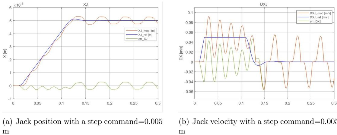
Figure 5.21: Position and Velocity of the actuator with a step commands
