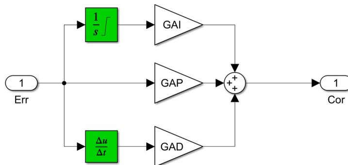
Figure 3.4: Controller PID
