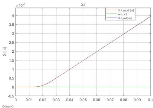
(e) Jack position with a ramp command=0.05 m/s
