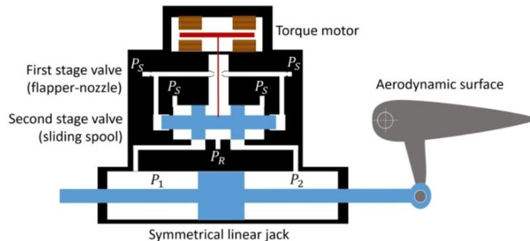
Figure 2.5: Flapper-nozzle valve with the Jack and the surface control
