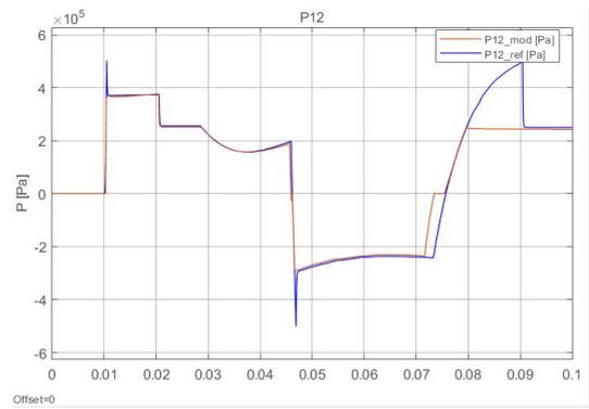
(d) [Pressure Difference in the actuator with a step command=0.001m
