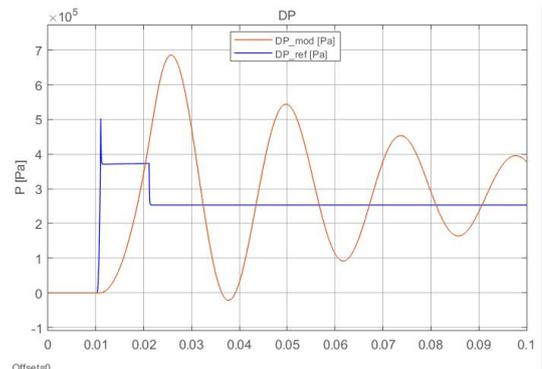
(b) Pressure Difference in the actuator with a ramp command=0.5 m/s
