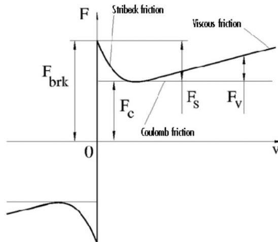
Figure 4.14: Friction Model in SimScape friction blocks
