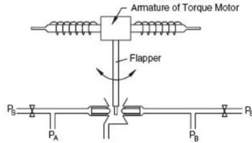
Figure 2.4: Detail of the first stage of Flapper-nozzle valve
