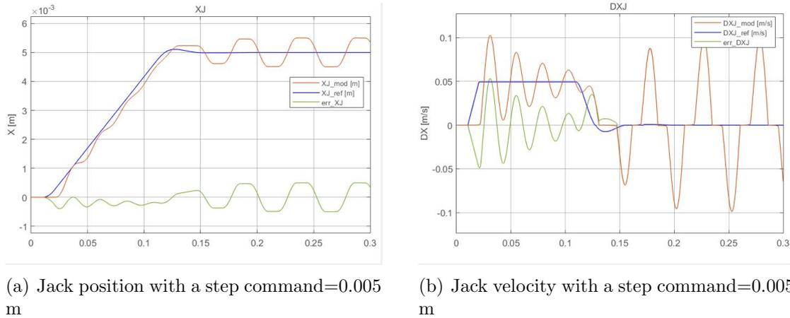
Figure 5.17: Position and Velocity of the actuator with a step commands
