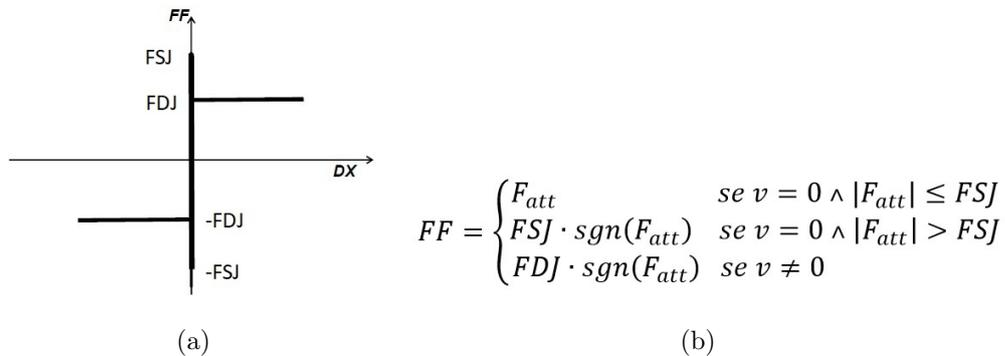
Figure 2.12: Model and equation of Coulomb's friction model
