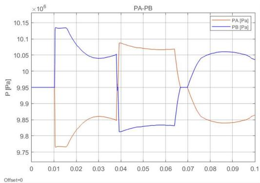
(e) Pressure in the chambers of the cylinder with a step command=0.0005m
