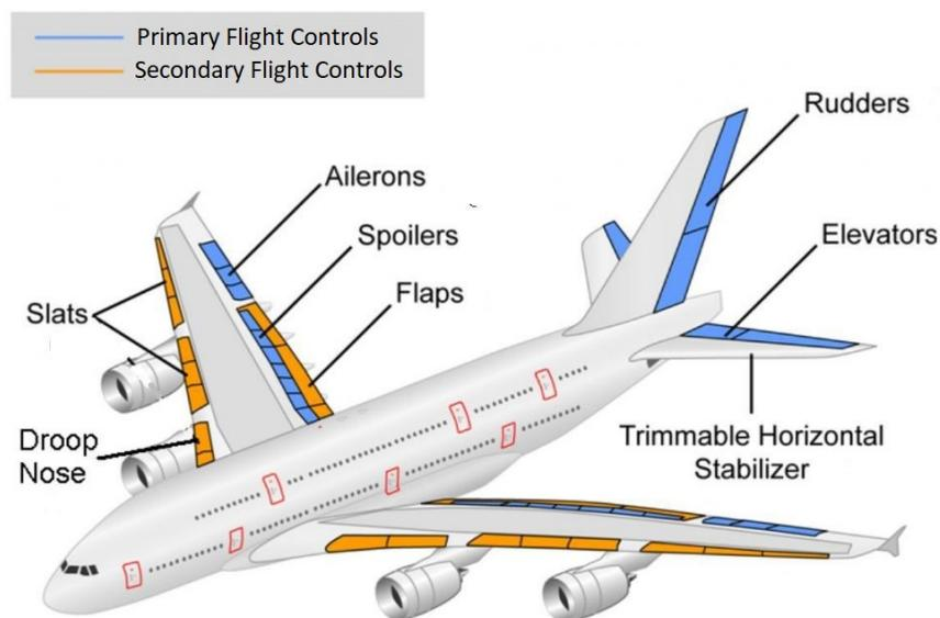
Figure 1.1: All of the control surfaces on a fixed-wing aircraft
