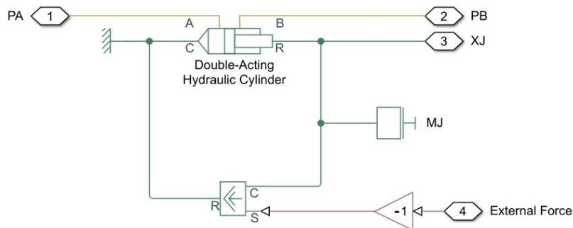
Figure 4.11: SimScape model of the actuator with the Double-Acting cylinder block
