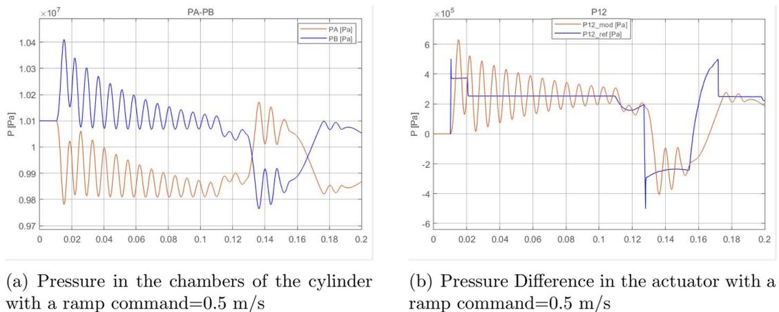
Figure 5.28: Pressure and difference pressure in the chambers of the actuator with the compressibility ON
