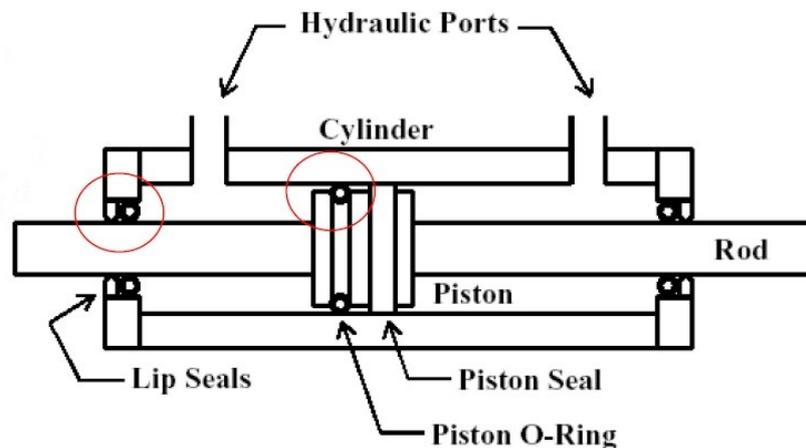
Figure 4.12: Details of where the friction could occur in a Double-Acting Cylinder
