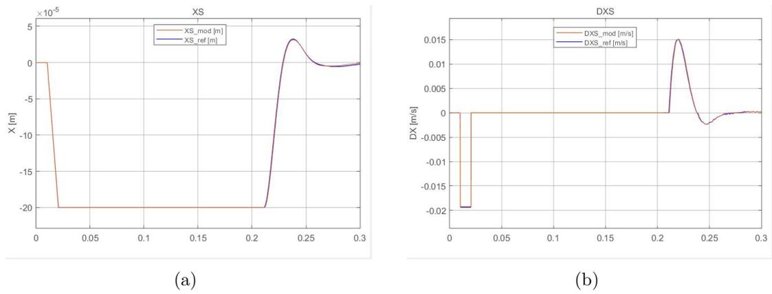
Figure 6.3: Position and Velocity of the spool with a step command
