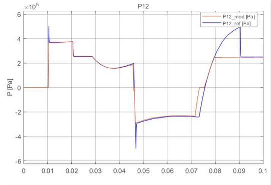
(d) [Pressure Difference in the actuator with a step command=0.001m
