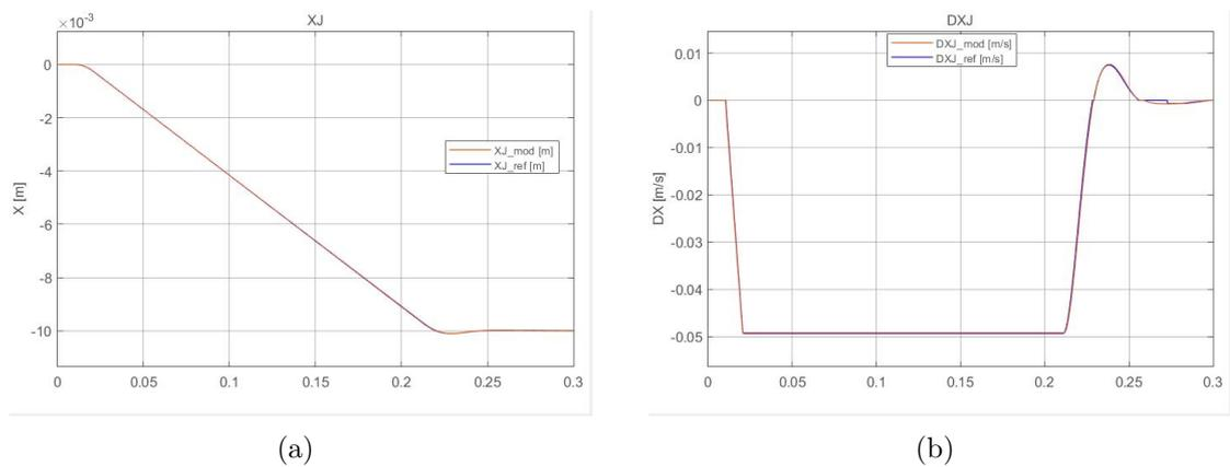
Figure 6.5: Position and Velocity of the jack with a step command
