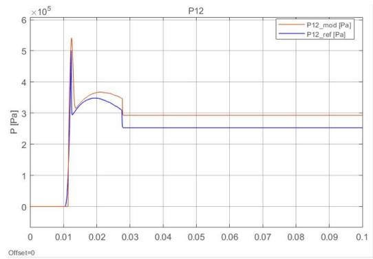
(f) [Pressure Difference in the actuator with a ramp command=0.05 m/s
