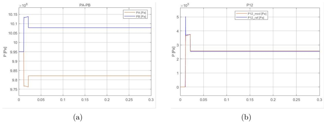
Figure 6.9: Pressures and Difference pressure with a ramp command
