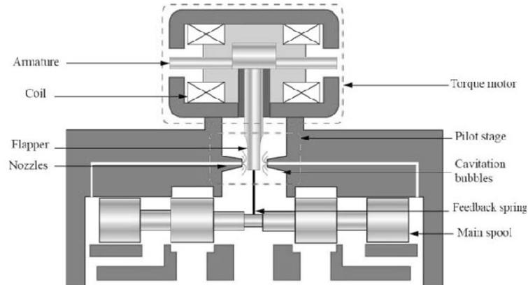
Figure 2.3: Scheme of Flapper-nozzle valve
