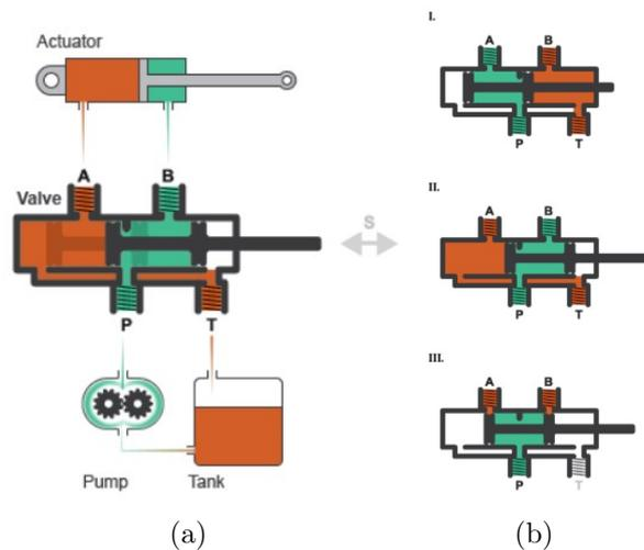
Figure 4.8: General setup of a valve and different position of the spool
