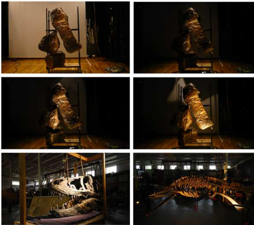
Testing lights on the studio mock-up (1 to 4 pictures) and on the real one(5 to 6 pictures). Starting from the left corner the dinosaurs are lit as: downlight with metal halide lamp and generic ambient light; accent-light with spot LED light; accent-light with two spots LED lights; accent-light with metal halide spot lamp. In the two last pictures the same test was made on the real dinosaur mockup in Los Angeles
