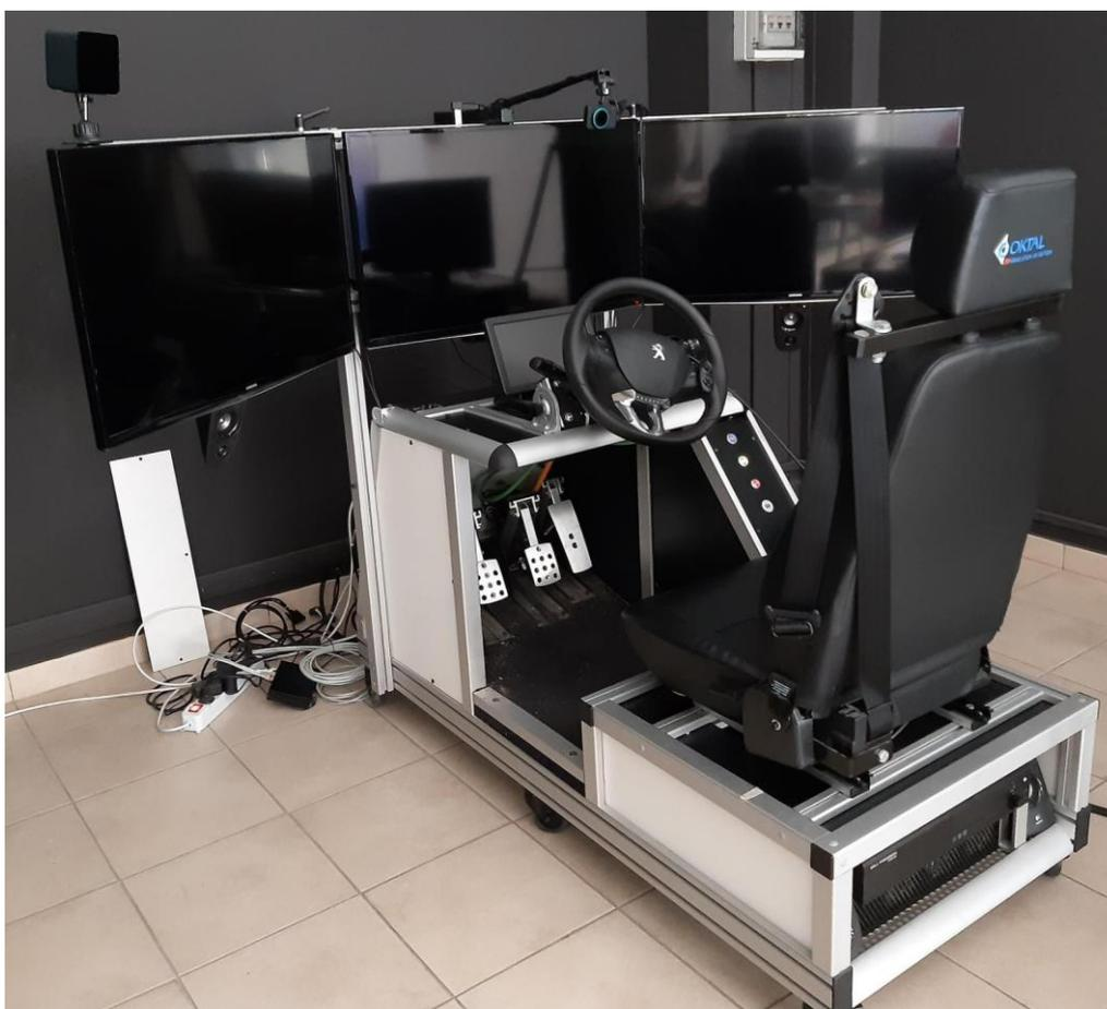
*Figure 15. Fixed-base driving simulator at RSDS laboratory (DIATI, Politecnico di Torino).*
