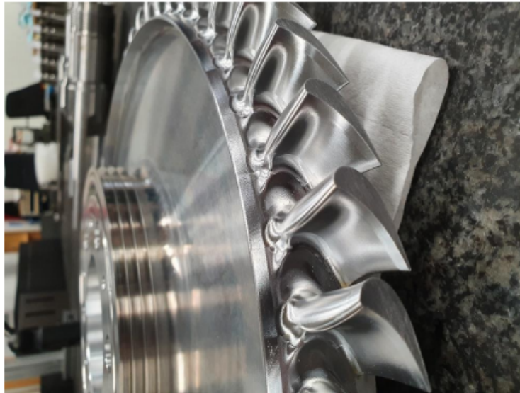
Figure 5.2: Rotor blisk of test object No 6
