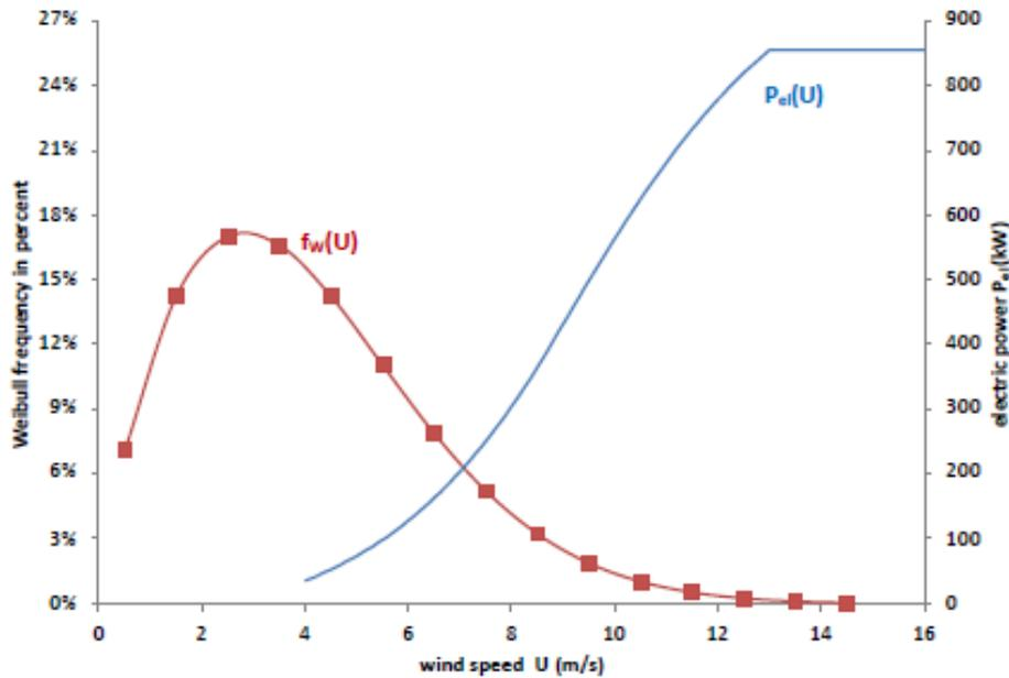
Figure 1. 13 Power curve of WT and Weibull distribution [10]
