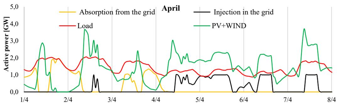
*Figure 4. 16 Maximization of self-sufficiency, monthly profiles with absorption and injection in the grid*
