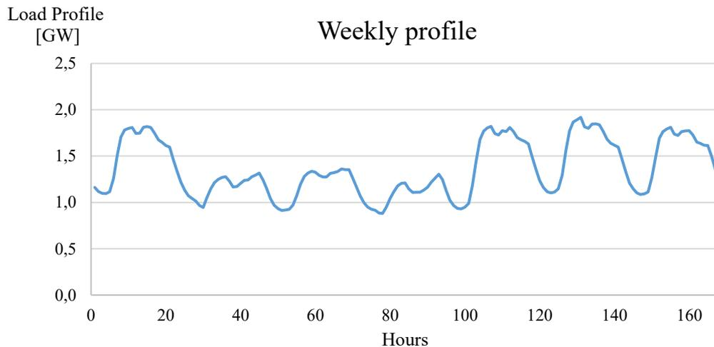
Figure 3. 10 Calculated weekly load profile
