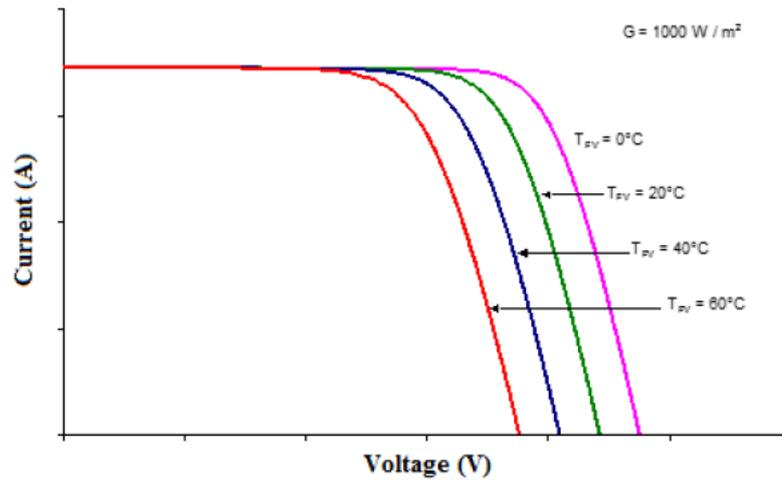
Figure 1. 8 Characteristic curves at different temperature [6]
