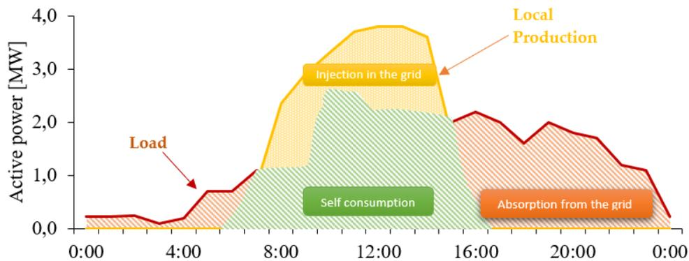
*Figure 1.2 Representative load and generation profiles*
