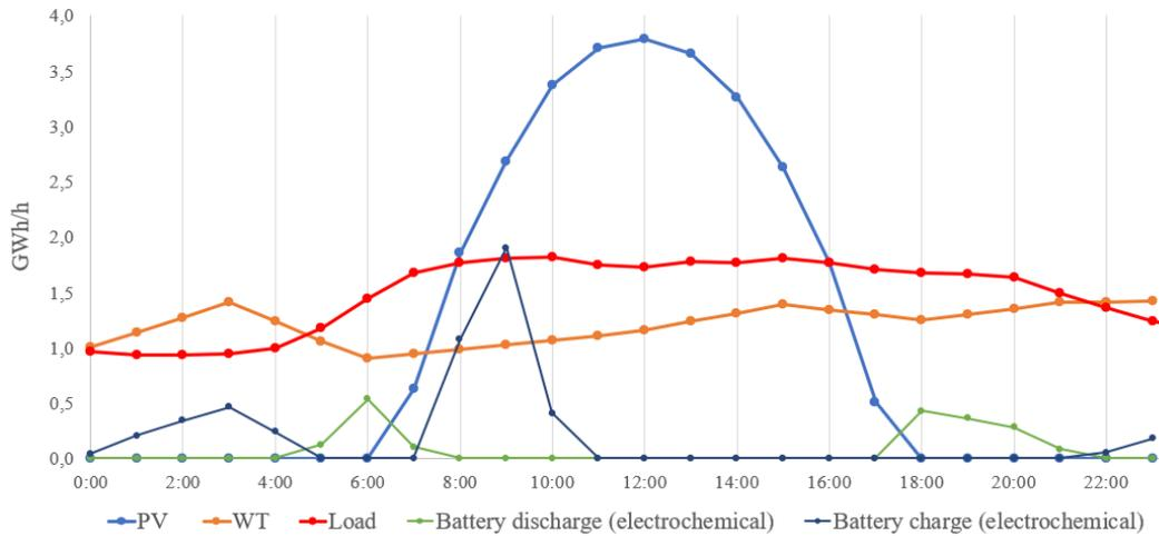
Figure 4. 10 Daily profiles with use of the storage battery for a clear day
