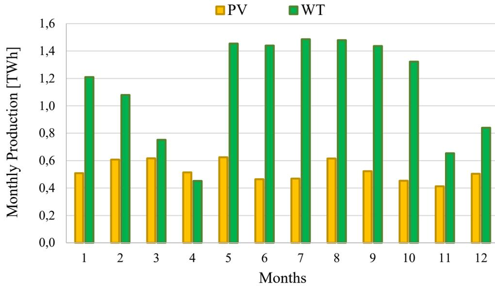
Figure 4. 17 Maximization of self-sufficiency, monthly production of the photovoltaic and wind power plant
