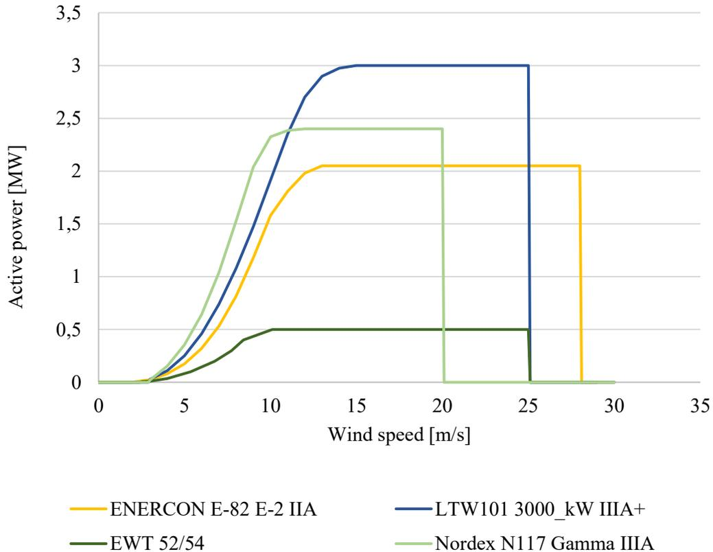
Figure 1.19 Power curve of four wind turbines
