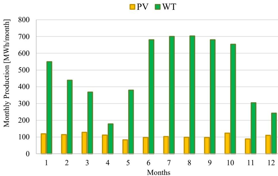
Figure 4. 6 Monthly production of the photovoltaic and wind power plant for Site #2
