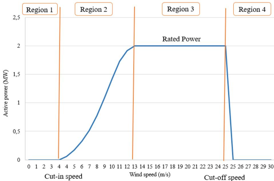
*Figure 1. 12 Power curve of wind turbine*
