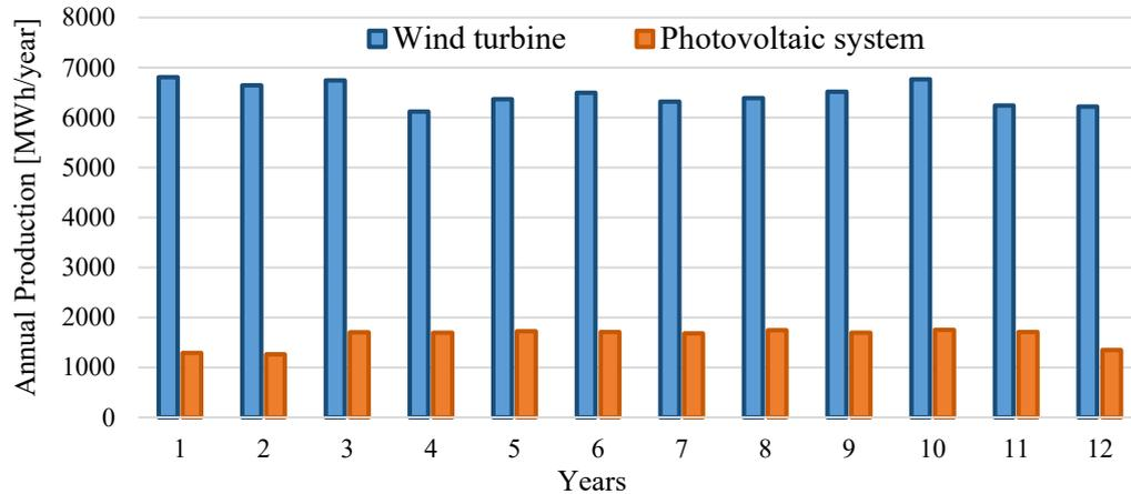
Figure 4. 7 Annual production of the wind and the photovoltaic system, Site #2
