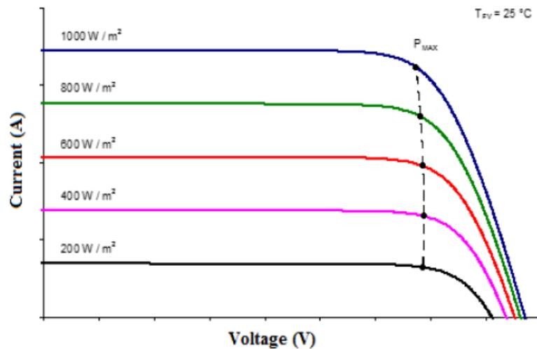
Figure 1. 7 Characteristic curves at different solar radiation [6]
