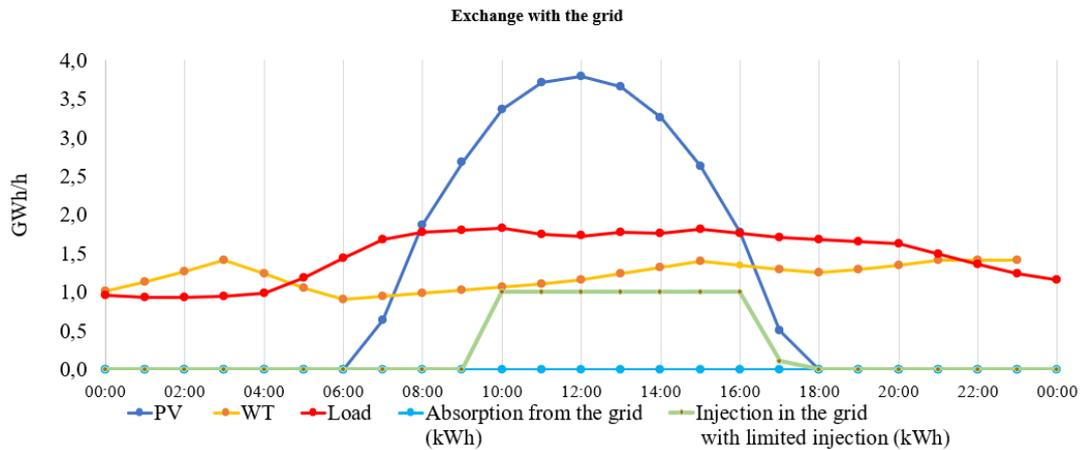
Figure 4. 11 Daily profiles with exchanges with the grid for a clear day
