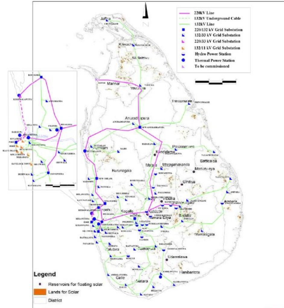
Figure 2. 15 Suitable sites for PV installations near to transmission grid
