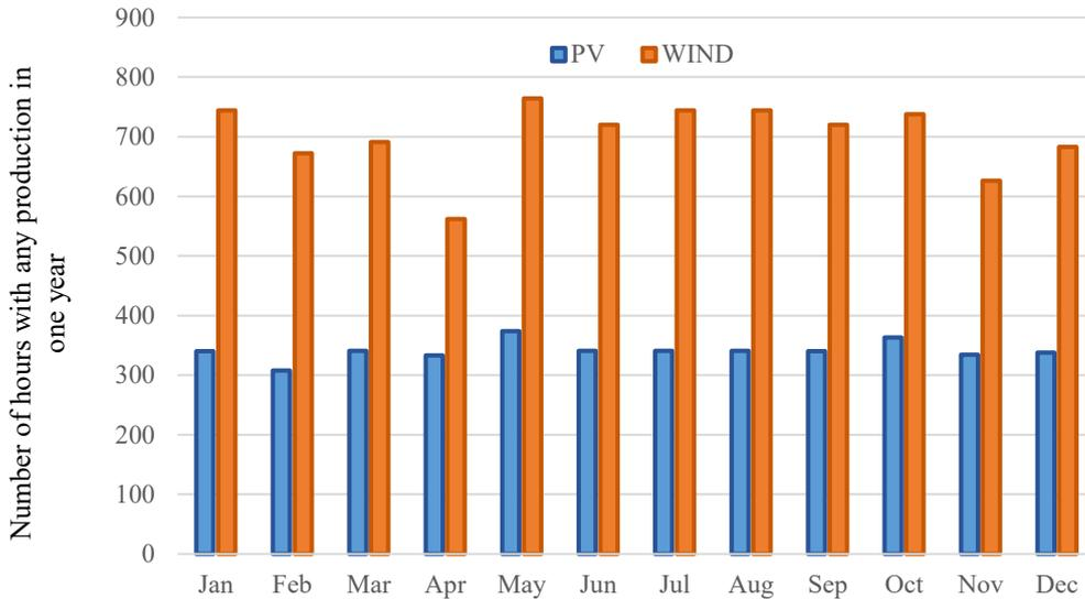
Figure 4. 1 Monthly resource hours of PV and wind systems for Site #2
