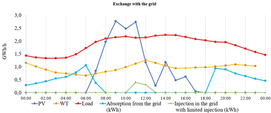
Figure 4. 14 Daily profiles with exchanges with the grid, for a day with low availability of the wind resource
