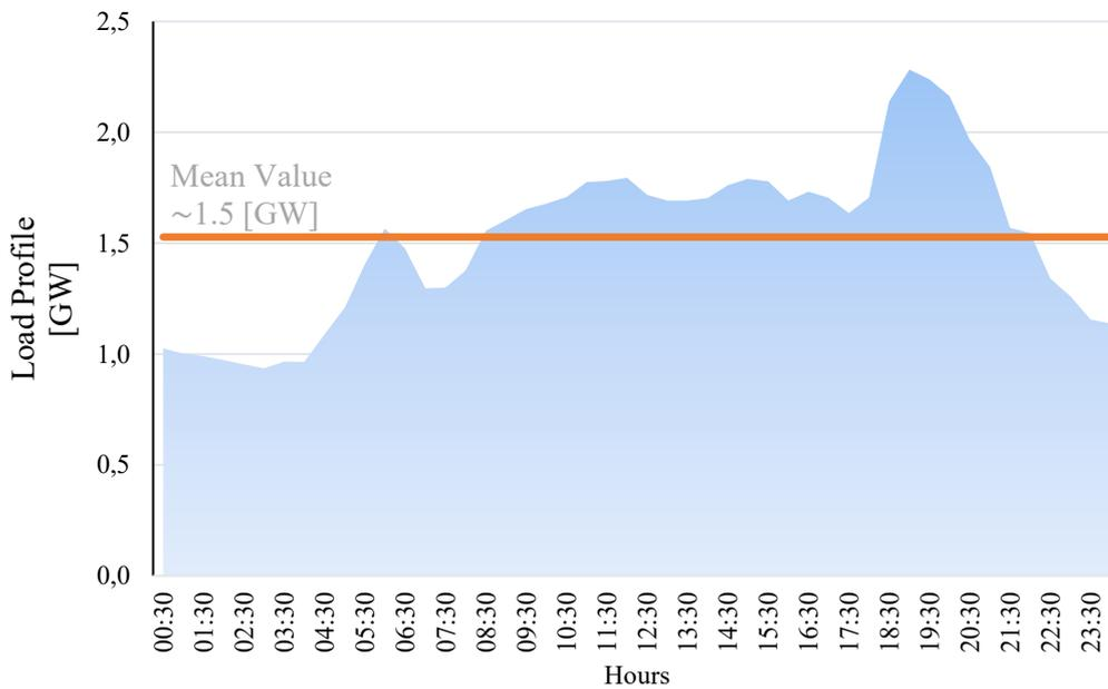
Figure 3. 8 Load Profile of 22/09/2015 in Sri Lanka [73]
