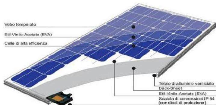
Figure 1. 9 Components of a photovoltaic module [5]
