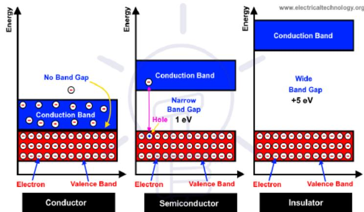
*Figure 1. 3* Diagram of the electronic band structure for conductors, semiconductors and insulator materials [5]
