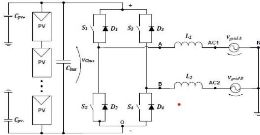
Figure 1. 10 Diagram of a full bridge inverter
