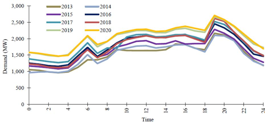
Figure 3. 9 Daily profile in Sri Lanka for different years [71]
