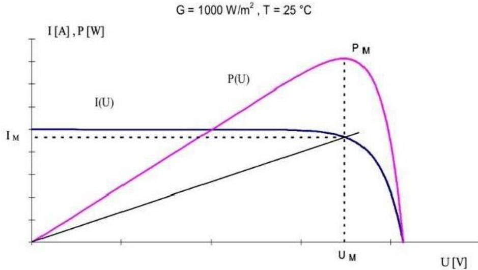
Figure 1.6 Characteristic curve of solar cell at standard test condition
