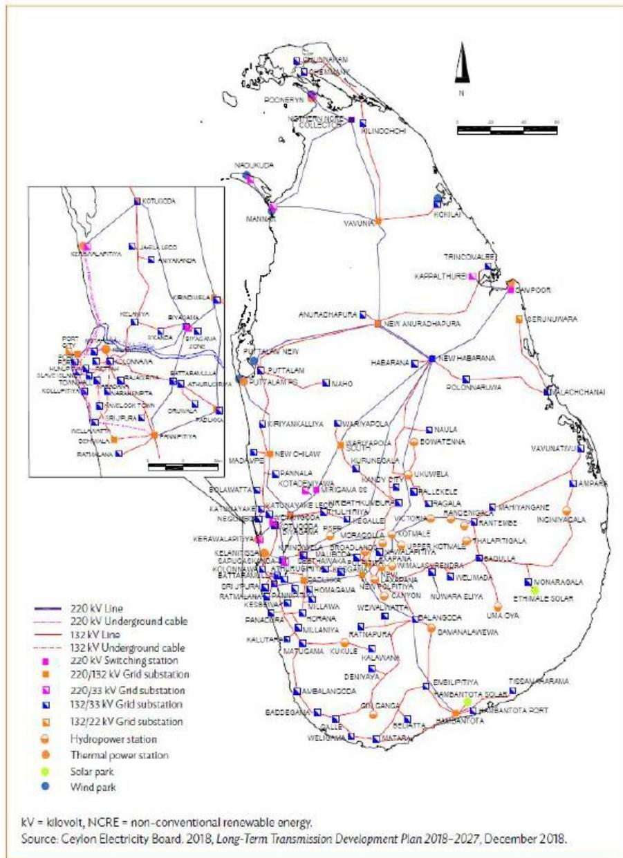
*Figure 2. 8 Transmission grid of Sri Lanka [23]*
