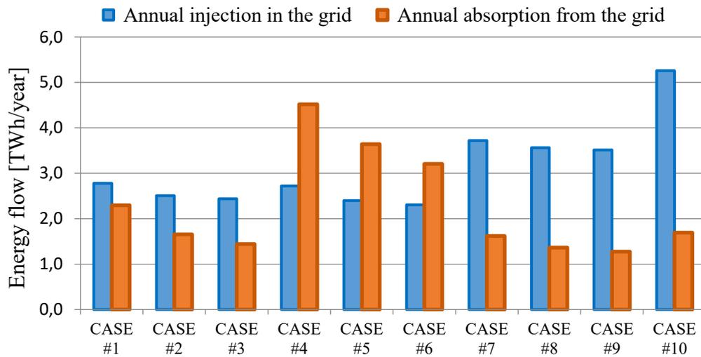
Figure 4. 24 Exchanges with the grid for 10 simulations. Part. 1
