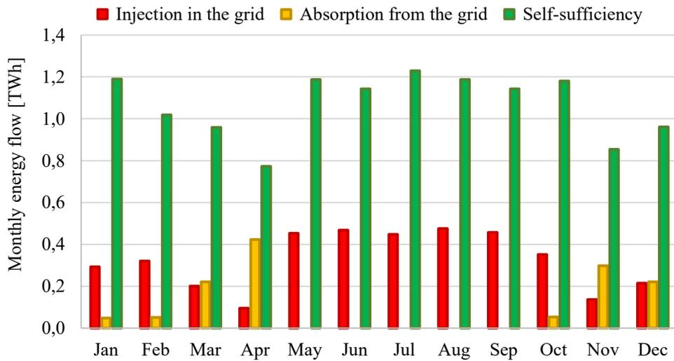
Figure 4. 18 Maximization of self-sufficiency, annual exchanges with the grid and monthly value of self-sufficiency energy
