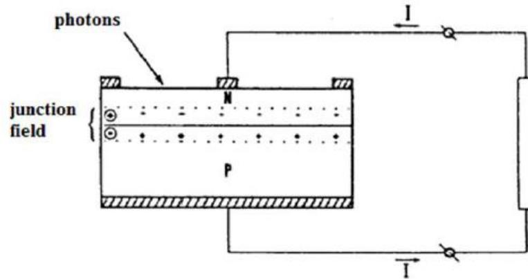
Figure 1. 4 Structure of polycrystalline Silicon solar cell [6]
