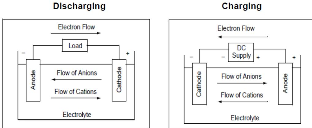
Figure 1. 15 Charging and discharging processes of a battery [12]
