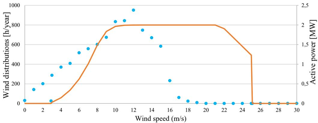
*Figure 1. 20 Distribution curve vs. power curve*
