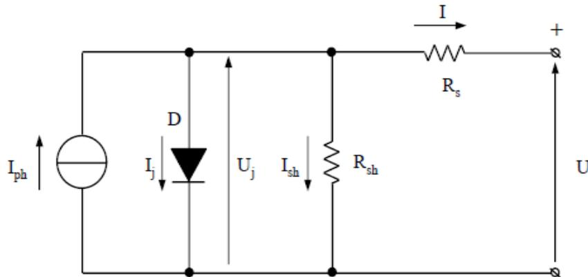
*Figure 1. 5 Equivalent circuit of solar cell [6]*
