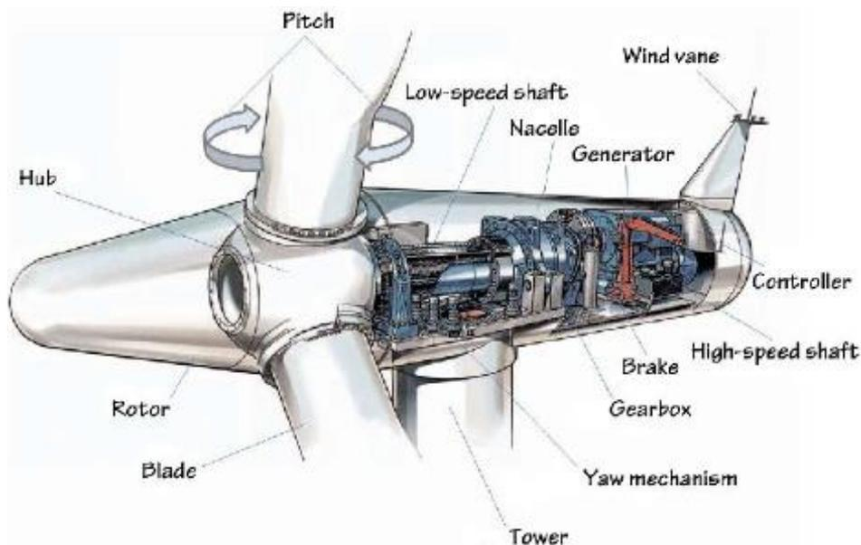
Figure 1. 14 Components of a wind turbine [10]
