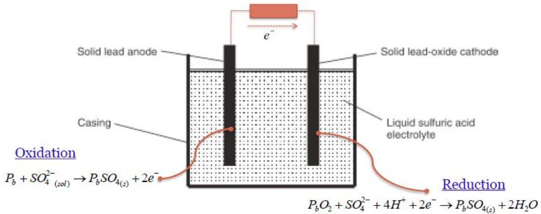
Figure 1. 16 Representation of an acid lead battery [13]
