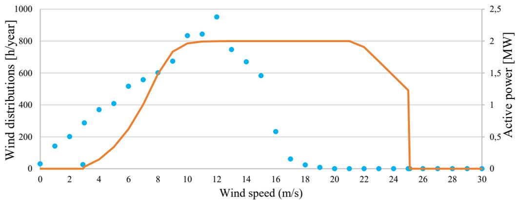
Figure 4. 9 Representation of the wind distribution and power curve of the turbine with higher productivity for Site #2
