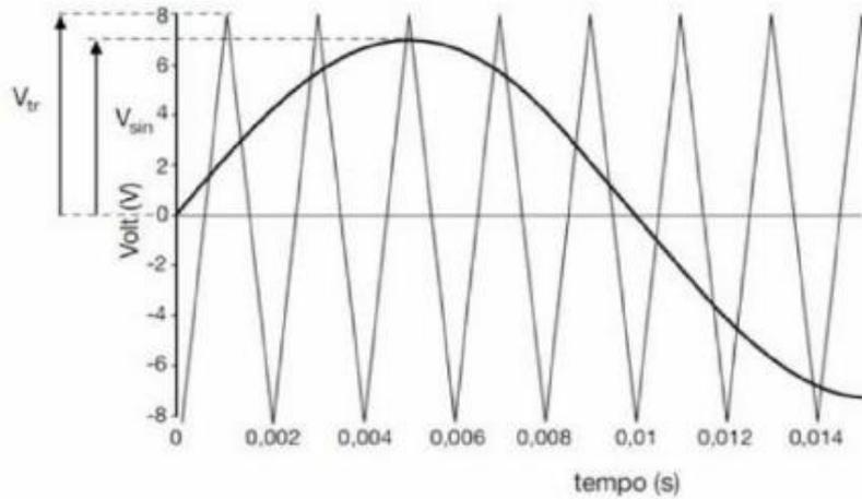
Figure 1. 11 Pulse Width Modulation technique - comparison between a sine wave and a triangle wave
