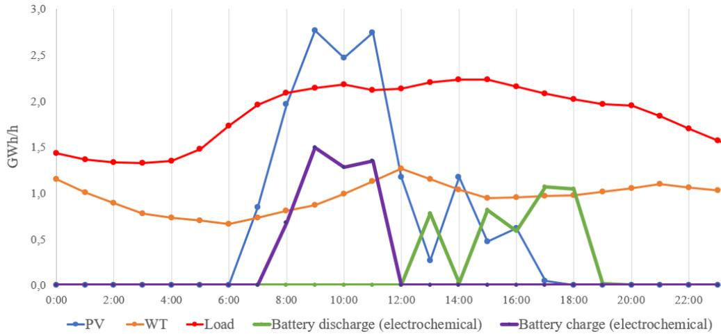
Figure 4. 13 Daily profiles with use of the storage battery, for a day with low availability of the wind resource
