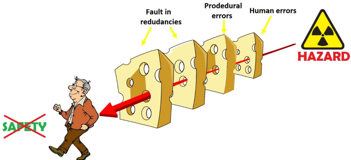
**Figure 23:** graphical representation of the Swiss Cheese Model principle. Even though there are multiple barriers, one or more failures in each one may occur; if all the holes are aligned, the person is not safe any longer.
