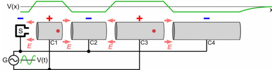
Figure 4: schematic representation of a Linear Particle Accelerator.
