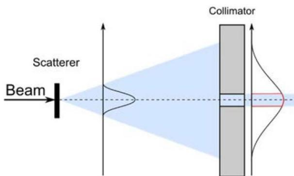
**Figure 21:** passive scattering technique for the beam size magnification during a proton therapy treatment.
