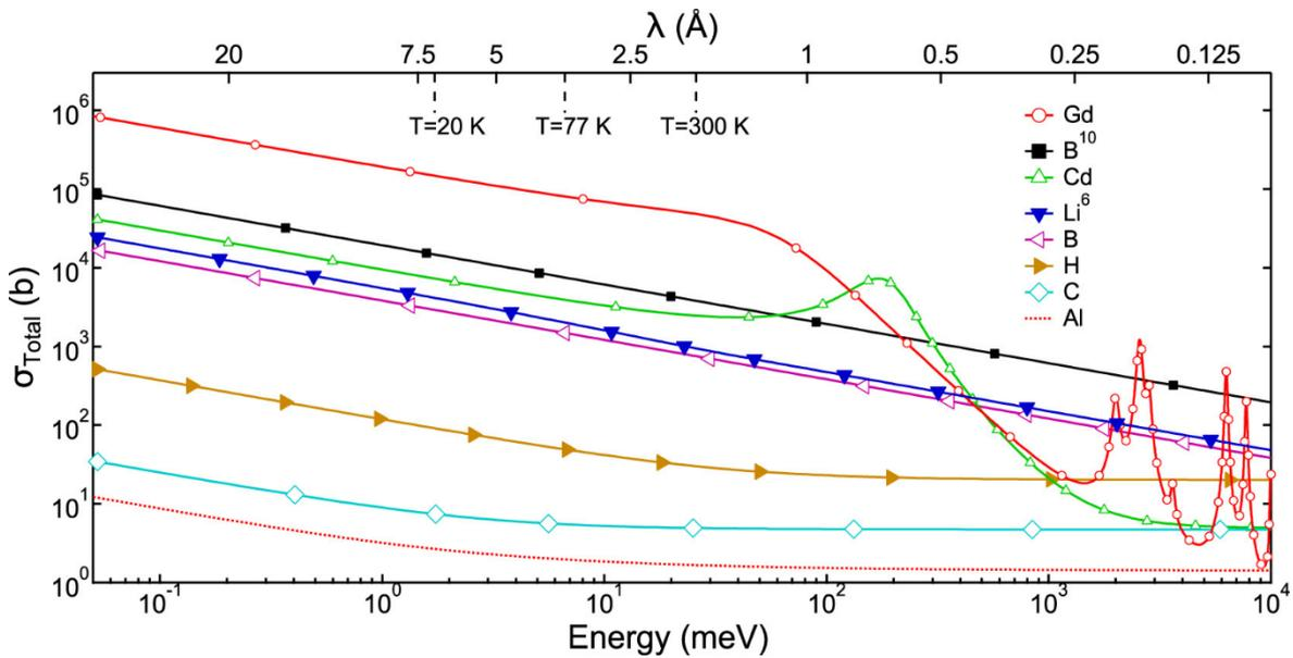
**Figure 27:** trend of the total neutron cross section (in logarithmic scale) as a function of neutron energy for several isotopes used in neutron shielding.
