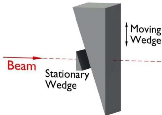
*Figure 2: schematic representation of a degrader, which aims at adjusting the ion beam energy.*
