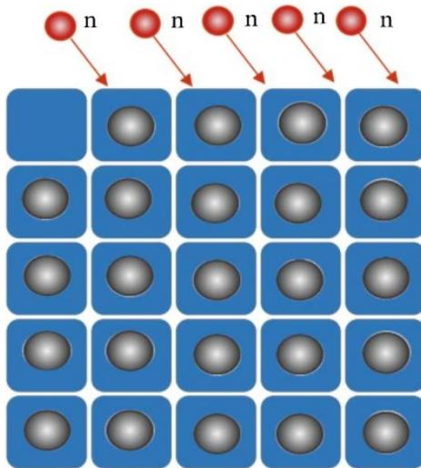
Figure 29: graphical depiction of the neutron shielding principle in a mass of borated concrete – prior to neutron collision.
