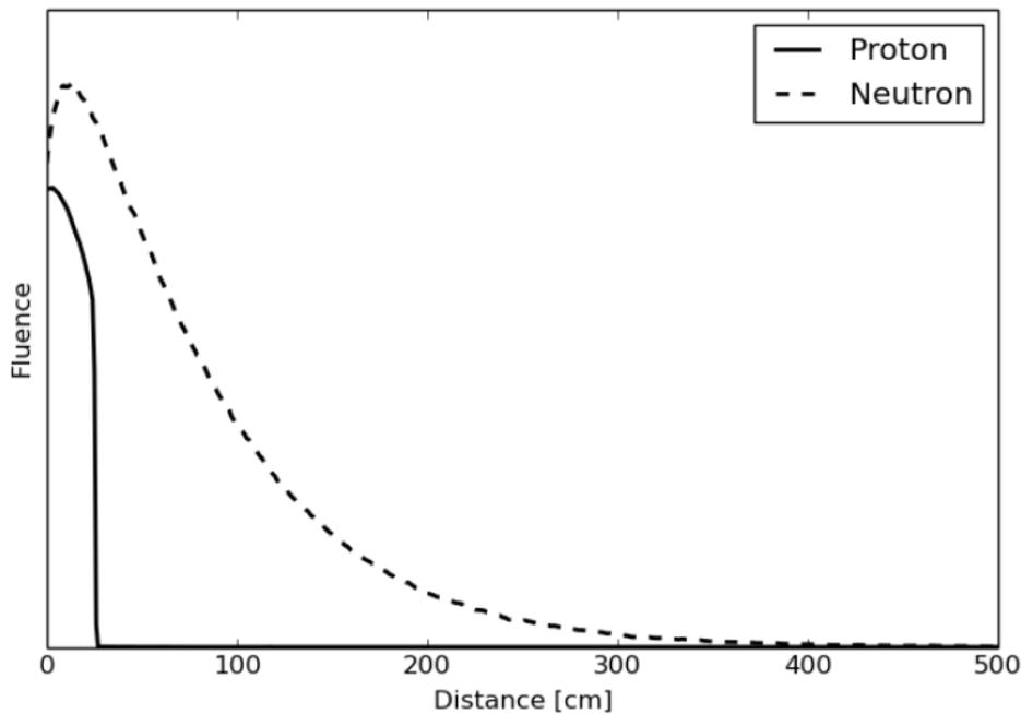
**Figure 16:** Monte Carlo simulation of fluence in water for a 220 MeV proton beam and for a 220 MeV neutron beam.
