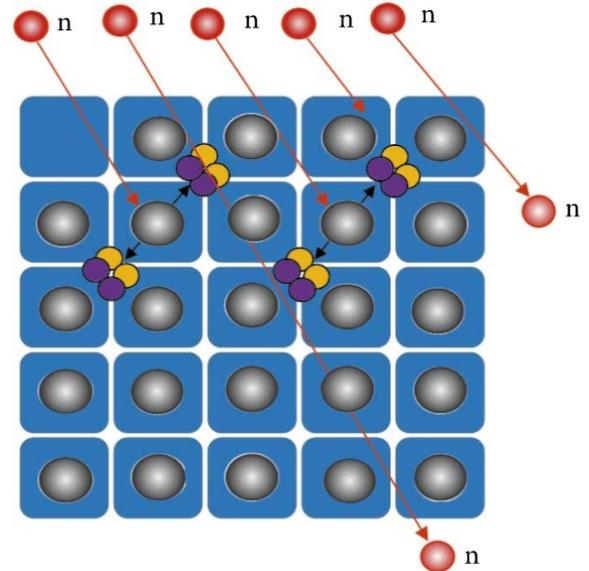
Figure 30: graphical depiction of the neutron shielding principle in a mass of borated concrete – after the neutron collision.
