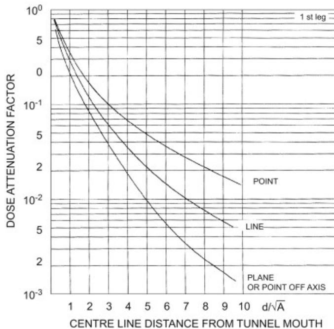
**Figure 26:** universal transmission curves proposed by CERN for the estimation of the dose attenuation factor in a duct, as a function of the ratio between the geometrical distance from the entry and the square root of the duct cross section.
