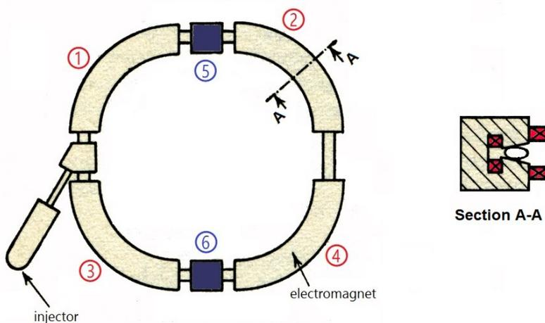
**Figure 6:** schematic representation of a Synchrotron.
