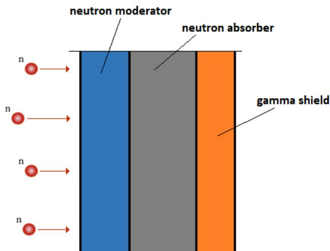
**Figure 28** illustrates the typical arrangement of a neutron shielding material wherein the three layers are parted (oftentimes denoted as *multilayer shield*) [349]. However, in the majority of proton therapy facilities the adoption of a single material which can accomplish all the three shielding functions (designed as *composite shield*) is preferred.
