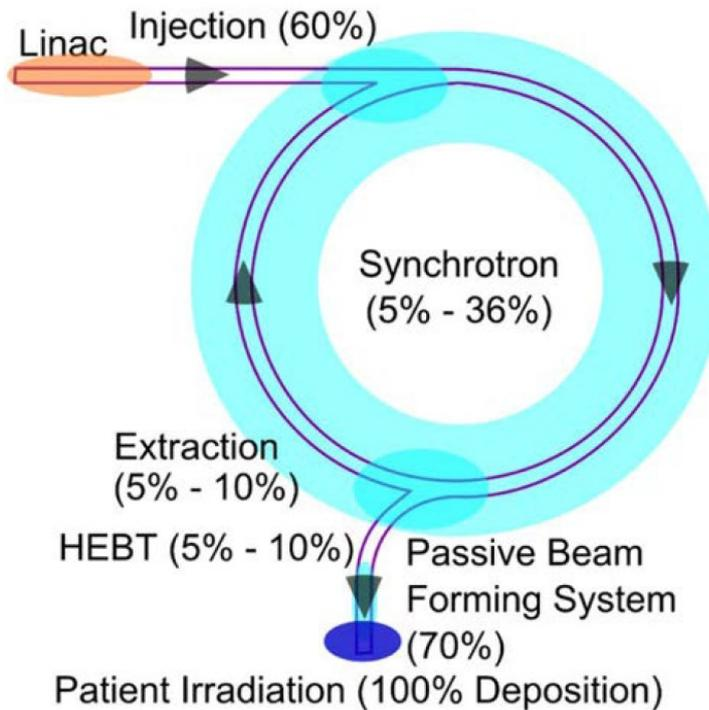
*Figure 18: indicative beam losses in a proton therapy facility utilizing a synchrotron.*
