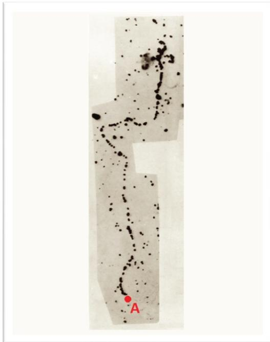
**Figure 8:** trajectory of an electron into a medium (with energy of 250 keV).
