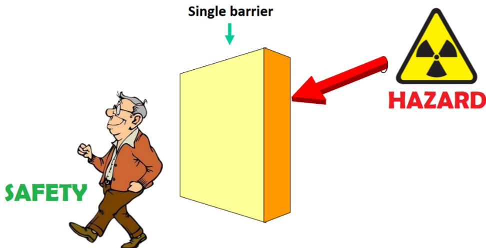
**Figure 22:** Graphical representation of the Parmesan Cheese Model principle: the condition of full safety is attained by means of a single barrier. In this model, no failure of the barrier is expected.
