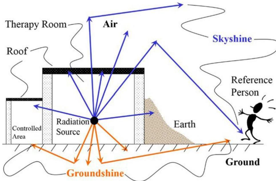
**Figure 20:** graphical depiction of the skyshine effect and the groundshine effect in a bunker of a proton therapy facility.
