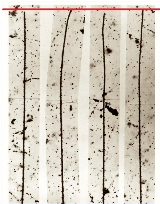
*Figure 7: trajectory of four 22 MeV  $\alpha$ -particles in photographic emulsion.*
