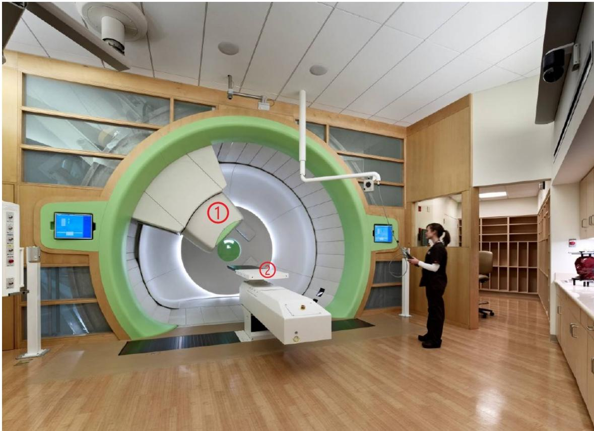
**Figure 3:** Gantry Treatment Room of IBA™ Proteus proton therapy system.
