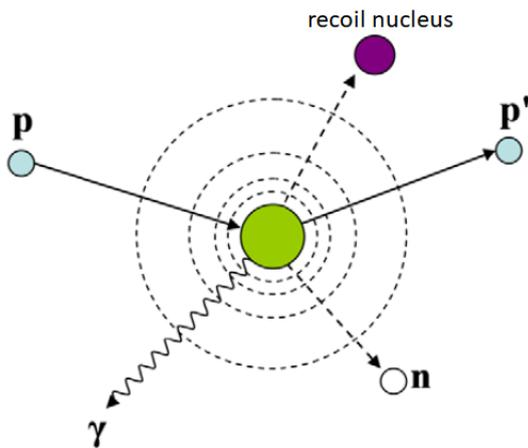
**Figure 15:** nuclear reaction between a proton (in light blue) and a nucleus (in green), with subsequent emission of a few typical particles.
