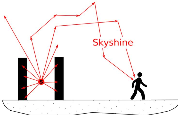
*Figure 19: graphical depiction of the skyshine effect onto a person situated at the exterior of the shielded area.*
