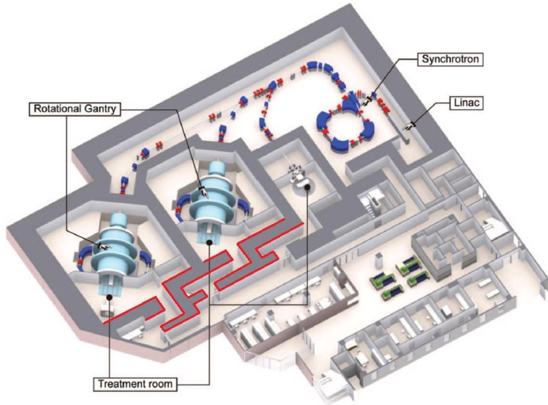
**Figure 25:** layout of Fukui Prefectural Proton Therapy Centre of Japan. One of the shielding mazes is highlighted in red lines.
