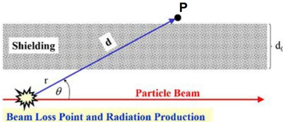
**Figure 32:** example of application of a line-of-sight model for the dose estimation in point  $P$  (provided an assumption on the thickness  $d_0$ , on the distance  $d$ , on the angle  $\vartheta$  and on the localization of the beam loss).
