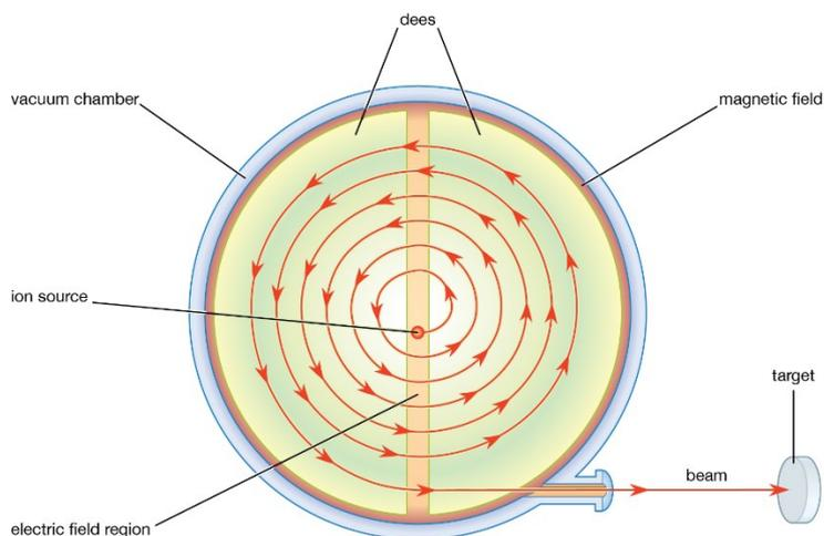
**Figure 5:** schematic representation of a Cyclotron Accelerator.
