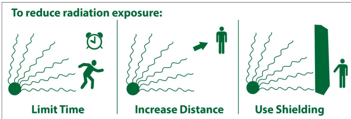
*Figure 24: Graphical illustration of the “time-distance-shield” principle.*
