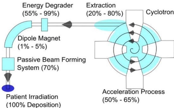
*Figure 17: indicative beam loss repartition in a proton therapy facility utilizing a cyclotron.*
