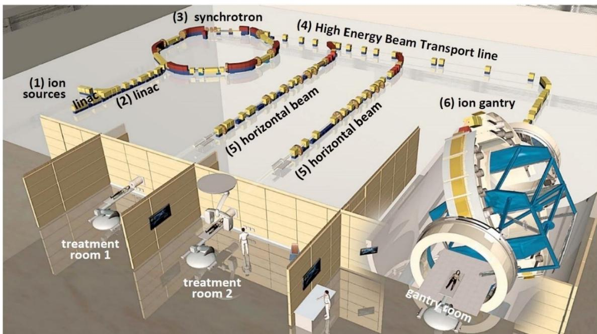
**Figure 1:** layout of Heidelberg Ion-Beam therapy Centre (HIT) in Germany.
