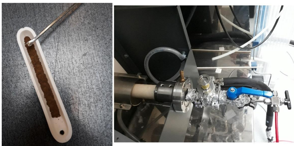
Figure 42: Reactor configuration with alumina crucible.
