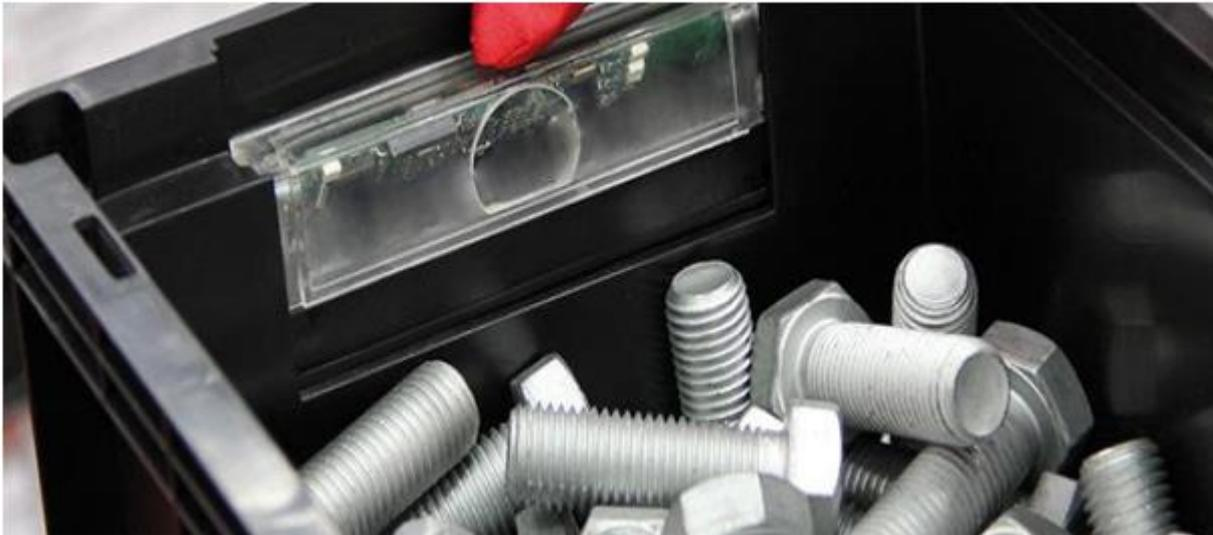
Figura 15: SENSORE E-KANBAN IMPLEMENTATO IN UN CONTENITORE (WURTH INDUSTRIE, 2018).
