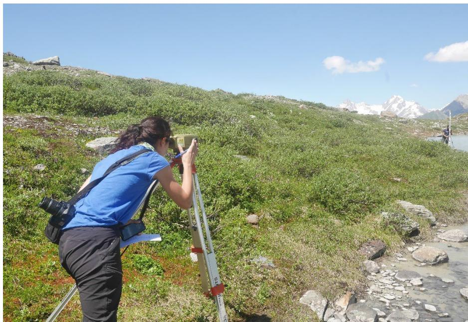
Figure 23 Levelling the free surface of Serac lake
