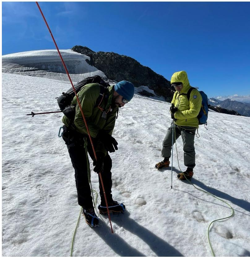
Figure 32 Probe sampling to measure ice thickness
