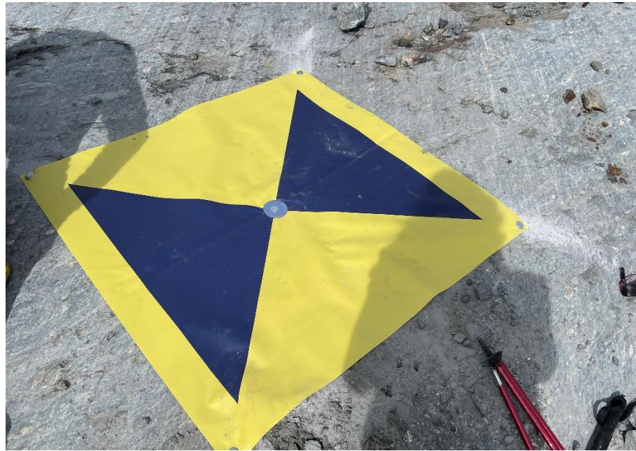
Figure 33 Marker on the glacier to set a GCP 1m x 1 m
