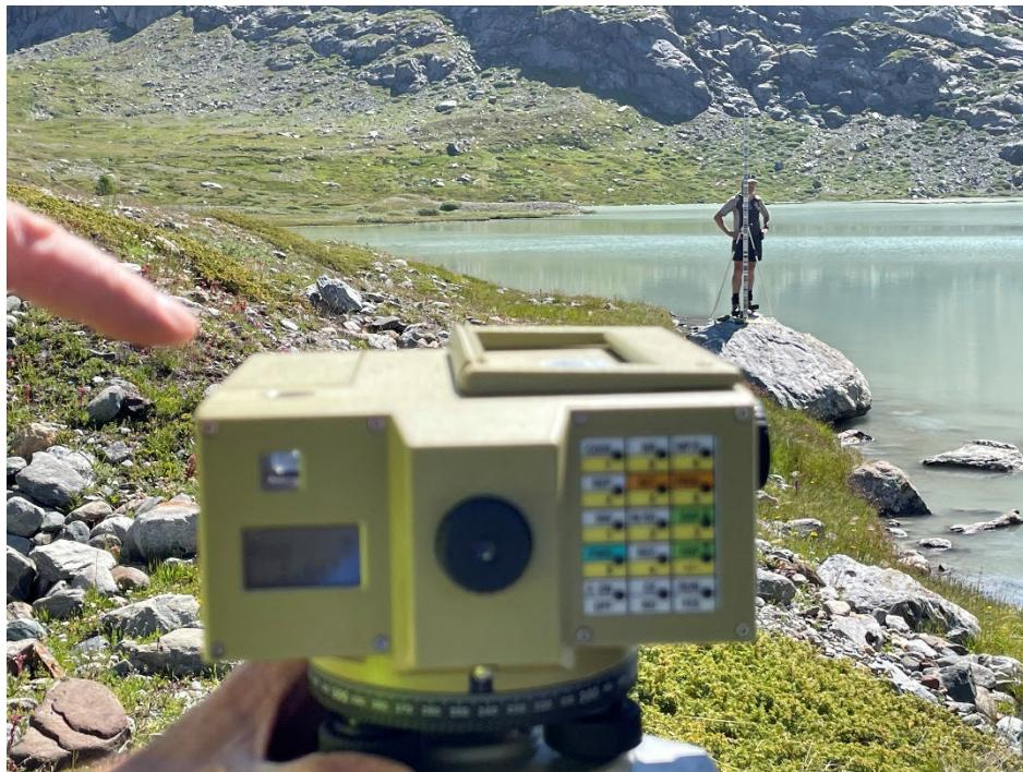
Figure 24 Levelling the free surface of Serac lake
