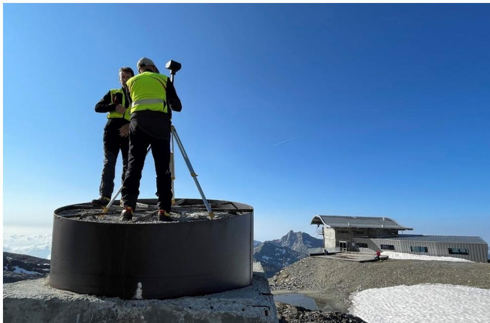
Figure 128 RTK station INDREN 1 base station
