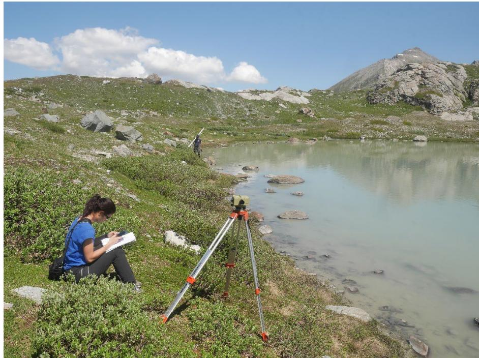
Figure 25 Levelling the free surface of Serac lake
