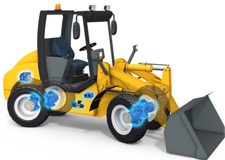
Figure 1.13 – Mini loader and its hydraulic components
