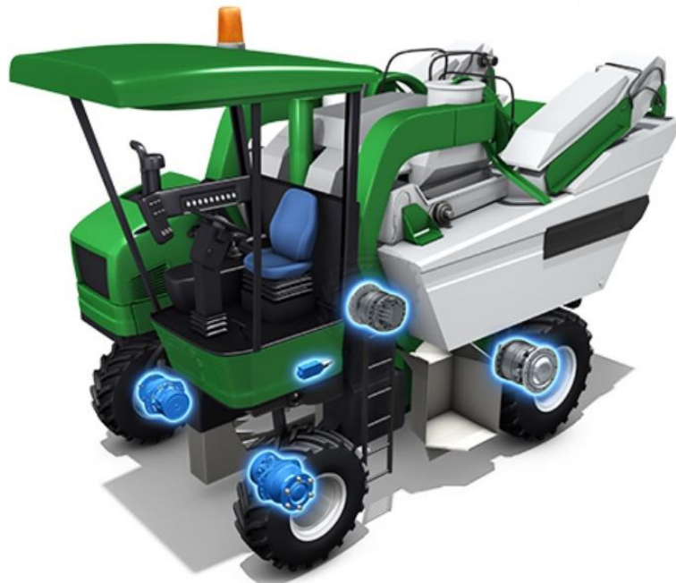
Figure 1.17 - Grape harvester and its hydraulic components
