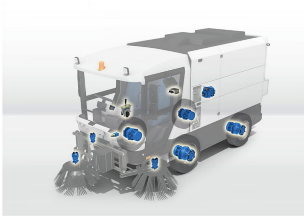
Figure 1.16 - Sweeper and its hydraulic components
