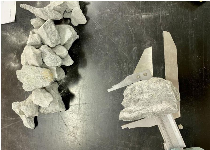
Figure 25. The particle double caliper used to perform the shape index
