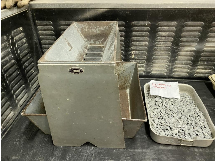
Figure 24. The Jonson separator used to obtain the particle size fraction.
