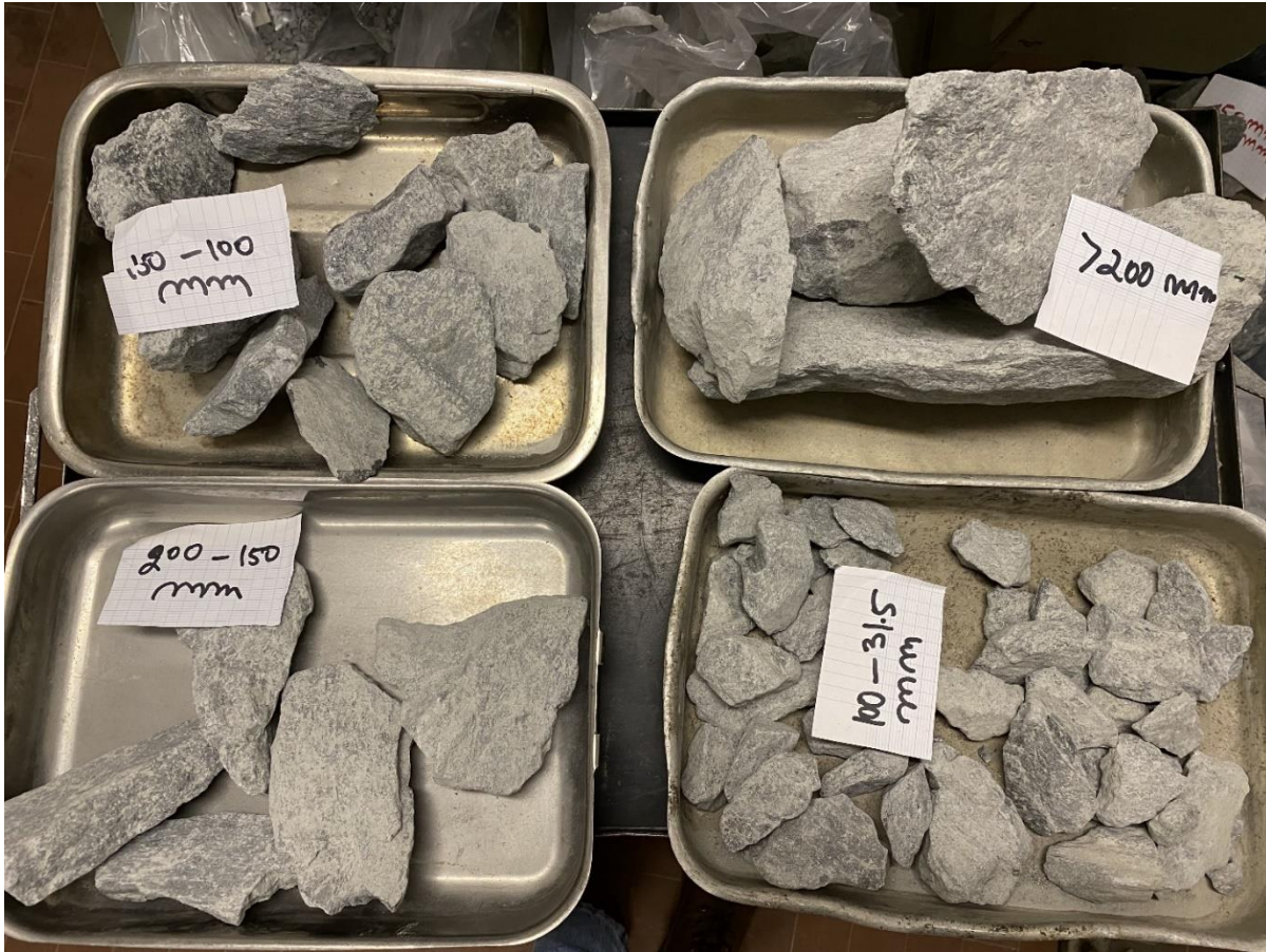
Figure 22. Example of the sieved boulder/ cobbles particles with D \geq 31,5 mm that were performed manually.
