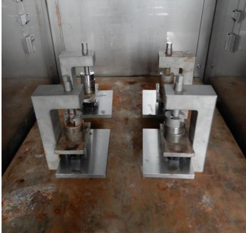
*Figura 17 Sistemi c-clamp inseriti in camera climatica*
