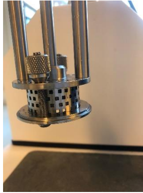
Figure 12. Homogenizer working head used to homogenize raw material in NaOH solution
