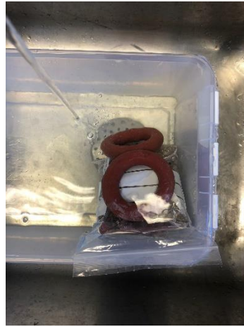
Figure 11. Thawing of raw material (stored at -80^{\circ}\text{C} ): raw material inside sealed zip bags immersed in water with cold water running
