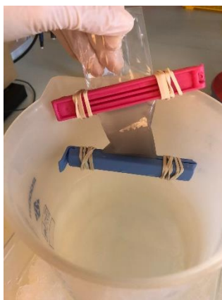
Figure 16. Dialysis setup used to remove salt from collagen recovered via salting out (SO): dialysis bags are sealed using clamps and rubber bands and immersed in the solution in a plastic beaker.
