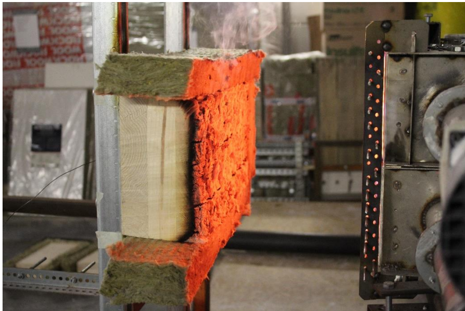
Figure 11. CLT smouldering combustion.
