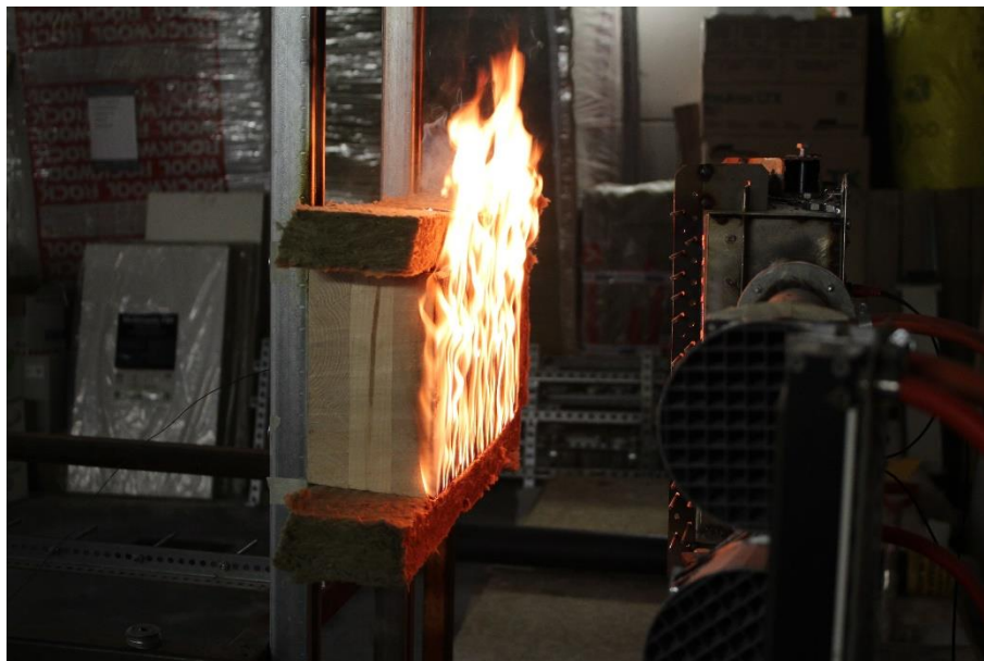
Figure 10. CLT flaming combustion.
