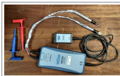
Figure 5.9: Differential probe with shielding.
