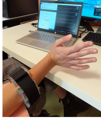
Figure 5.1: Armband's electrode disposition referenced to the forearm muscles. On the left, the forearm section from distal to proximal. On the right, armband positioning during an acquisition session.
