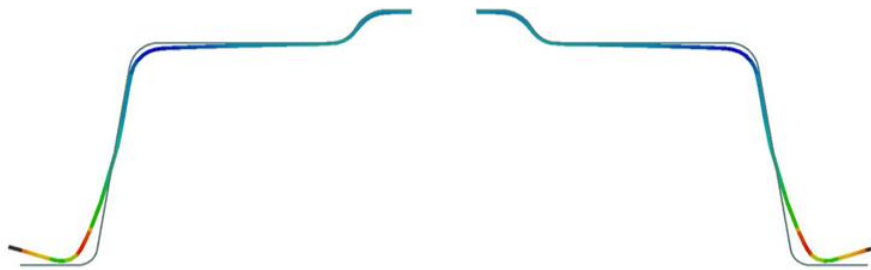
Figure 110: Simulation of the stamping operation without the implementation of the lock beads
