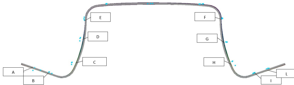
Figure 75: Schematic of comparison between actual springback measured points (blue dots) and simulated springback prediction, Hill Model
