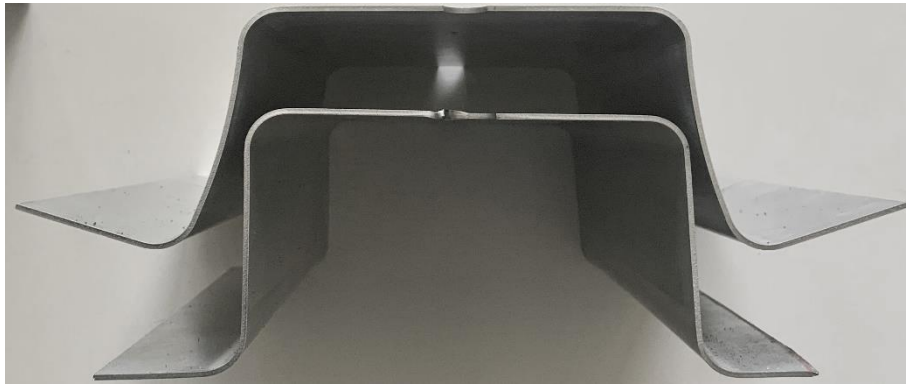
Figure 92: Picture of the stamped samples: to the top the sample stamped without lock beads, to the bottom the sample stamped with double lock beads
