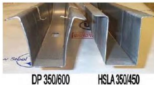
Figure 7: Comparison of two channels obtained with different materials, made sequentially in the same die.
