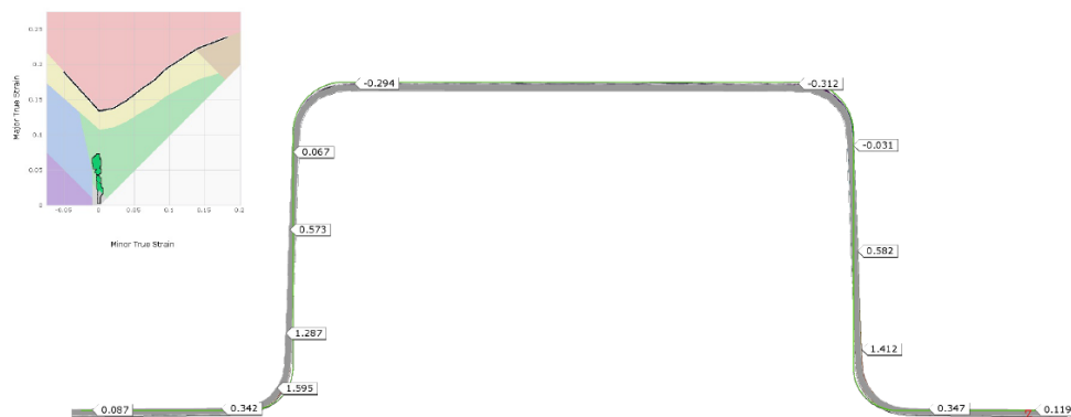
Figure 89: End of the forming process. Springback evaluation with post stretch method, Double lock beads
