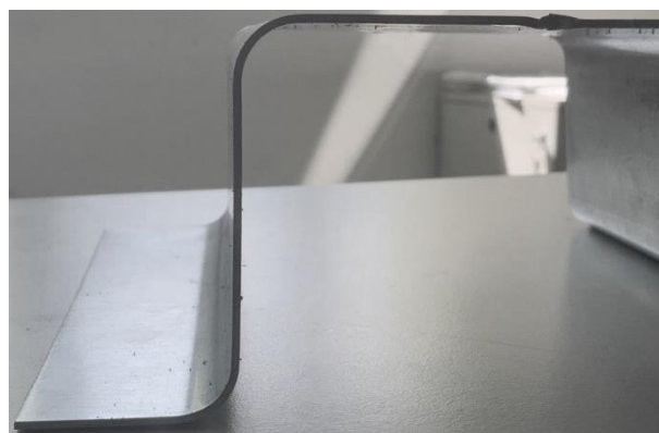
Figure 94: Picture depicting the sidewall of the stamped part with lock beads, almost null springback defect
