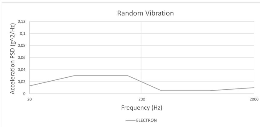
Figure 2.24: ELECTRON Random Vibration Maximum Predicted Environment
