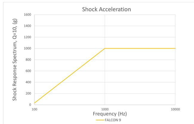
Figure 2.16: Falcon 9 induced Shock Loads
