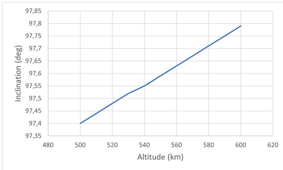
Figure 2.1: Inclination changes between 500 km and 600 km
