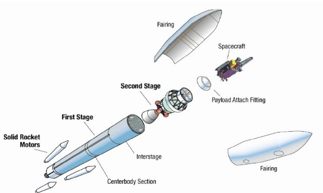
Figure 1.1: Delta II configuration for SMAP observatory [2]
