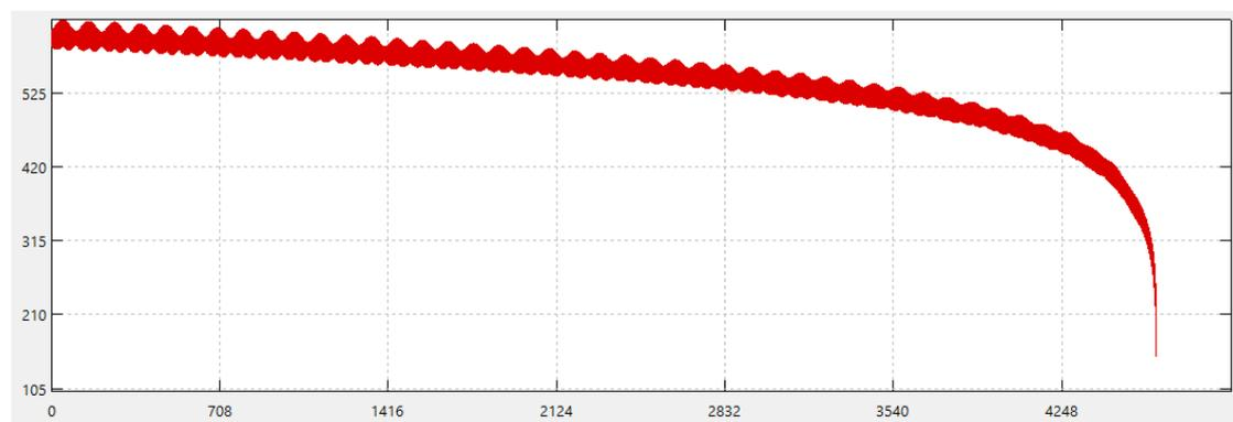
Figure 2.7: Orbit Altitude vs Mission Elapsed Days
