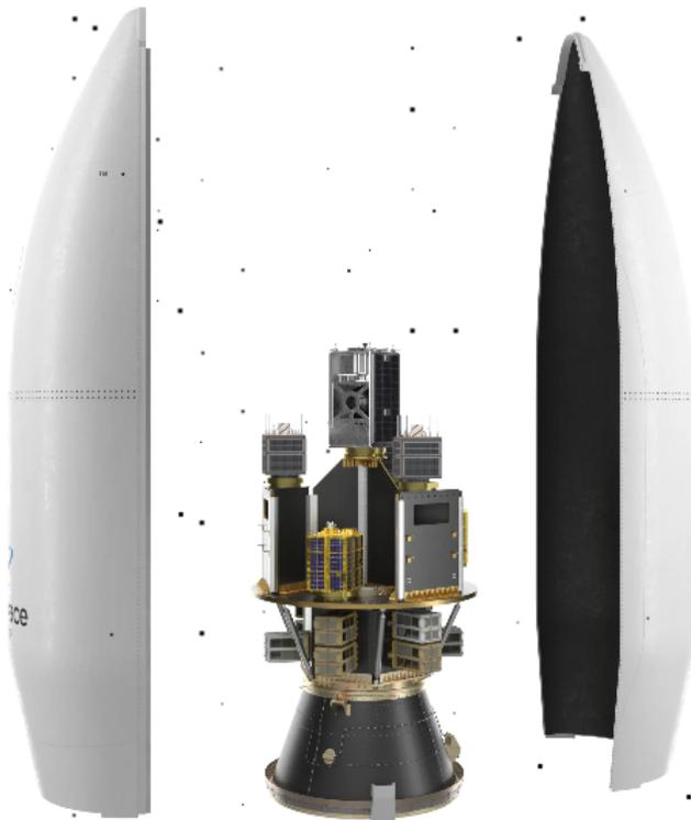
Figure 1.3: Vega-C example render for Small Spacecraft Mission Service [5]
