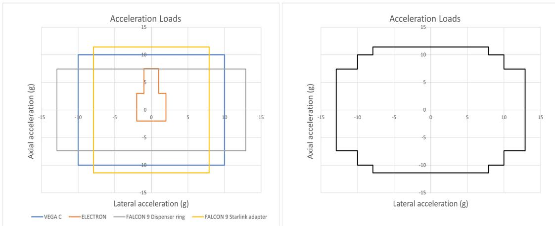
Figure 2.25: Launch Vehicles Loads Factor, all (left) and overall (right)
