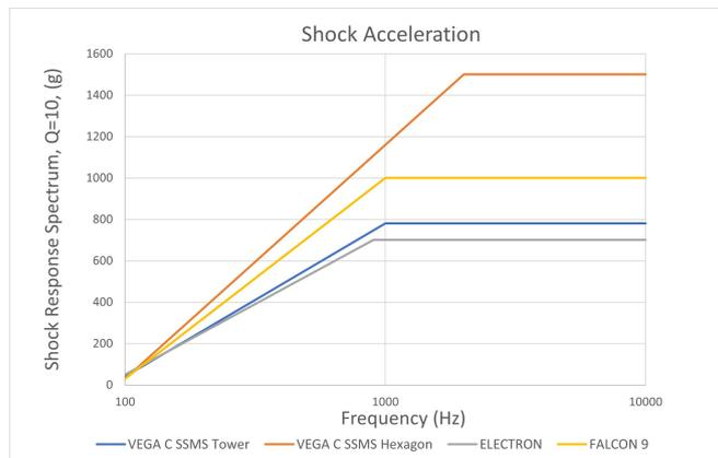
Figure 2.26: Launch Vehicles induced Shock Loads
