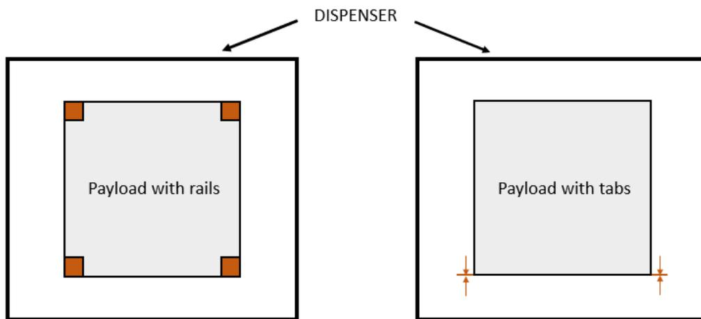
Figure 2.10: Rails and tabs configuration illustration
