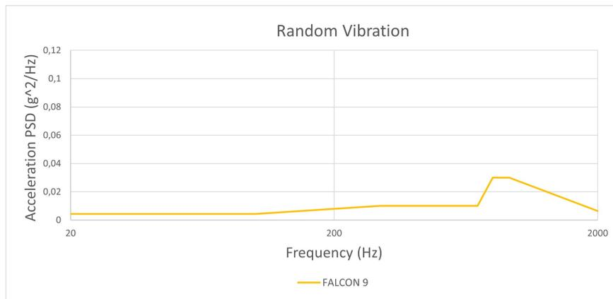
Figure 2.17: Falcon 9 Random Vibration Maximum Predicted Environment
