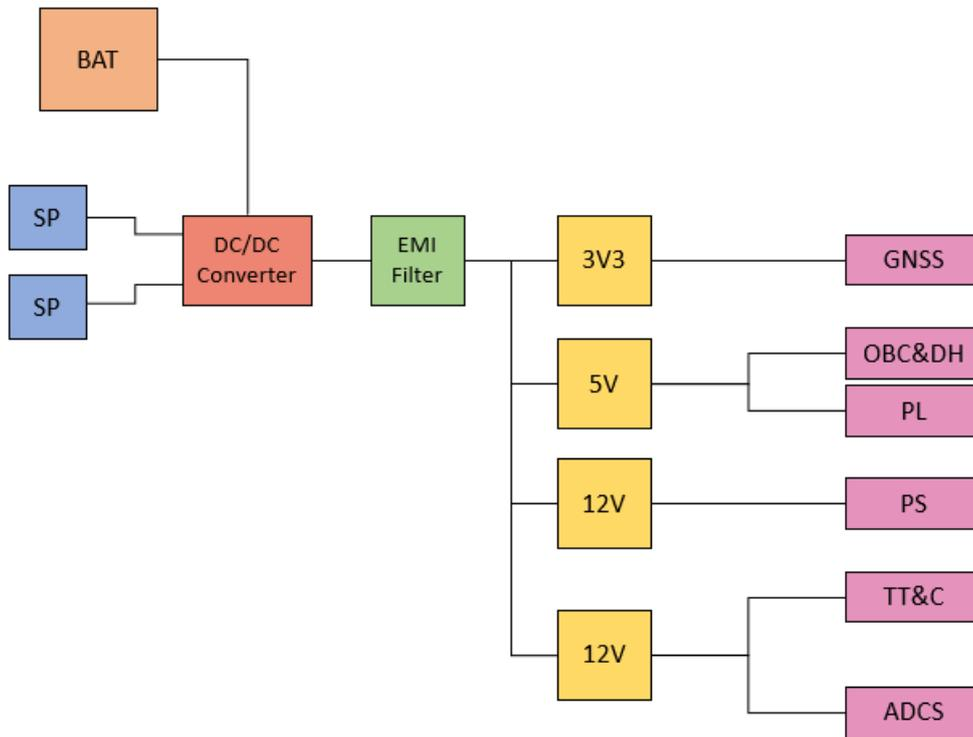
Figure 2.34: PDCU Preliminary Block Diagram
