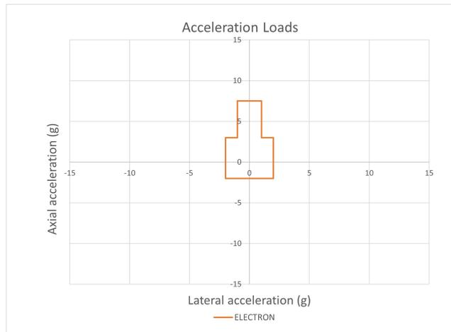
Figure 2.22: ELECTRON Loads Factor
