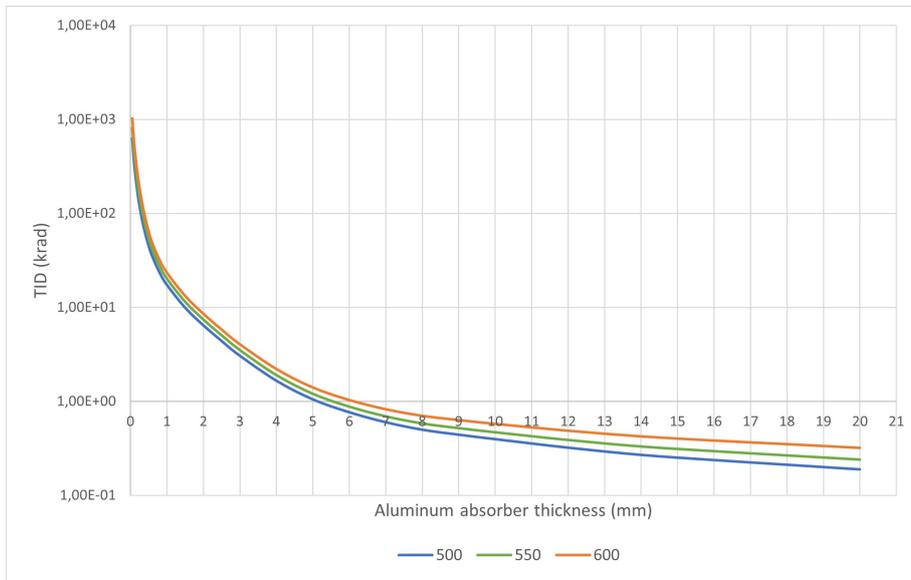
Figure 2.5: Total Ionizing Dose when varying thickness
