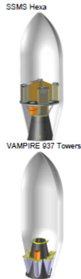
Figure 2.18: SSMS Hexagon (top) and Tower (bottom) positions
