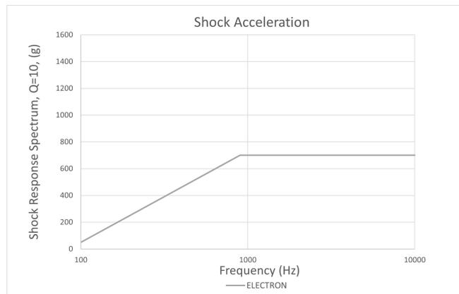
Figure 2.23: ELECTRON induced Shock Loads
