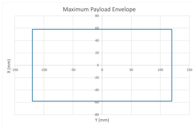
Figure 2.31: CSD's payload envelope
