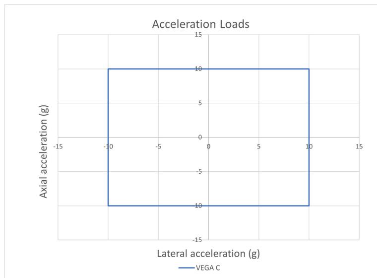
Figure 2.19: VEGA C Loads Factor for SSMS
