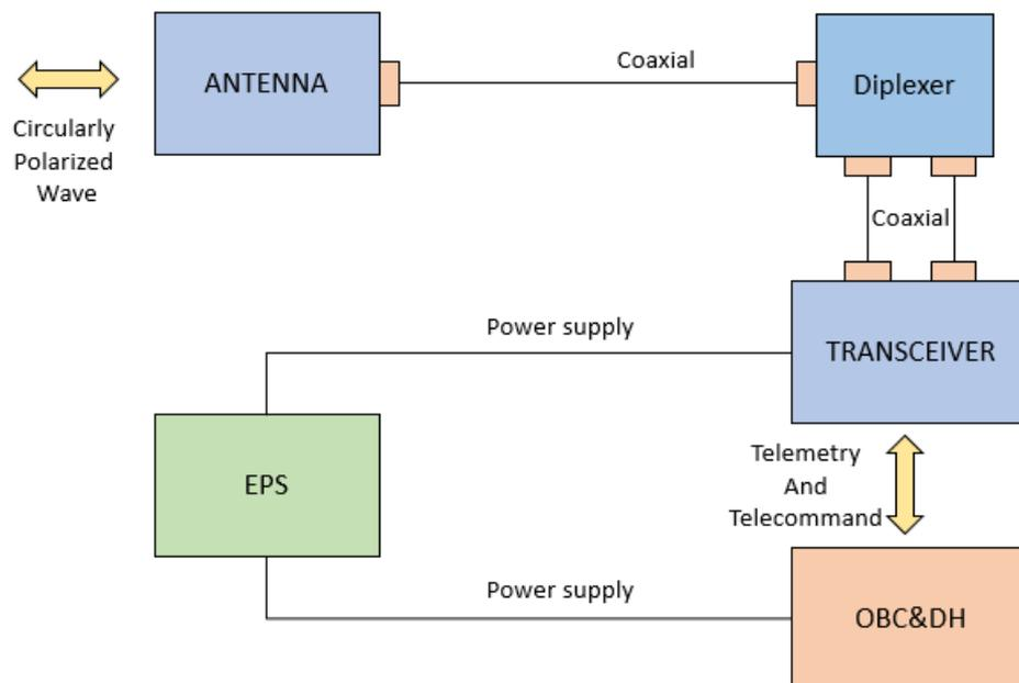
Figure 2.35: TT&C Preliminary Block Diagram
