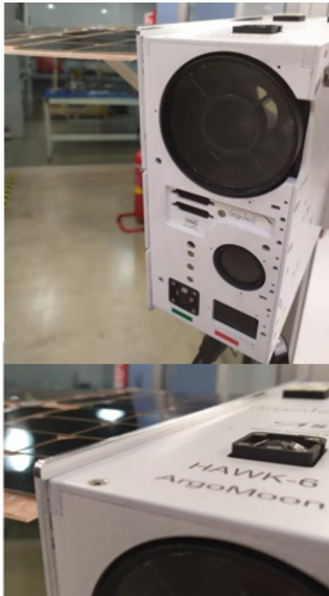
Figure 2.11: Argotec 6U platform with detailed zoom on tabs
