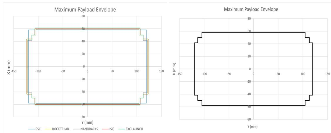
Figure 2.33: Dispenser payload envelope, all (left) and overall (right)
