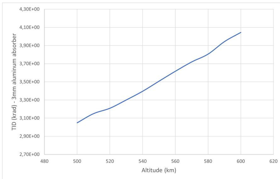
Figure 2.6: Total Ionizing Dose for a 3mm structure thickness
