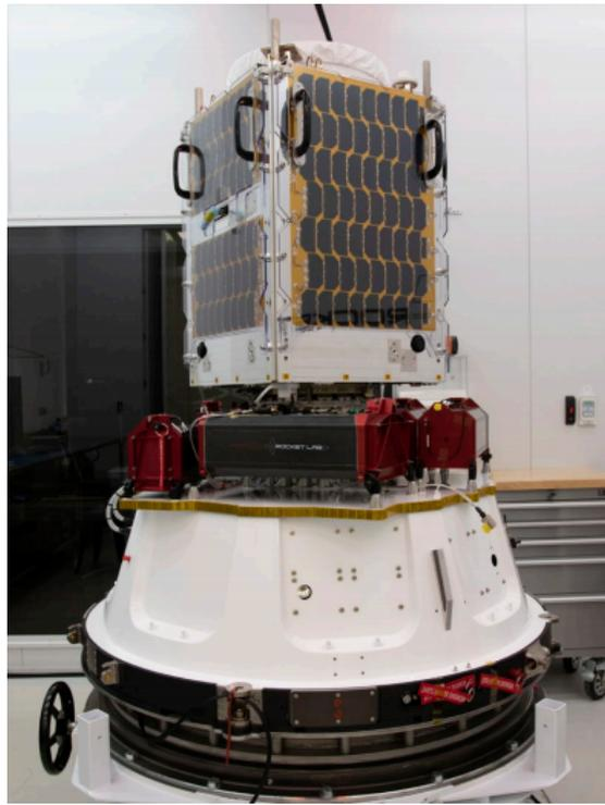
Figure 1.2: Primary (top) and secondary (bottom) spacecrafts accommodated on the Electron payload plate. Secondary spacecrafts are contained in Rocket Lab dispenser [3]
