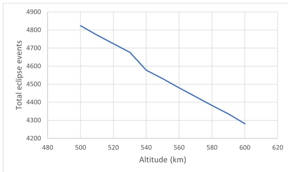
Figure 2.2: Total eclipse events when varying altitude
