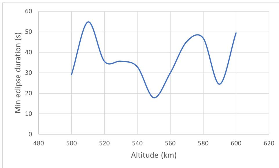
Figure 2.4: Minimum eclipse duration when varying altitude
