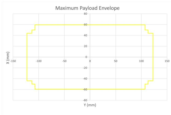
Figure 2.30: Maxwell Dispenser's payload envelope
