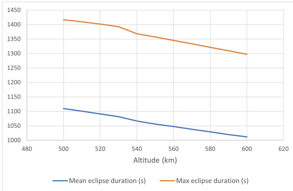
Figure 2.3: Mean and maximum eclipse duration when varying altitude
