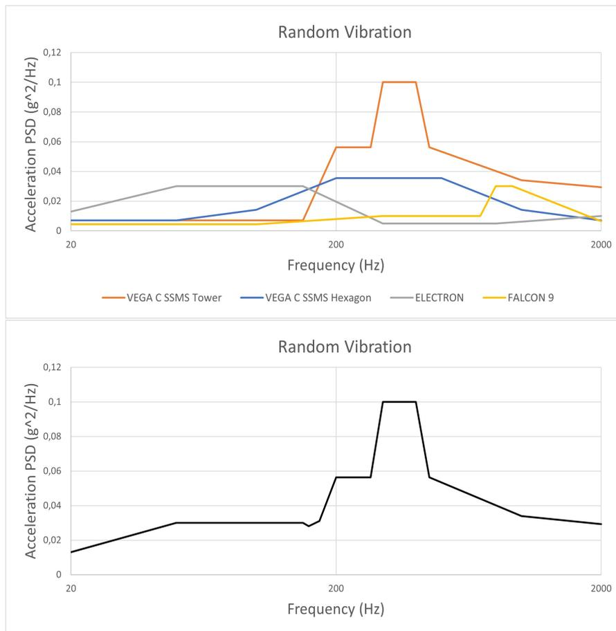
Figure 2.27: Launch Vehicles Random Vibration Maximum Predicted Environment, all (top) and overall (bottom)
