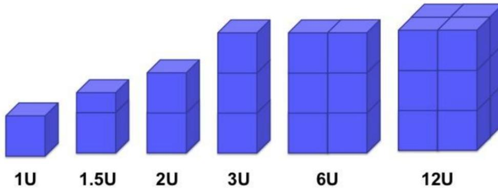
Figure 1.8: Examples of CubeSat configuration [1]
