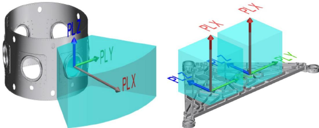
Figure 2.14: Dispenser Ring (left) and Starlink Adapter (right) models
