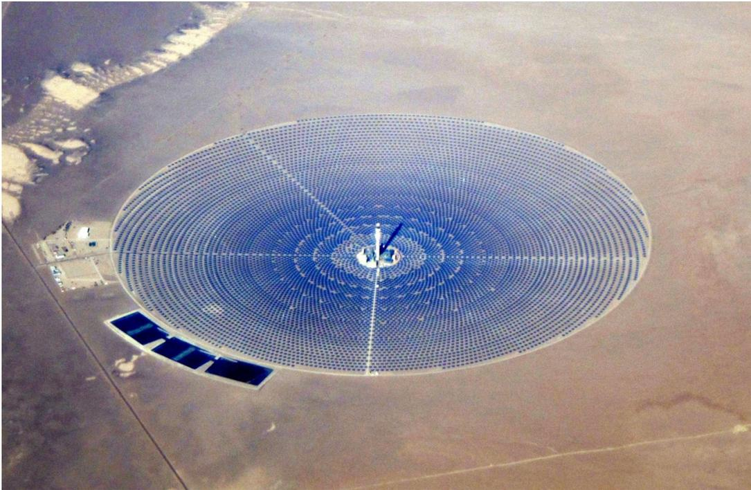
Figure 1: Solar power tower concentrating light via 10,000 mirrored [3]
