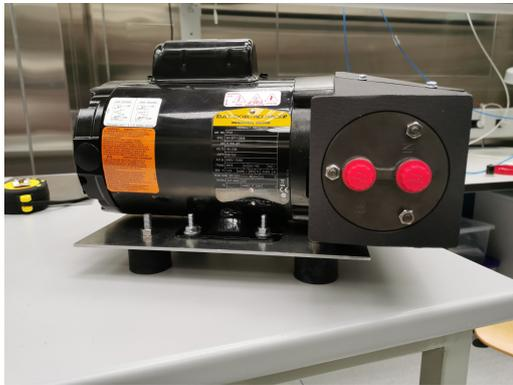
(a) Gas Pump with anti-vibration support
