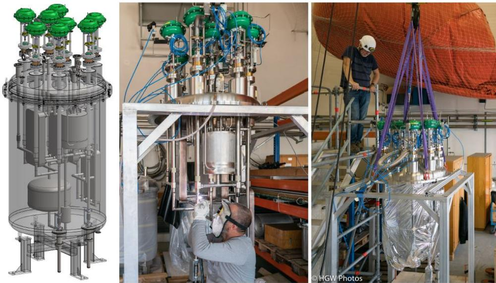
Figure 1.9: DS-20k condenser box design, fabrication and assembly
