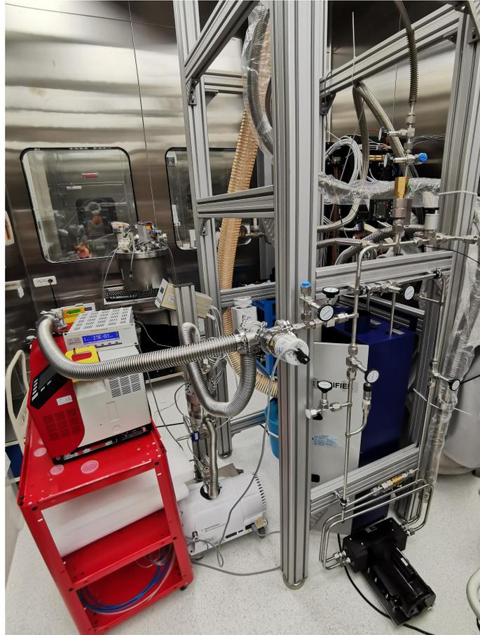
Figure 5.10: Assembled system leak test
