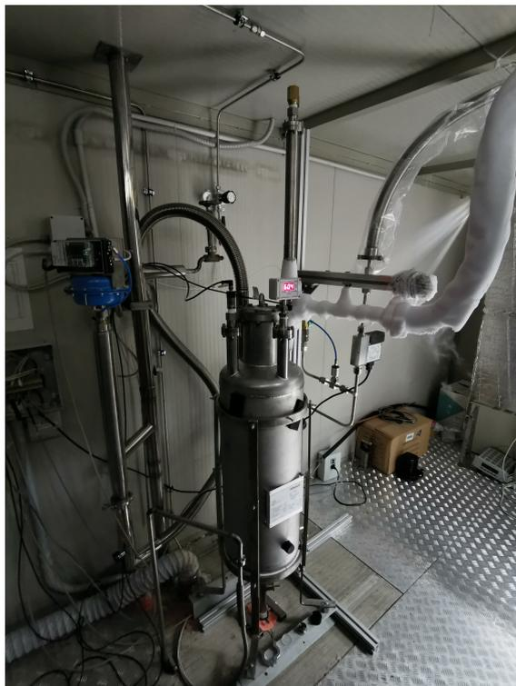
Figure 5.11: Manual vent line for the nitrogen in the N<sub>2</sub> barrel
