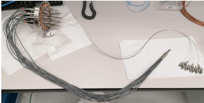
Figure 2.17: Optical splitter from one to 16 available for the light distribution
