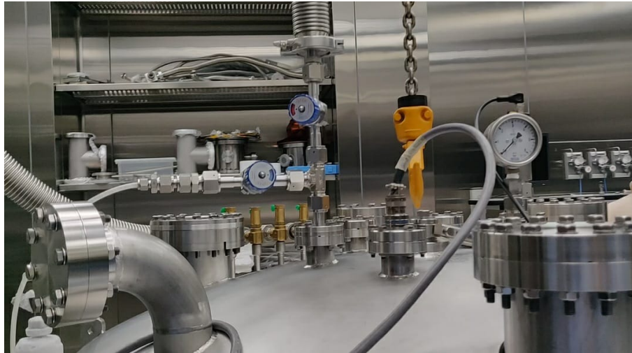
Figure 4.12: 3-way fitting with two manual valves VN2 & VN3
