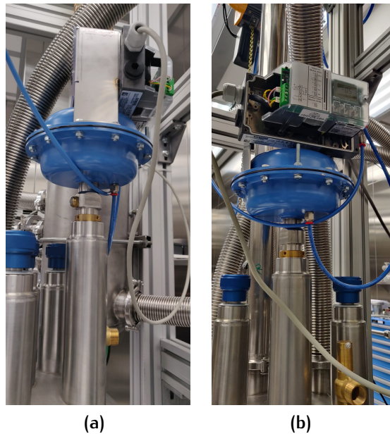
Figure 4.19: Proportional valve VC1 linked to the PXIe and controlled by Slow Control
