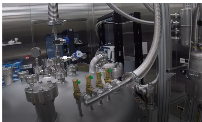
Figure 4.16: KF40 metal hose from 4 safety valves
