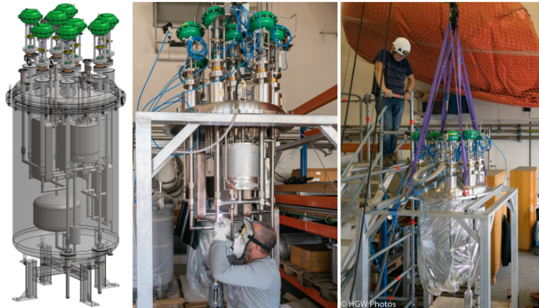
Figure 1.8: DS-20k cold box design, fabrication and assembly.
