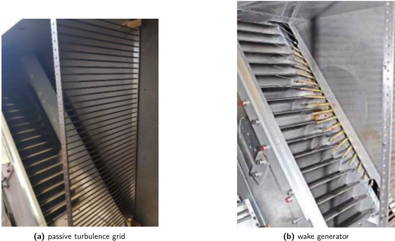
Figure 3.2: View of the passive turbulence grid (a) and of the wake generator (b)
