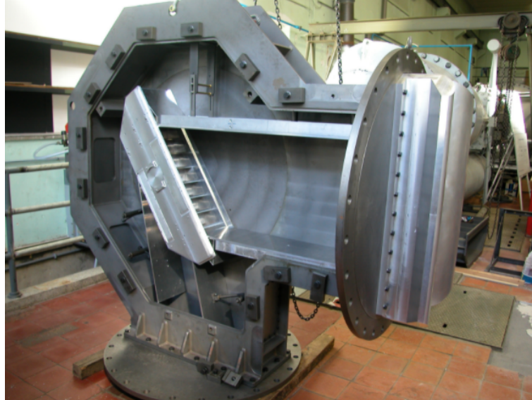
Figure 1.1: View of the test section of the VKI S-1/C high-speed low-Reynolds linear cascade
