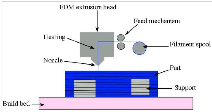
*Figure 1.17 - FDM process. Source: researchgate.net*
