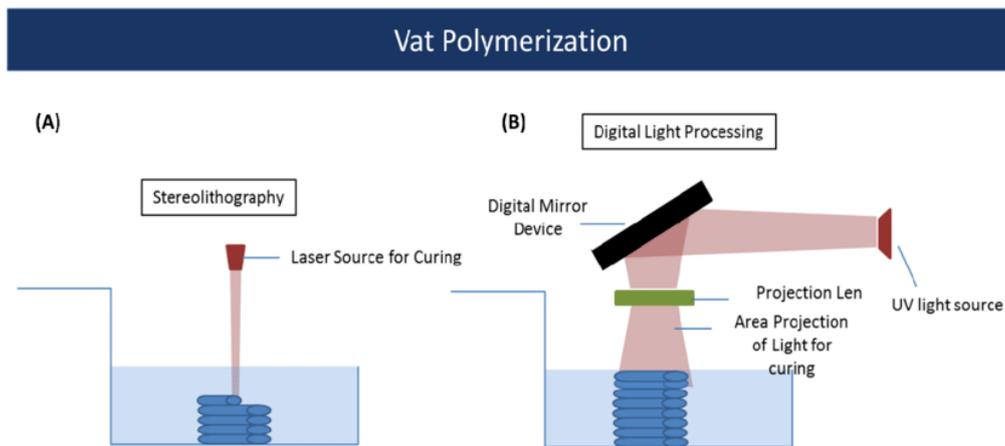
**Figure 1.6-** "Stereolithography (SLA) and Digital Light Processing (DLP) processes " [9]
