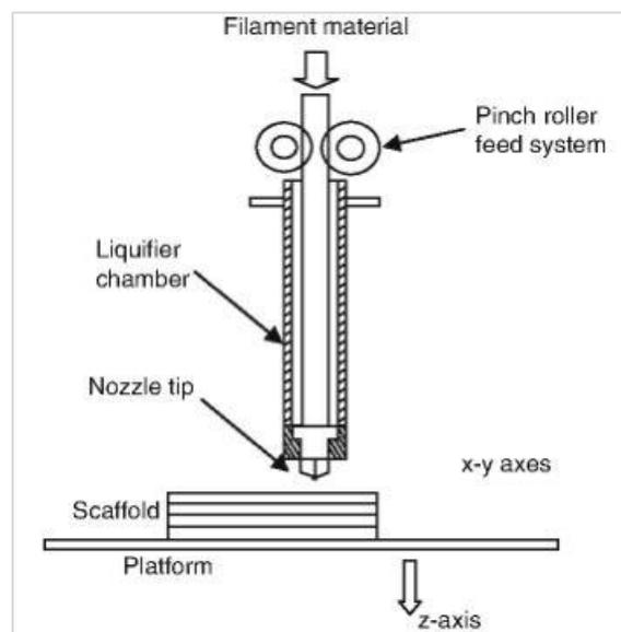
**Figure 1.12** – “Material Extrusion process”[17]
