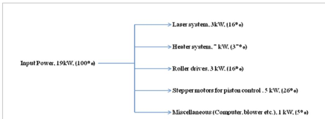
*Figure 5.7 - Power drawn by individual components. [52]*
