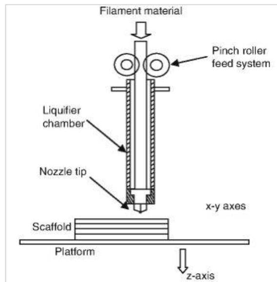
**Figure 1.12** – “Material Extrusion process”[17]
