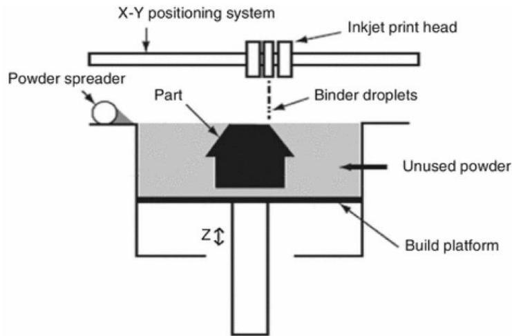
*Figure 1.9- "Binder Jetting process components" [14]*
