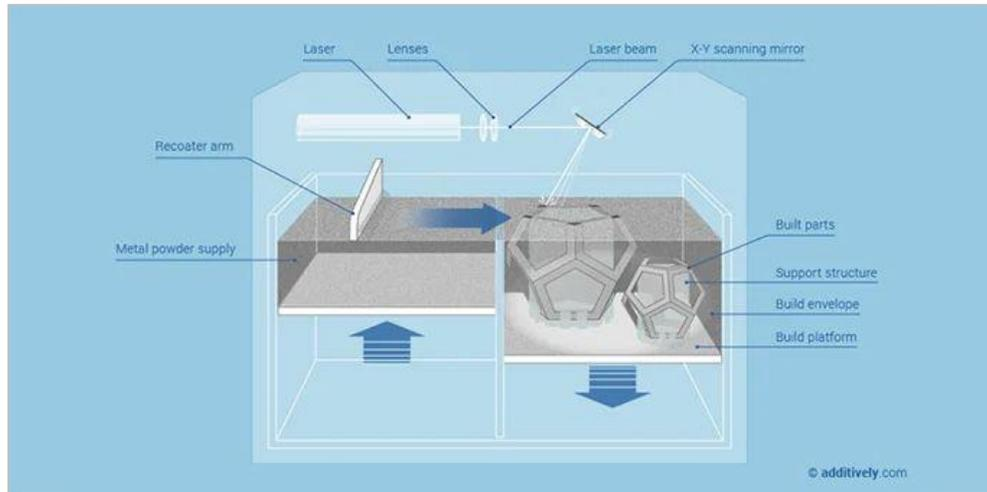
*Figure 1.20 - SLM process. Source:all3dp.com*
