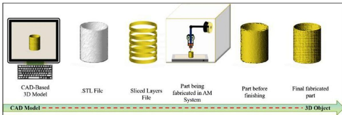
*Figure 1.2-“Basic additive manufacturing process” [4]*
