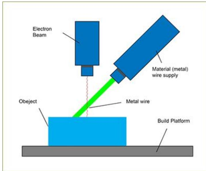
*Figure 1.10 - "Direct Energy Deposition process". Source: <https://www.lboro.ac.uk/>*
