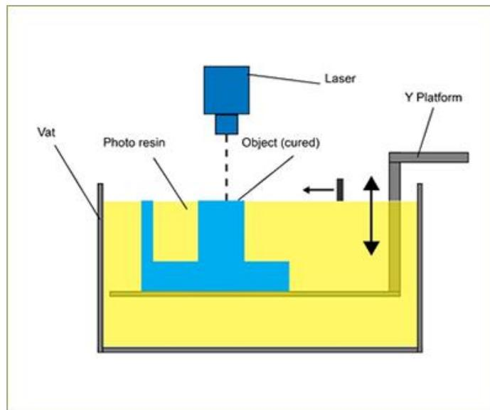
**Figure 1.5** - "Vat Photopolymerization process" [8]
