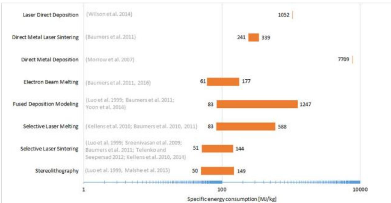
**Figure 5.8-** Specific energy consumption (logarithmic scale) for AM systems. The energy values represent the electrical energy demand of the AM systems. AM = additive manufacturing; MJ/kg = megajoules per kilogram. [55]
