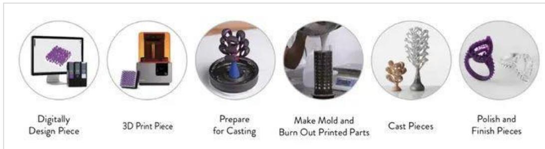
*Figure 3.2 - Direct Microfusion steps. Source: formlabs.com*
