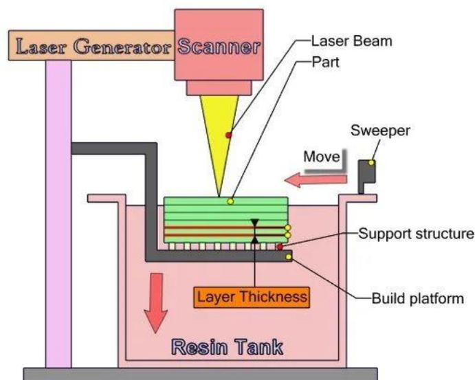
*Figure 1.7- Stereolithography (SLA) process [10]*
