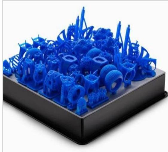
*Figure 3.1 - Jewellery prototypes 3D printed. Source: manufat.com*
