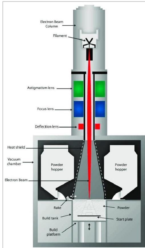
*Figure 1.19 - EBM process. Source: researchgate.net*
