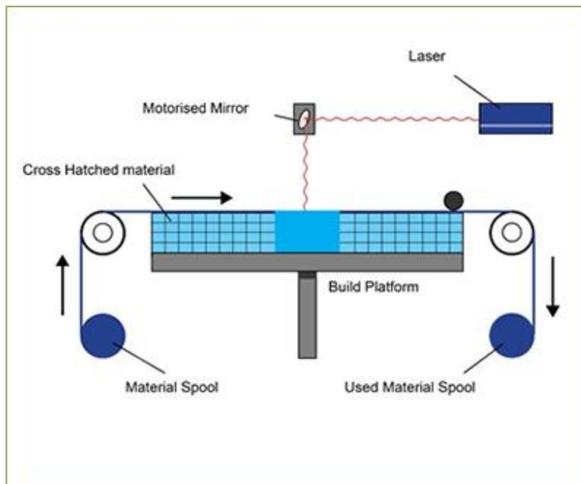
*Figure 1.11 - "Sheet Lamination manufacturing process" [16]*
