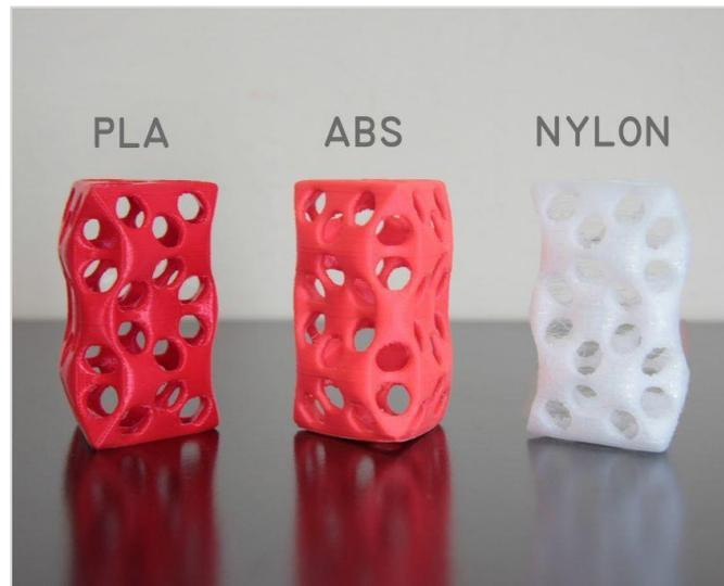
*Figure 2.6 - 3D printed parts with different materials*
