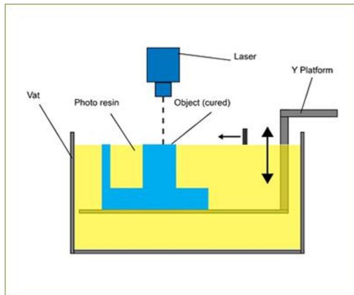
**Figure 1.5** - "Vat Photopolymerization process" [8]
