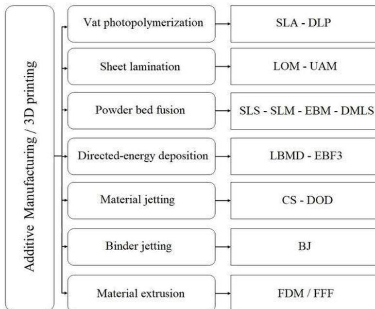
**Figure 1.3-** “Standard classification of AM technologies based on ASTM F24 Committee” [5]
