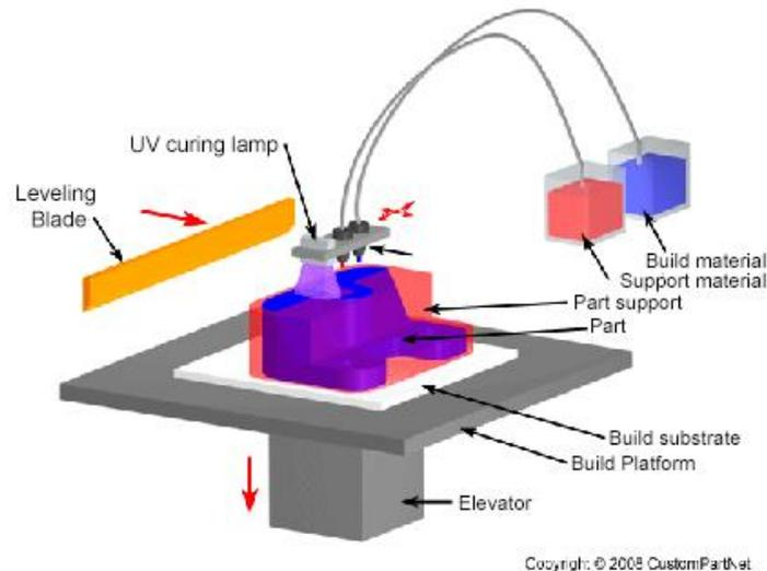
*Figure 1.8-"Material Jetting process scheme" [12]*
