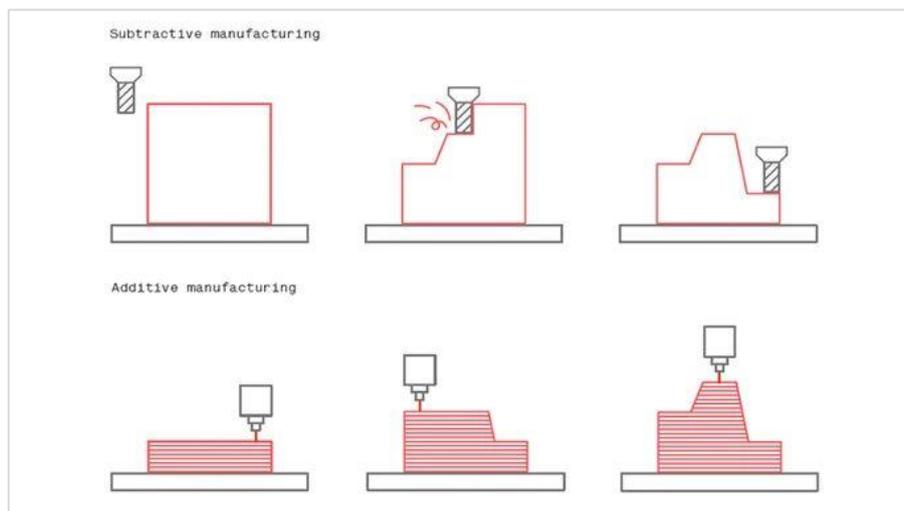
*Figure 2.5 - AM vs SM. Source: core77.com.*
