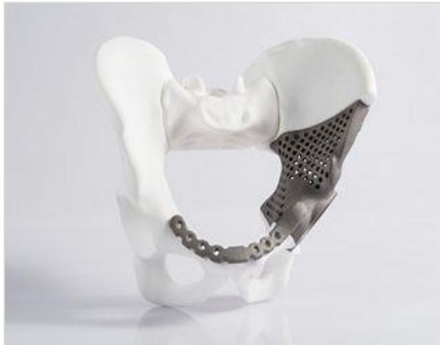
*Figure 2.8 - Titanium hip implant. Source: EOS*
