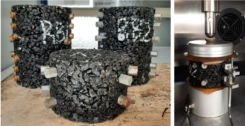
Figure 33. Samples of 130 mm and 65 mm with different gauge points
