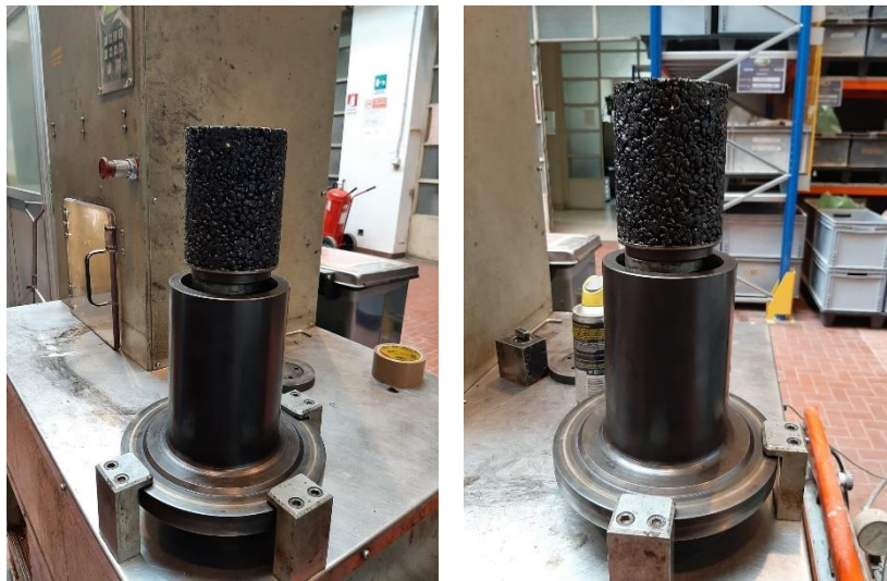
Figure 24. Specimens after compaction procedure
