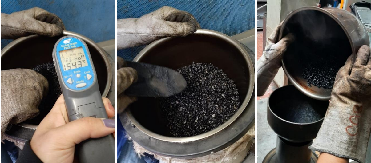
Figure 20. Mixing procedure for RA samples
