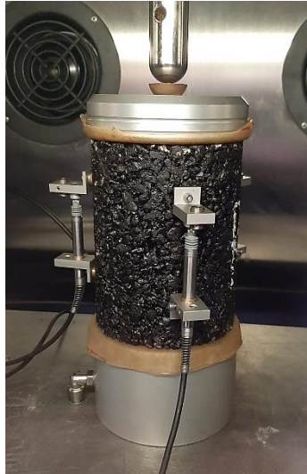
Figure 28. Configuration of Dynamic modulus test in UTM-30
