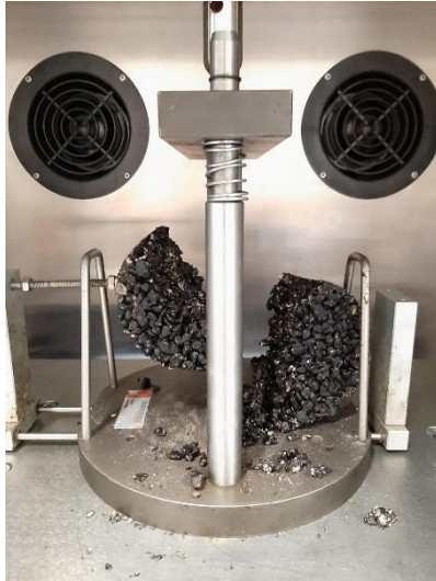
Figure 42. ITS sample break
