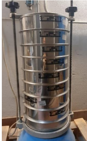
Figure 8. Automatic sieving machine
