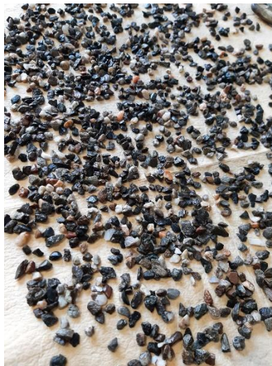
Figure 17. Sample (>4 mm) placed onto a dry cloth with saturated and surface-dried condition
