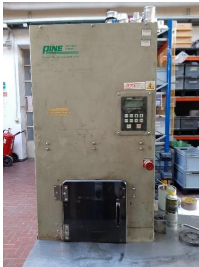
Figure 22. Gyratory compactor machine employed
