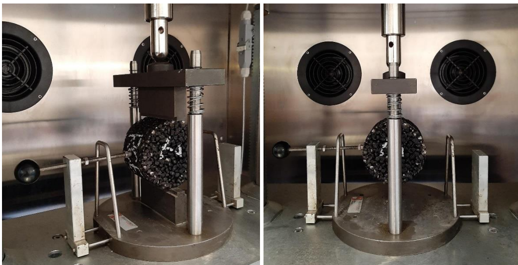
Figure 41. ITS test configuration
