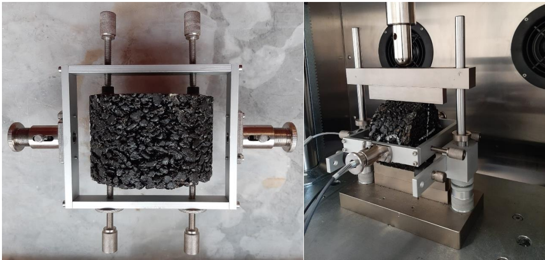
Figure 37. LVDT mounting frame and example of test equipment.
