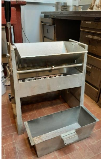
Figure 7. Riffle box employed to realize sample reduction
