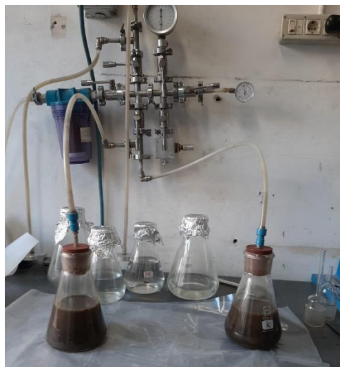
Figure 15. Pycnometers with samples immersed vacuum process
