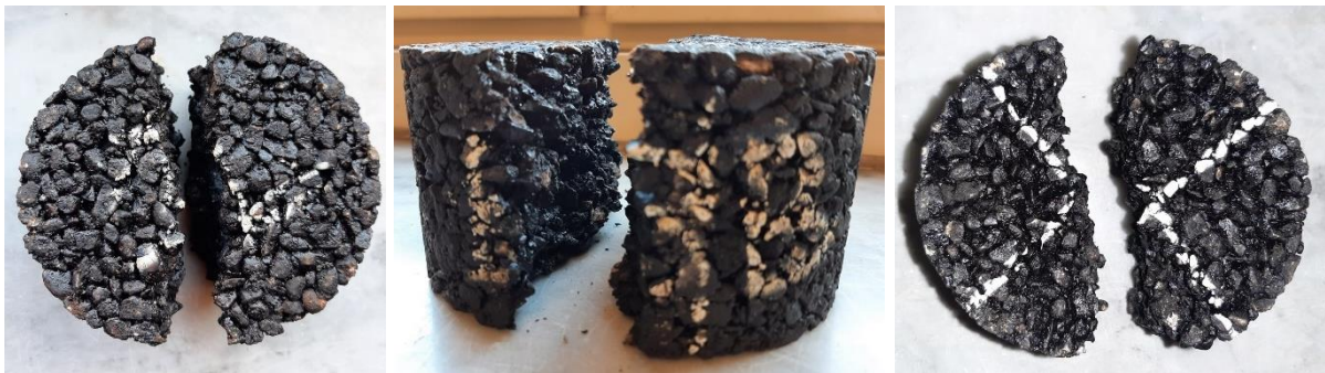
Figure 44. Samples after ITS
