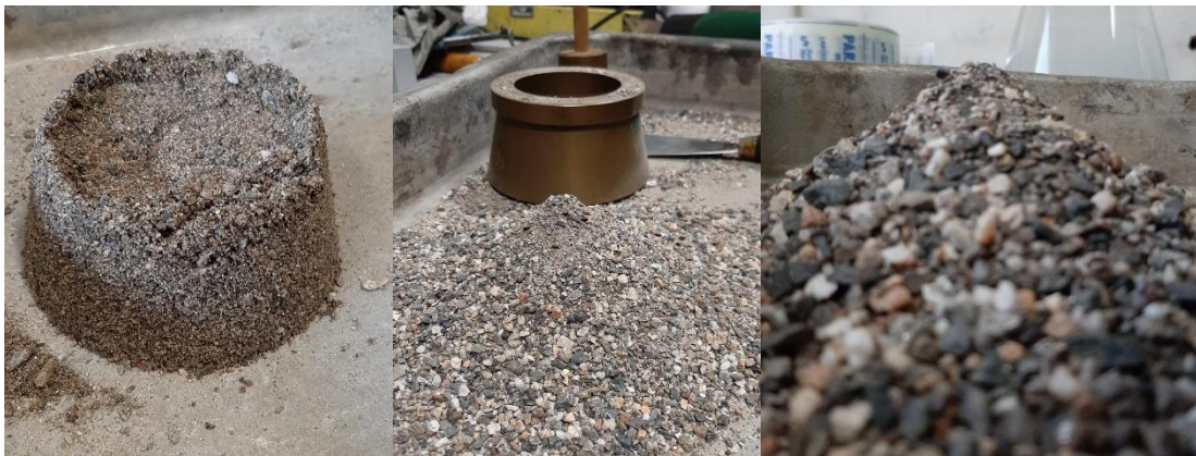
Figure 16. Procedure to obtain saturated dried surface condition
