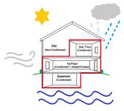
*Figure 2. Diagram of building envelope*
