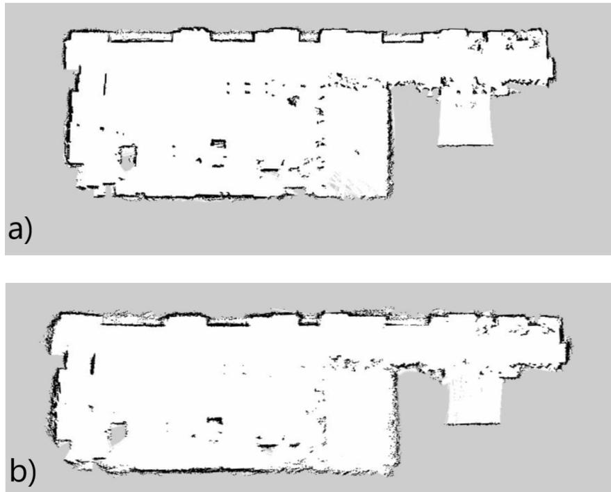
**Figure 6.18:** Map acquisition of the CIM 4.0 environment. In figure (a) in the upper part of the image it is possible to see the accurate acquisition with only one LiDAR. Instead in figure (b) in the lower part, it is possible to see the less accurate acquisition of the map with two LiDARs.
