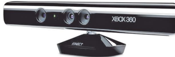
**Figure 3.2:** Microsoft Kinect sensor [7]
