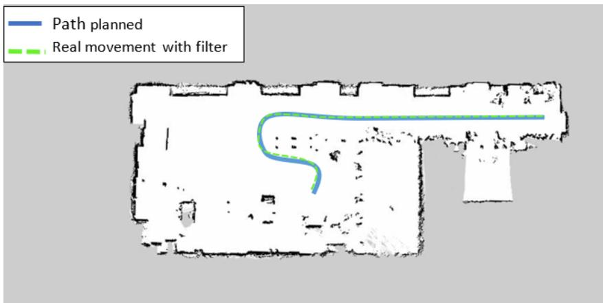
**Figure 6.21:** Map of CIM 4.0 and better path made by the robot. The blue line indicates the planned path instead the green dotted line indicates the path followed by the robot. With the use of sensor fusion to obtain odometry, a better result is obtained.
