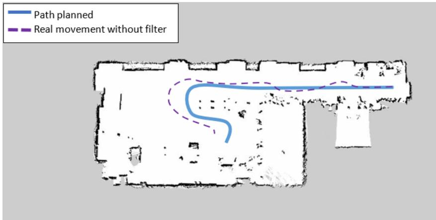
**Figure 6.20:** Map of CIM 4.0 and wrong path made by the robot. The blue line indicates the planned path instead the purple dotted line indicates the path followed by the robot. With the use of only one sensor to obtain odometry, there is an accumulation of errors.
