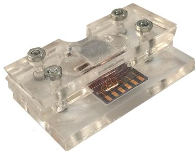
**Figure 3.6:** EGO-FET and microfluidic platform complete structure
