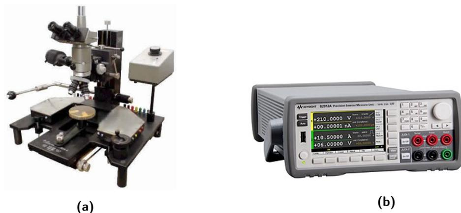
**Figure 3.8:** (a) Probe station (b) Keysight B2912A source/meter unit
