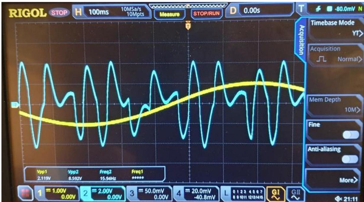
Figure 23 - 16Hz multiplier's stage output, yellow-1Hz, cyan-16Hz output of 4<sup>th</sup> stage multiplier
