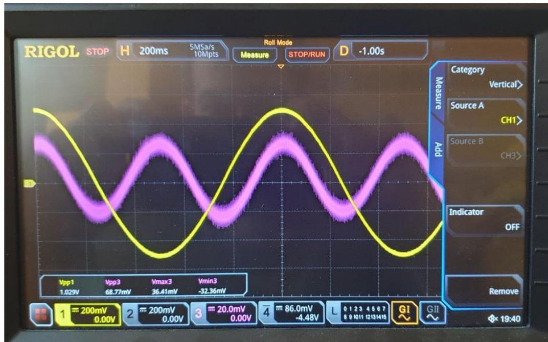
Figure 13 -The multiplication by 2 without DC compensation circuit
