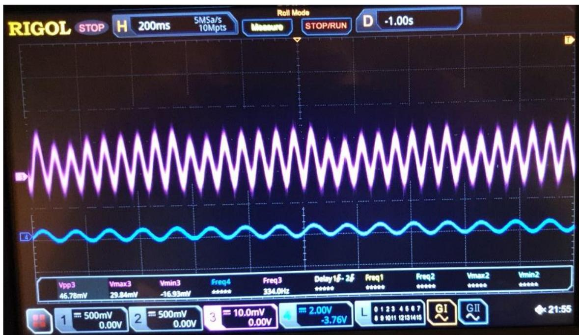
Figure 20 - 16Hz output of ad633 based multiplier
