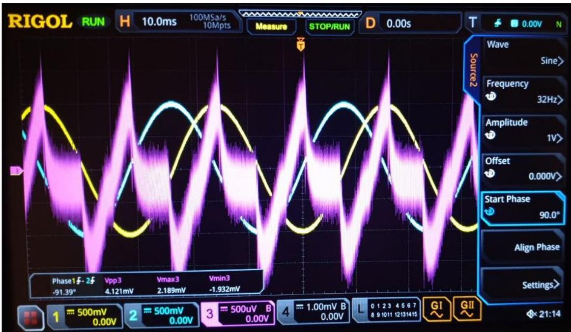
Figure 41 - AD834 phase detector output-pink, yellow-X input, Blue-Y input 90 degrees shifter
