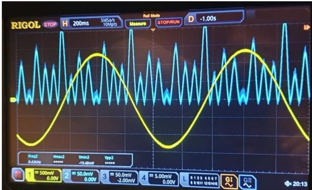
Figure 15- Multiplication by 16 with the DC compensator circuit
