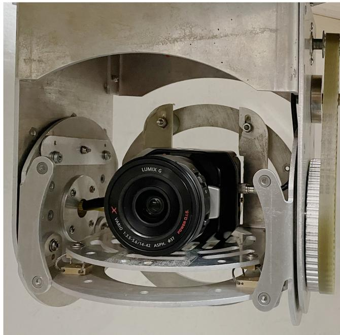
**Figure 7.2:** Camera mounted on the gimbal structure
