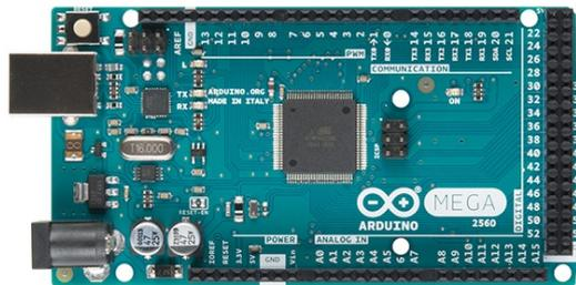
Figure 8.1: Arduino Mega 2560
