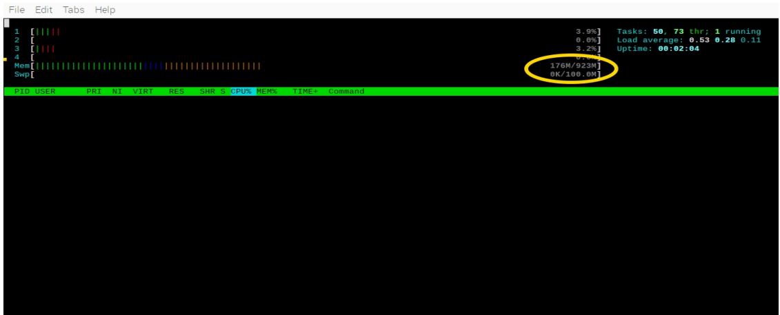
Figure 5.9. Raspberry Pi 3 Model B memory usage without launching the middleware.
