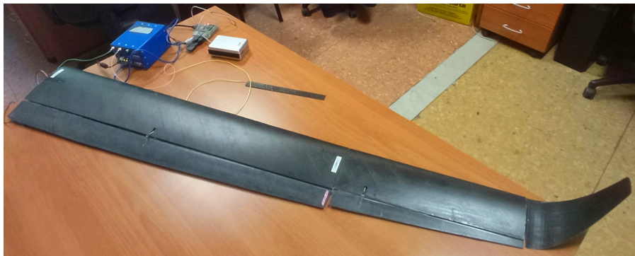
Figure 2.4. FBG sensor embedded inside an ICARUS aircraft wing.
