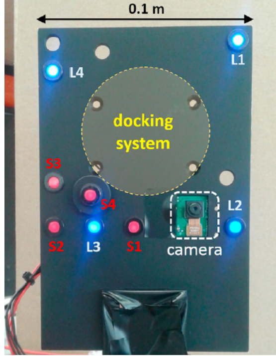
Figure 1.5: LEDs and camera setup on a 2U CubeSat panel [12]
