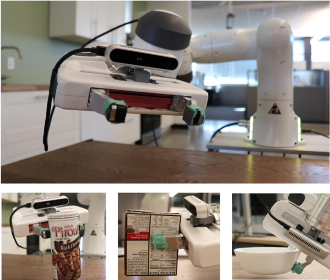
Figure 3.1. Robotic arm equipped with a 2-finger parallel-jaw gripper. The grasp task is usually intended as lifting and holding the object in a stable pose. Fig. source: [9].
