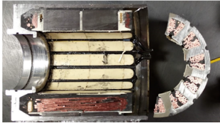
Figure 1.26: IPM motor internal section
