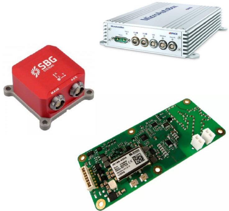
Figure 2.4: Some of the commercial boards in the vehicle. IMU in red, VCU in white and IMD in green
