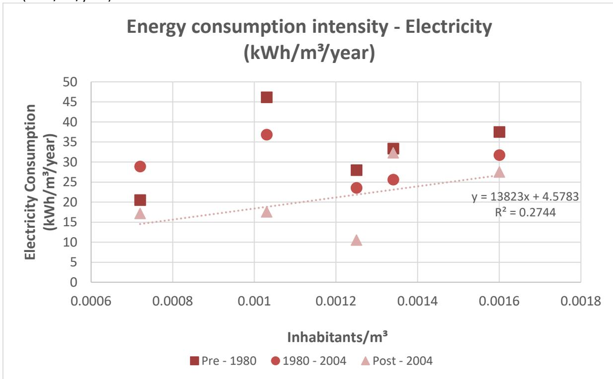
Figure 5.2.2.1, Linear regressions for energy consumption index on Electricity (kWh/m<sup>3</sup>/year) per unit of gross volume and Inhabitants
