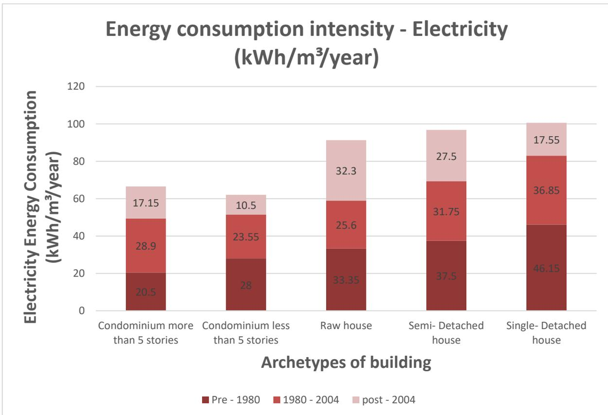
Figure 5.2.2.2, Total energy consumption for the Electricity (kWh/m<sup>3</sup>/year) considering the consumption of different archetypes of the residential buildings according to the inhabitants/m<sup>3</sup>.
