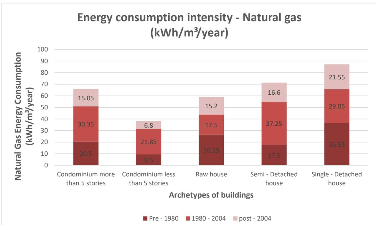
Figure 5.2.1 2, Total energy consumption for the Natural gas (kWh/m<sup>3</sup>/year) considering the consumption of different archetypes of the residential buildings during different periods of construction.
