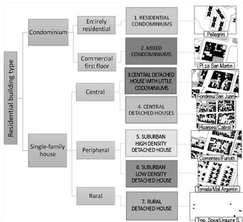
From this point, we started to define the typical model of the apartment building in different neighborhoods of the city, then the different areas were listed and analyzed along with the main characteristics that could affect the energy consumption so that each archetype has different energy consumption if the construction period different.
