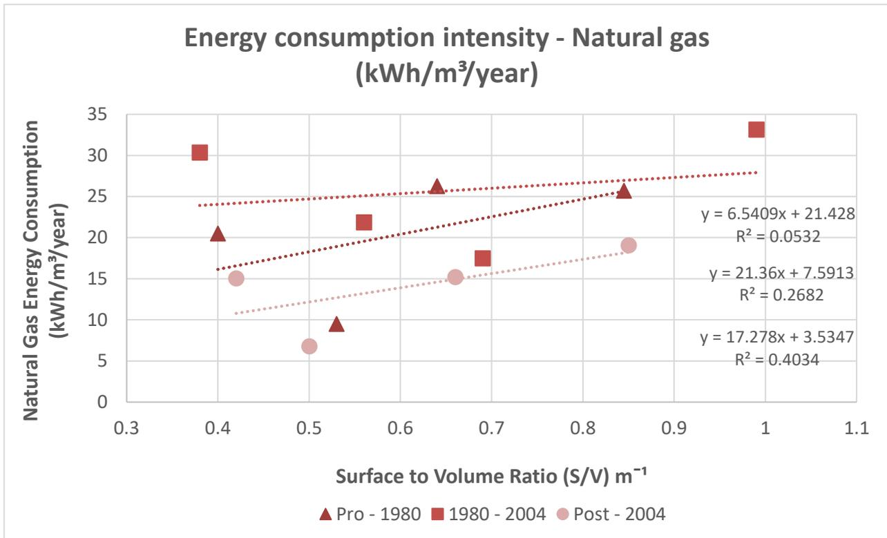
Figure 5.2.1 1, Linear regressions for energy consumption index on Natural gas per unit of gross volume and period of construction, (kWh/m<sup>3</sup>/year)
