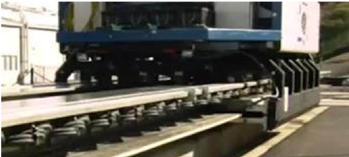
Figura 2.12: Full-scale Inductrack Demonstration, Fonte: National geographic
