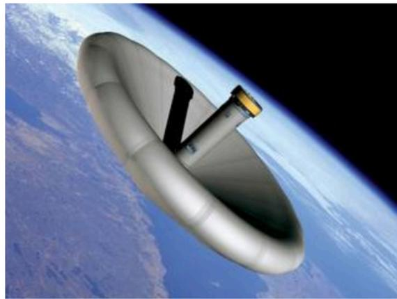
**Figura 2-17** Inflatable Aerodynamics Decelerator
