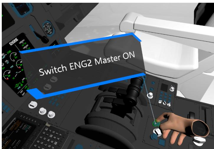
**Figura 4.11:** Step 6: Engine Master switch
