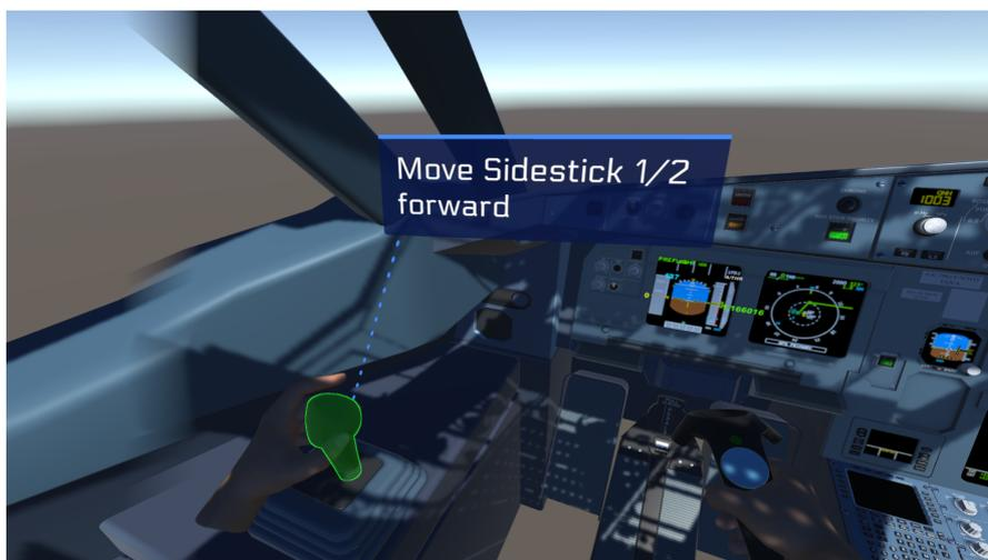
**Figura 5.11:** Step 1: Sidestick 1/2 forward
