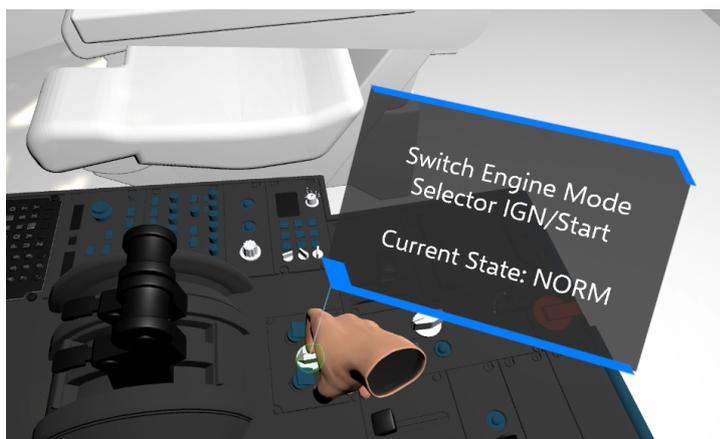
**Figura 4.6:** Step 1: Engine mode selector
