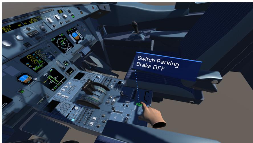
**Figura 5.12:** Step 2: Parking Brake OFF
