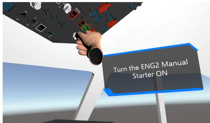
**Figura 4.10:** Step 5: Engine Manual Starter
