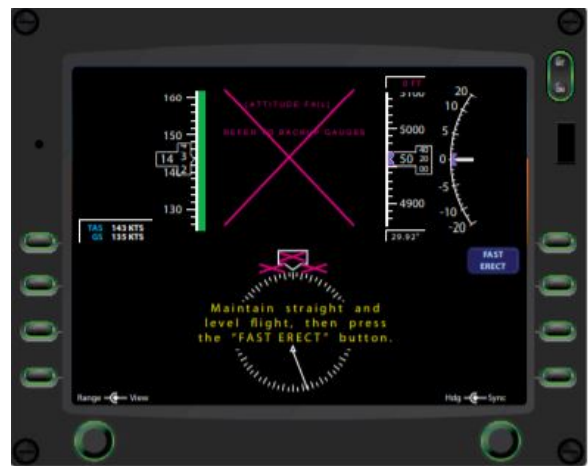
(b) A PFD indicating a failed AHRS
