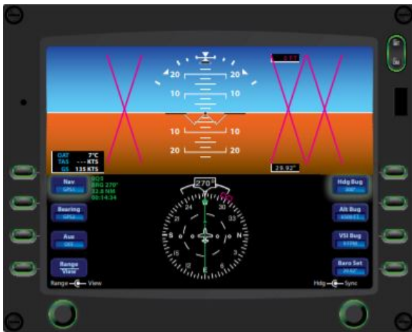
(a) A PFD indicating a failed air data computer
