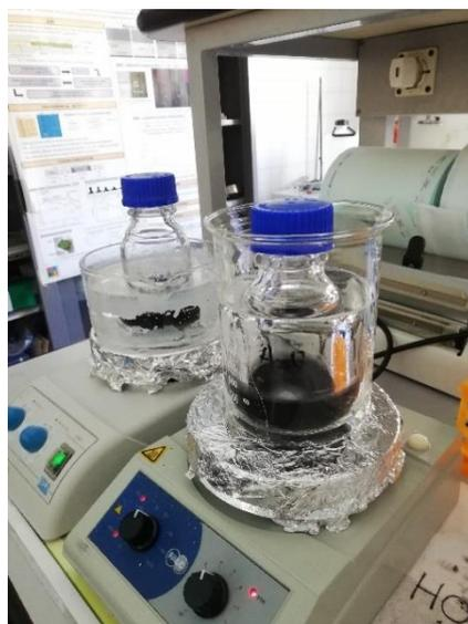
Fig.24 – EDTA chelation treatment ongoing on two samples.
