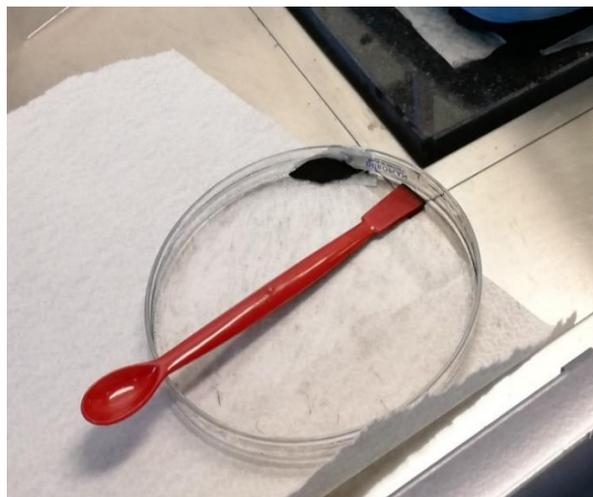
*Fig.17 – Cathode powders recover after scratching and drying.*
