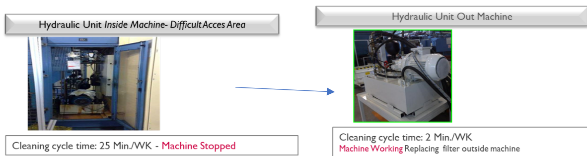
Figure 20: Difficult access area removal (Adapted from FPT Industrial S.p.A., 2021)
