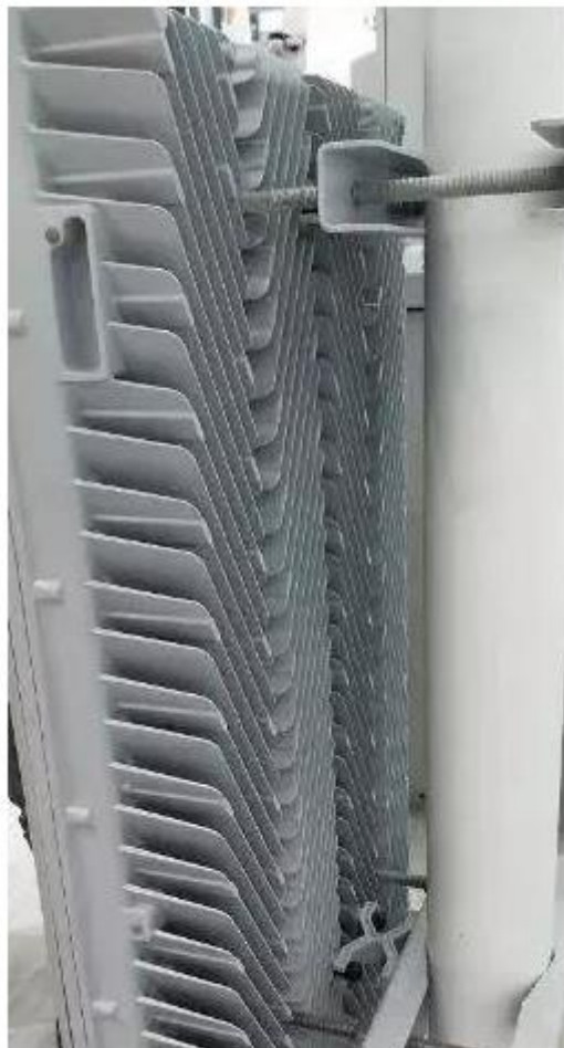
Figure 22: V-tooth structure design of the heat sink structure developed by ZTE Corporation [33].
